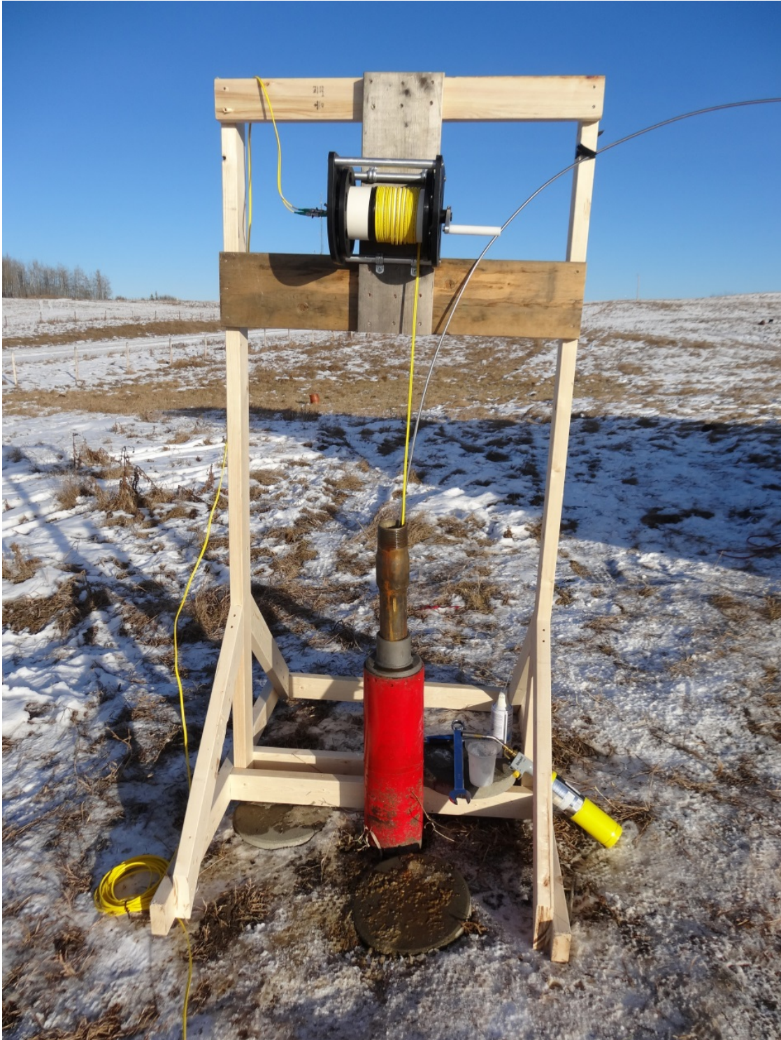
FIG 12. The gantry and winch for deploying the sensor in the well.
