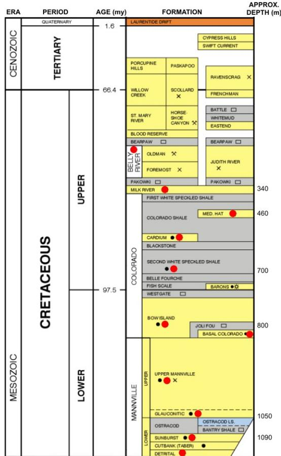
FIG. 2: Stratigraphic chart showing producing formations (after ERCB). Red dots indicate gas-producing formations. Our primary injection target is the Basal Belly River sandstone with possible secondary targets in the Medicine Hat and Second White Speckled Shale formations.
