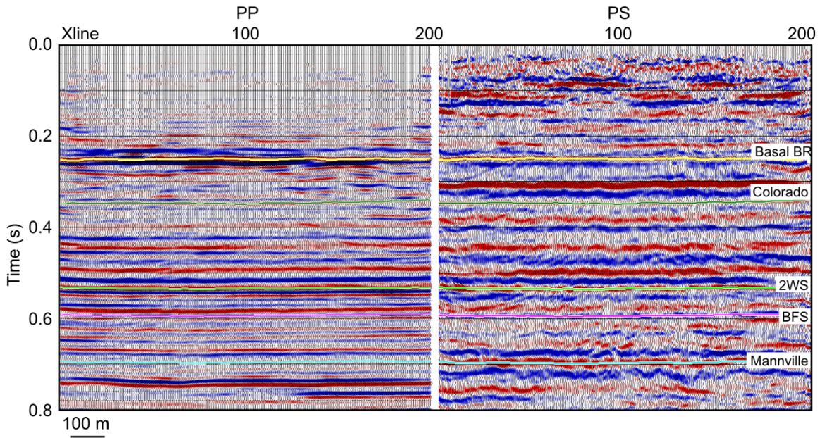
FIG. 11: Registered PP and PS data displayed together in PP time. The registration is based upon correlation of the annotated horizons.
