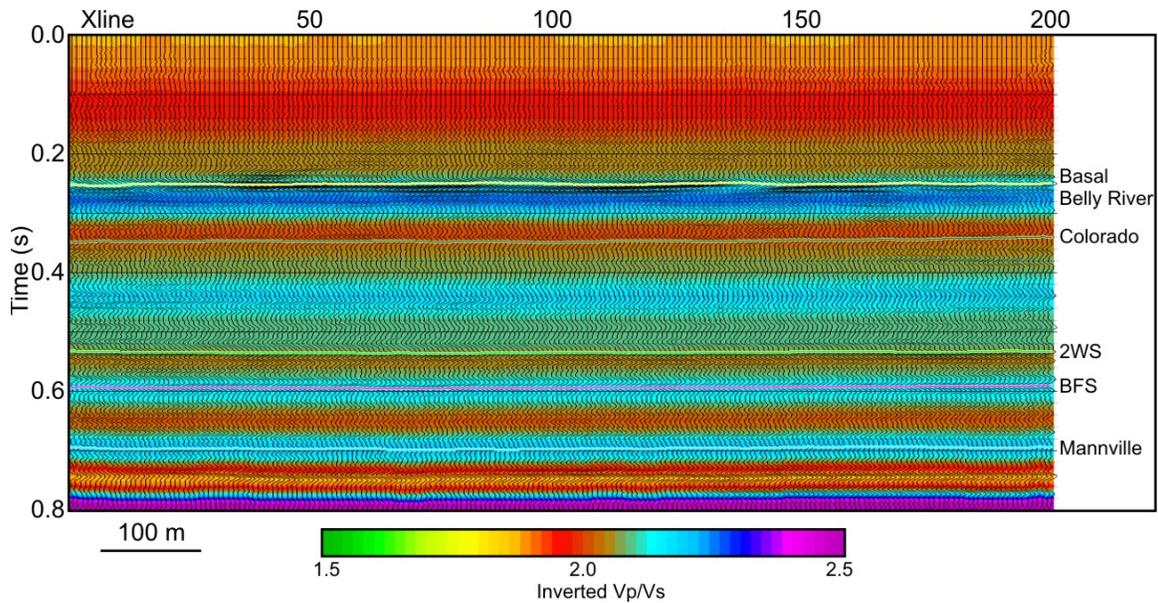
FIG. 13: Inverted Vp/Vs for inline 101.
