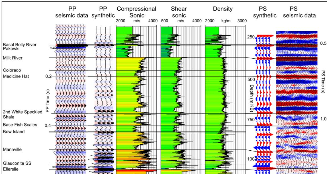
FIG. 8: Tie between PP data, well 07-22-017-016W4, and PS data.
