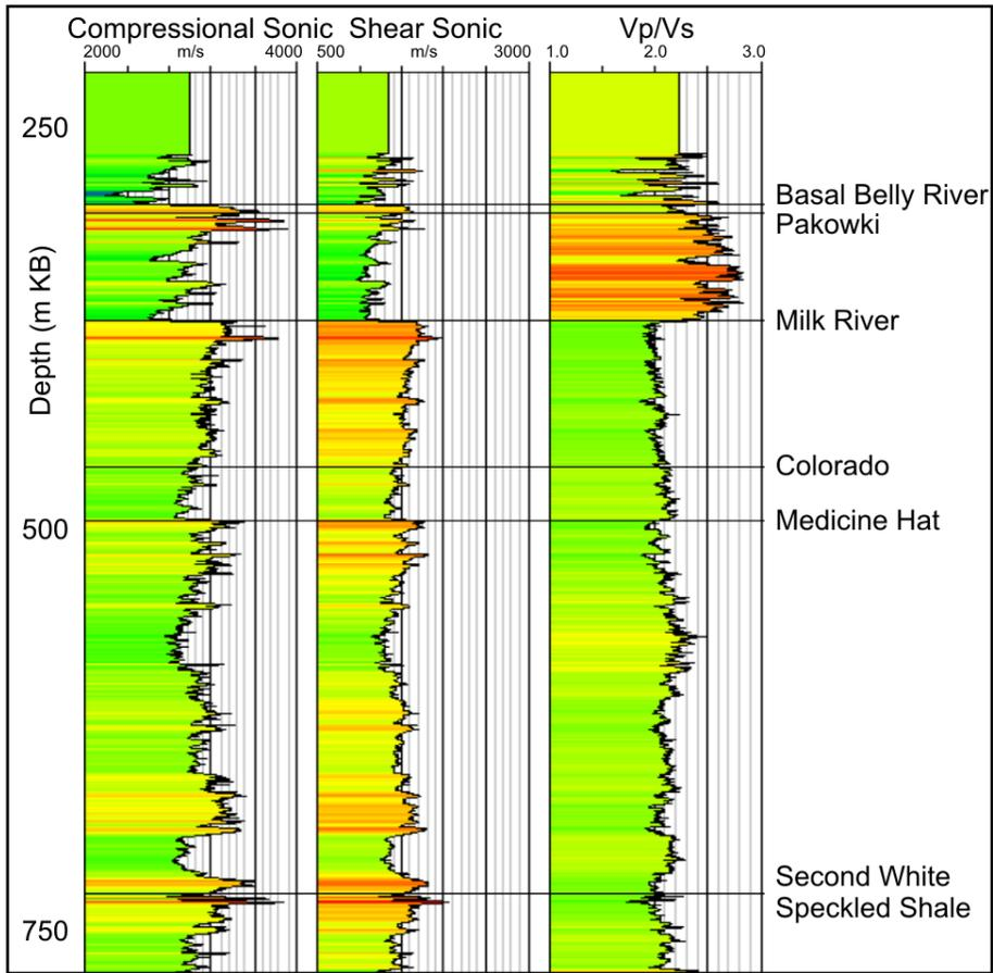
FIG. 6: Compressional and shear sonic logs from well 01-07-018-015W4 over the zone of interest and Vp/Vs calculated from them.
