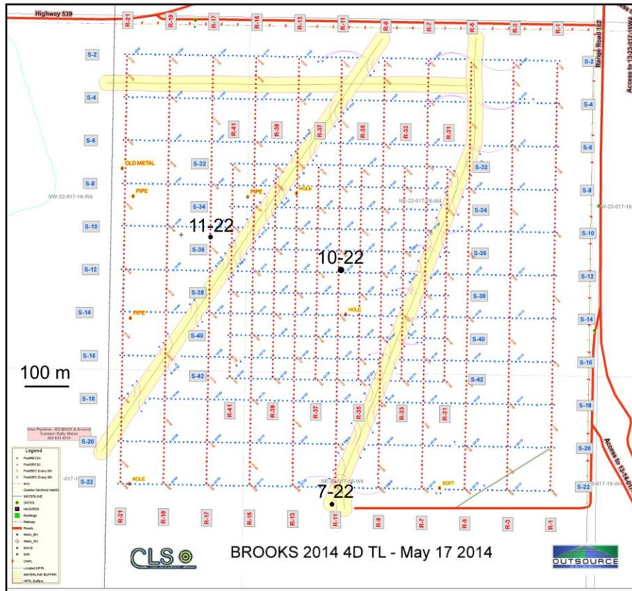
FIG 4: The layout of the 3D survey processed and interpreted for this study. The three wells shown in Figure 3 are annotated. 10-22 is the new well drilled in 2015.
