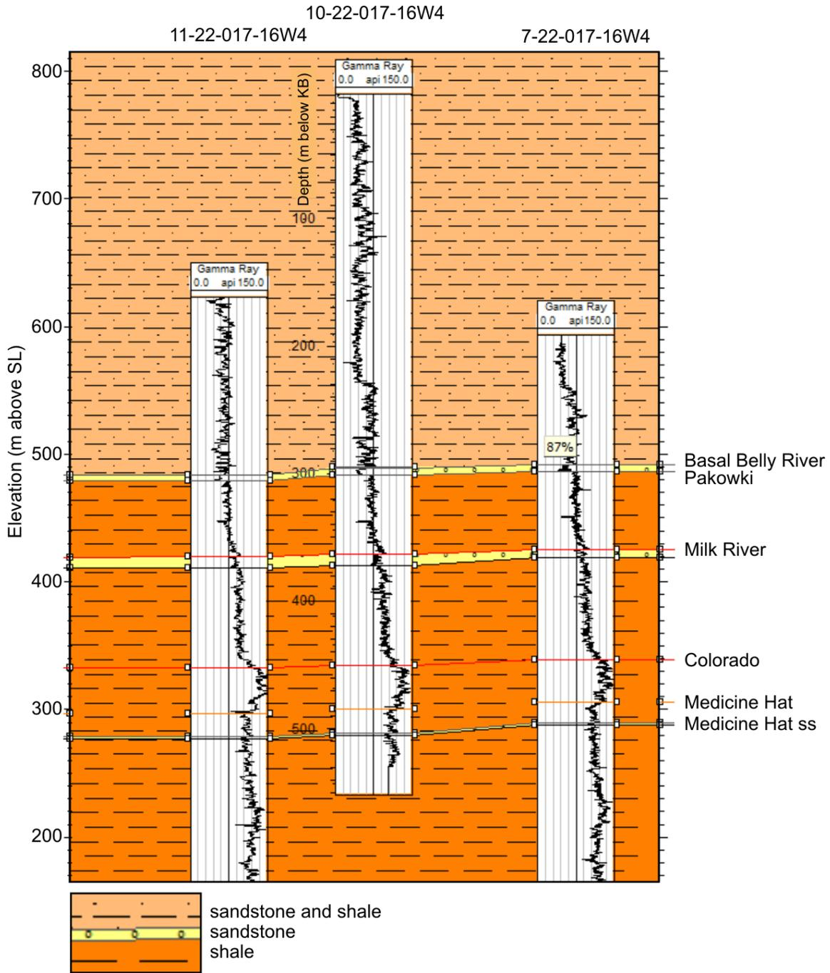
FIG. 3: Correlation of gamma ray logs across Section 22. The locations of the wells are shown in Figures 1 and 4. The primary sandstone of interest is the Basal Belly River.
