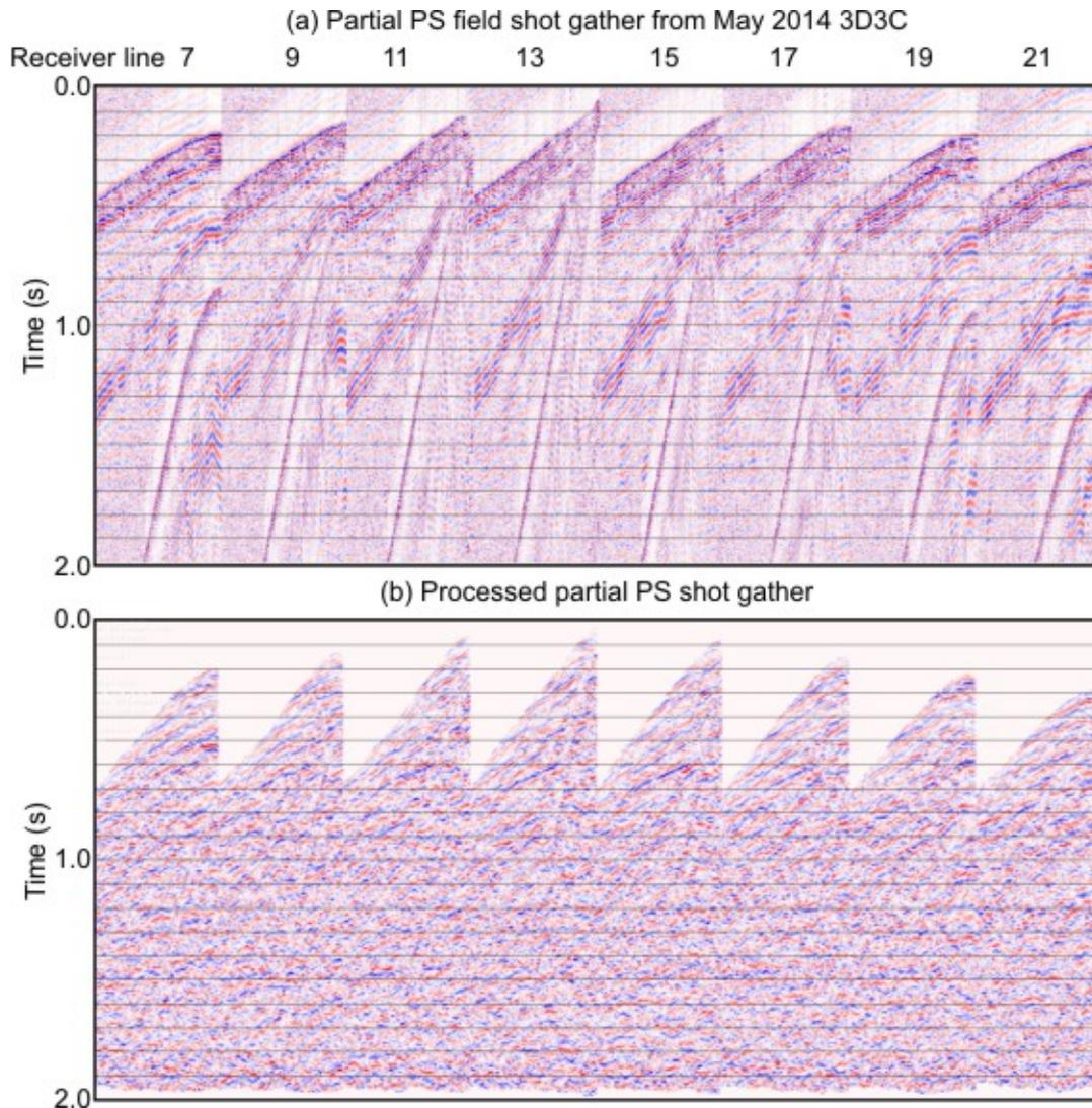
FIG. 5: Part of a PS shot gather before (a) and after (b) noise attenuation, statics and deconvolution.
