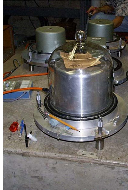
A state-of-the-art three-component broadband seismometer (Streckeisen STS-1) under vacuum cover.
