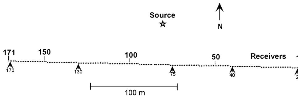
Figure 4.2. Field layout of the Blackfoot III 3C-2D test data. The source is 48 m offset from the line of receivers. Numbers on the line identify receivers and the receivers selected for testing are indicated with arrows.
