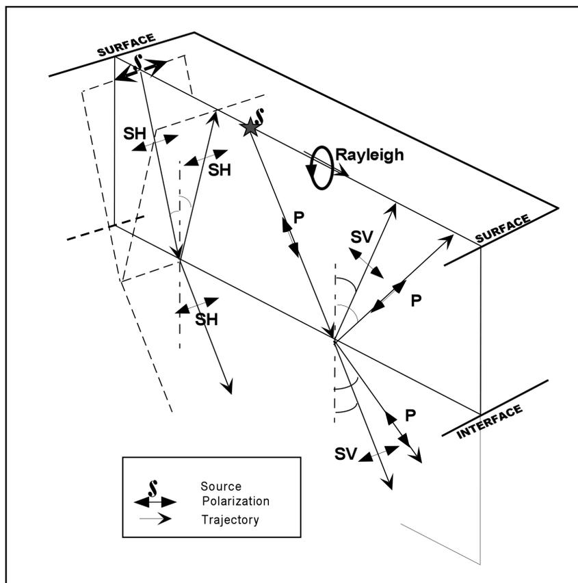
Figure 1.1. Schematic diagram of the two multicomponent seismic methods on land. On the left, pure  $S$  waves ( $SH$ ) and on the right, a converted  $S$  wave ( $SV$ ). The energy source is different in each case (an  $SH$  source in the first case and a standard  $P$  wave source in the second). The path of the trajectory is symmetrical for  $SH$  waves and asymmetrical for converted waves. (Modified after Tatham and McCormack, 1991).
