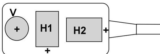
Figure 1.2. Top view of the elements of a Cartesian 3-C geophone.  $V$  indicates the vertical element, and  $H1$  and  $H2$  the two horizontal elements. The polarity is marked by the *plus* sign, which indicates the tap location that causes a positive value in the geophone's voltage output.
