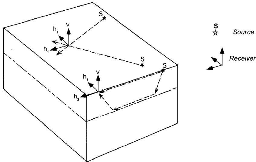
Figure 4.1. Relation between polarization and source-receiver direction in multicomponent 2-D and 3-D surveys. Receivers usually are oriented in the in-line direction. Source-receiver direction is on the line in 2-D and can have any direction in 3-D.
