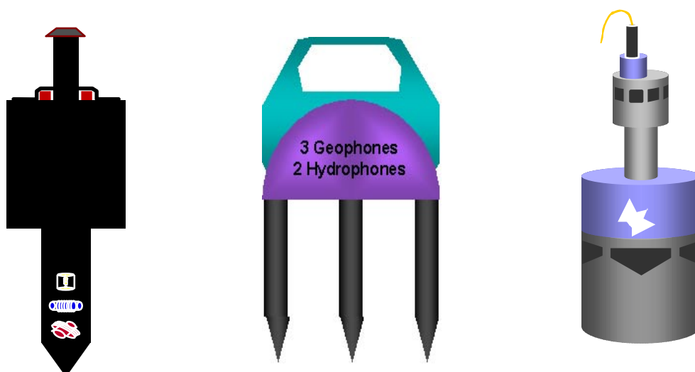
Figure 2.3.3 - Examples of single nodes 4-C receivers (after Entralgo and Wadsworth, 1999 ). Mechanical arms of remote operated vehicles (ROV) plant the sensors.
