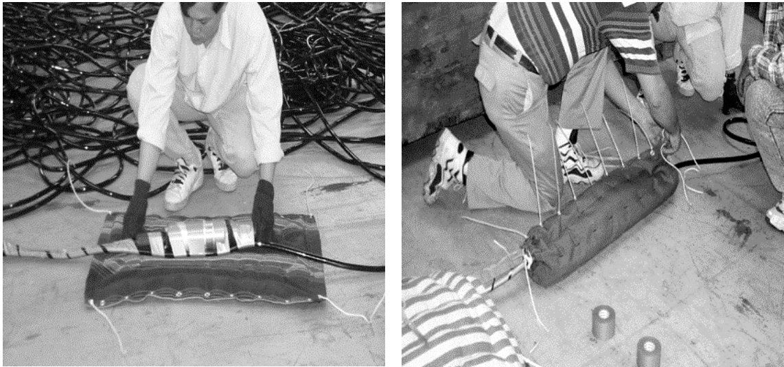
Figure 5.2.3 – 4-C receiver unit of Figure 5.2.2 being sandbagged ( after www.erch.com ). This method is licensed by Atlantic Richfield Co (Sullivan, 1995).
