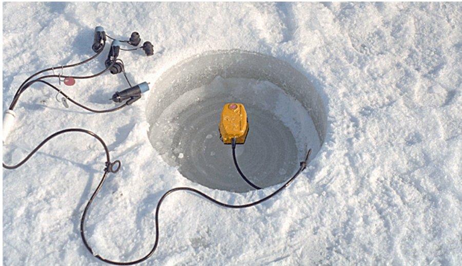
Figure 4.8 Typical 3-C geophone plant in an augured hole in the sea ice. Geophones were frozen in with fresh water.
