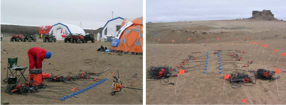
Figure 2.6 High resolution 3C-2D and 3C-3D seismic surveys, left and right panels respectively. The geophones in the 2D survey are oriented in the N-S direction, while in the 3D the receiver lines are oriented in the E-W direction.
