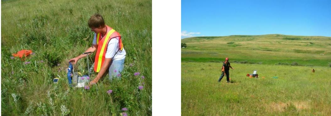
Figure 3.3. Vibration monitor setup (left) and shooter ready to fire a source point (right) (Photos by Dr. Robert Stewart).
