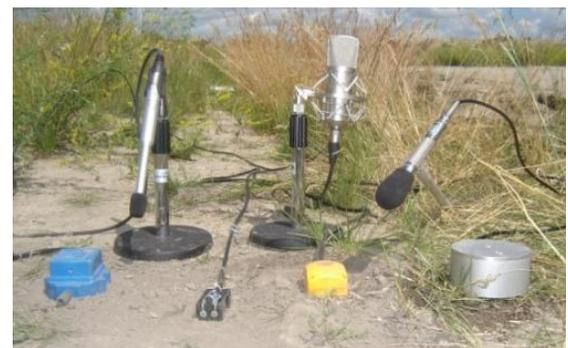
Figure 4.6. Southwest view of the seismic line with the mini Vibe located at shot point one (left) and the seven-sensor test pad located at the northeast end (bottom right). The observer's computer was located about 3.5m north of the test station while the Blastmate monitor was located about 1 m east of the test station (top right) (Photos by Alejandro Alcudia).
