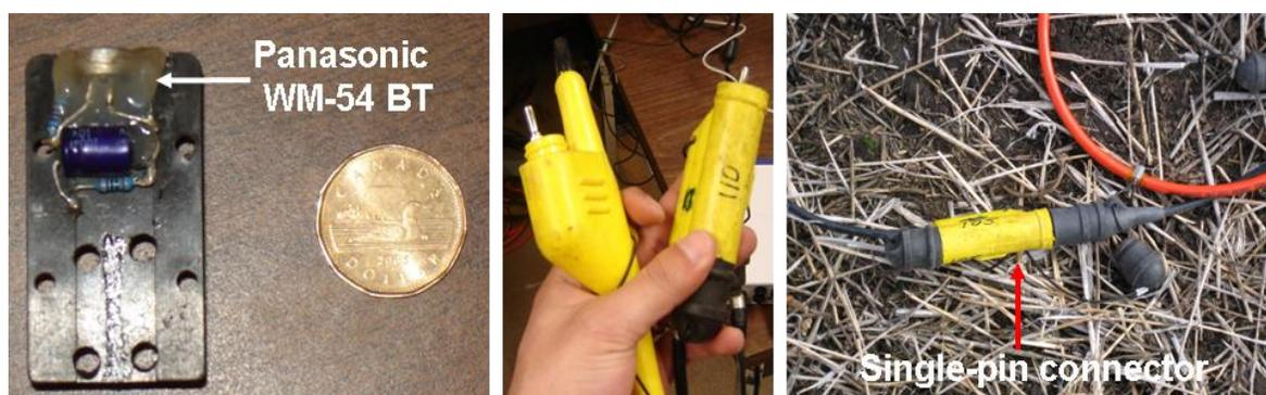
Figure 4.3. CREWES microphone prototype and single-pin connector used to transmit the microphone output to the recording system.
