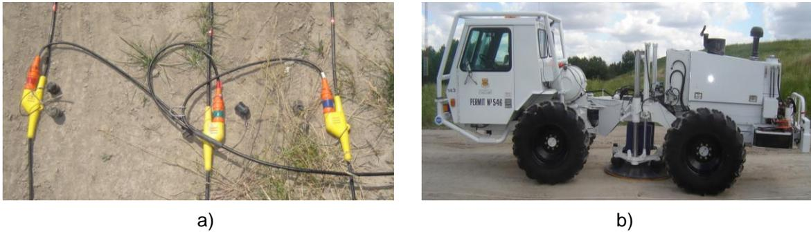
Figure 4.8. a) Geophone cable connections were facilitated by using color codes for each component. Each Geode recorded a full data set of a particular geophone component. b) The mini EnviroVibe, owned by the University of Calgary, was used as one of two seismic sources.
