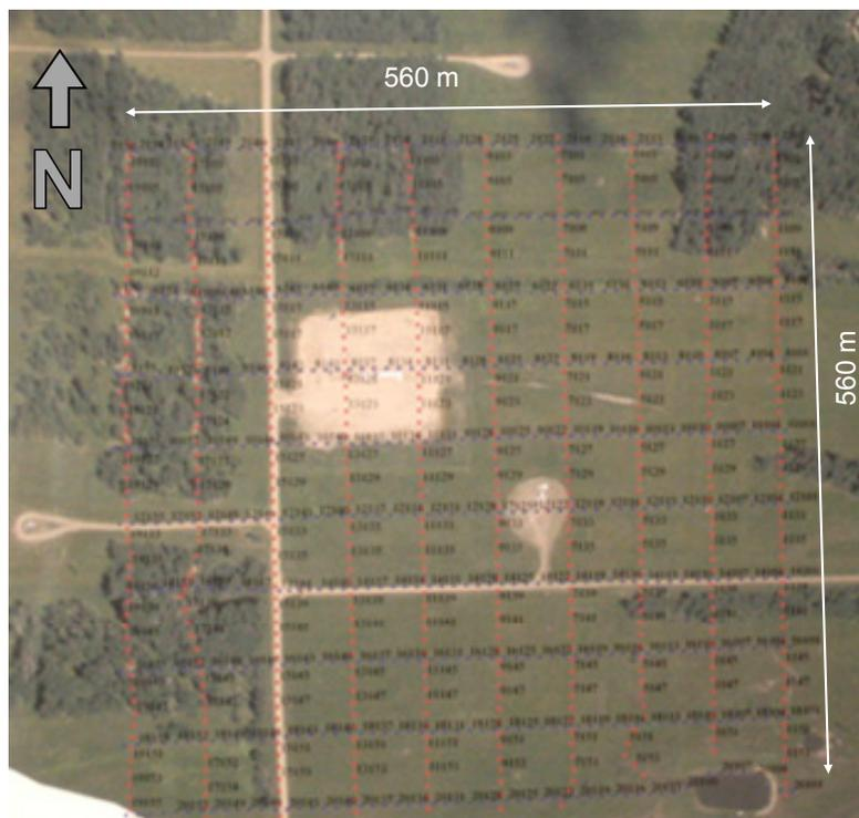
Figure 4-4: The survey layout in the field. Source lines run north-south and receiver lines run east-west.
