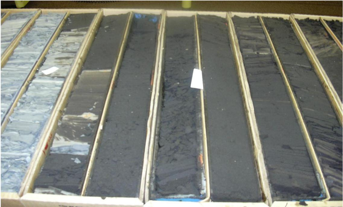
Figure 3.6 Cores of cap rock and reservoir rock (oil sands)
