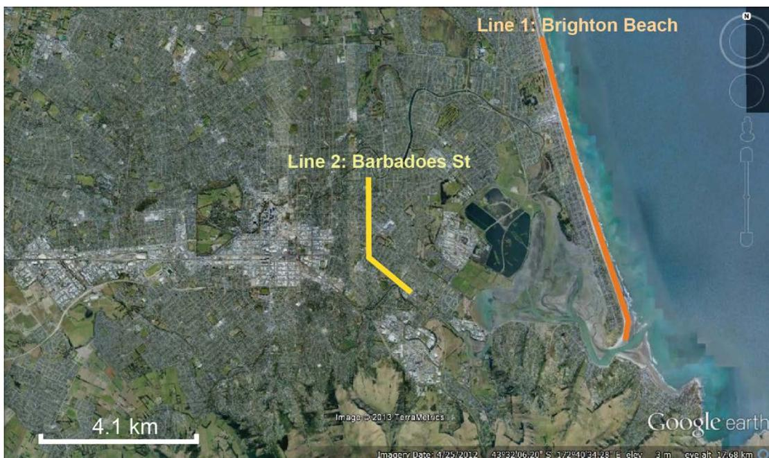
**Figure 2-6. Overview map showing seismic data acquisition in the city of Christchurch, New Zealand. Line 1 (orange) is along New Brighton Beach, and Line 2 (yellow) is along Barbadoes Street. Google earth V 7.0.3.8542. (25 April 2012) Christchurch, New Zealand. 43°32'06.48"S, 172°40'34.28"E, Eye alt 17.68 km. TerraMetrics 2013. <http://www.earth.google.com> [May 30, 2013].**
