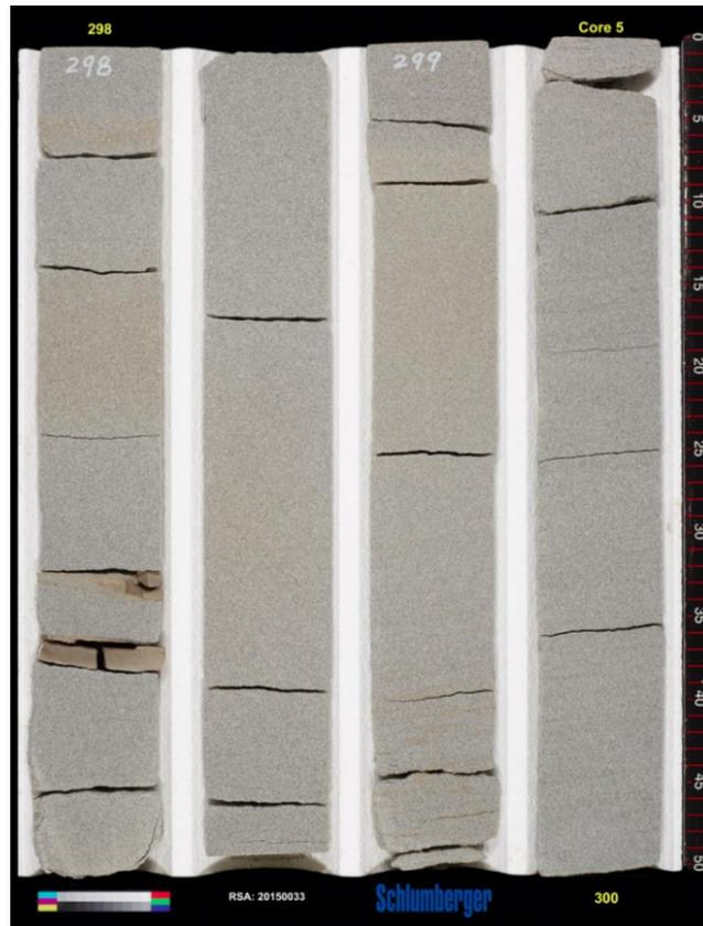
Figure 2-3. Photo of the slabbed core interval identifying the sandstone reservoir of the BBRs unit at a depth of 298 to 300 m.
