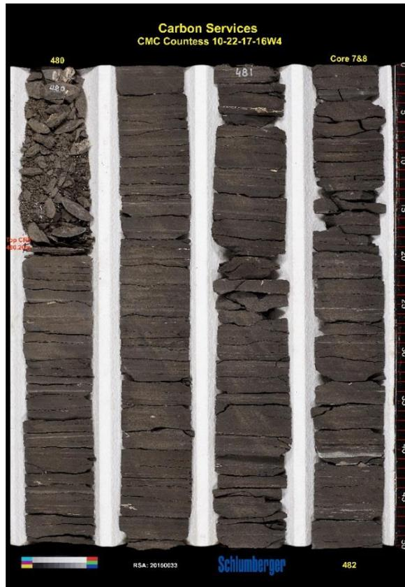
Figure 2-2. Photo of the slabbed core interval identifying the caprock seal interval of the 1WS Member at a depth of 480 to 482 m.
