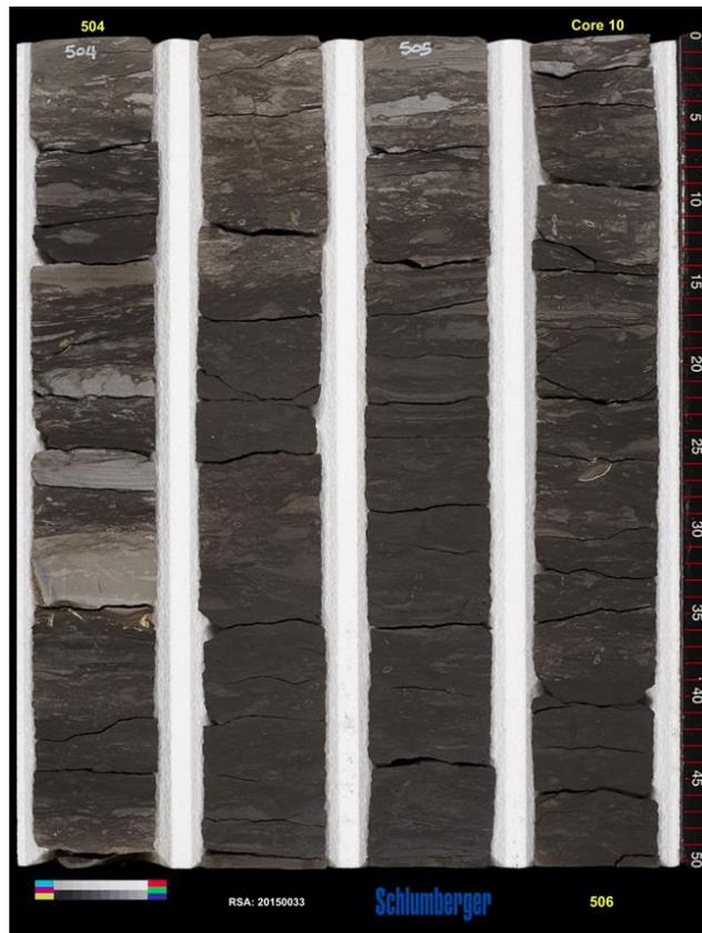
Figure 2-1. Photo of the slabbed core interval identifying the sandstone beds within the Medicine Hat Member interval at a depth of 504 to 506 m.
