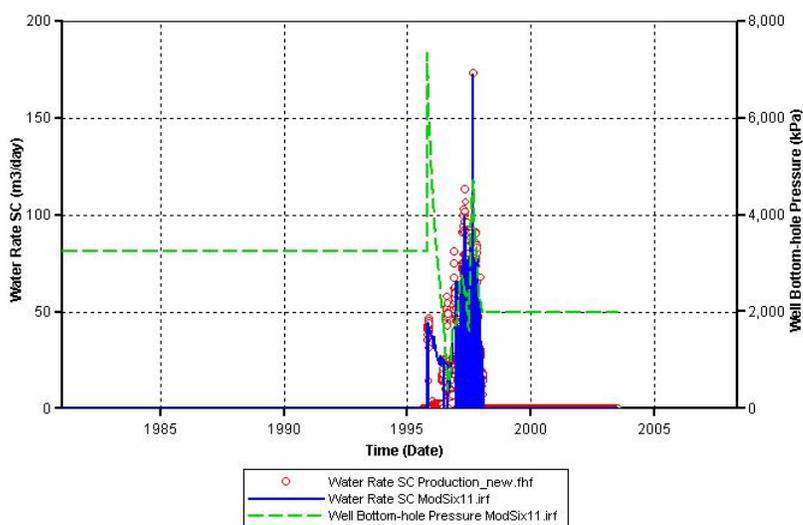
**Figure A.8 History matching results of water rate and bottom hole pressure for well 4A2-6. The red dots are the water rate in standard condition from the history file. The blue line is the water rate in standard condition from the simulation output. The green dash line is the well bottom-hole pressure from the simulation output (there is no pressure history file).**
