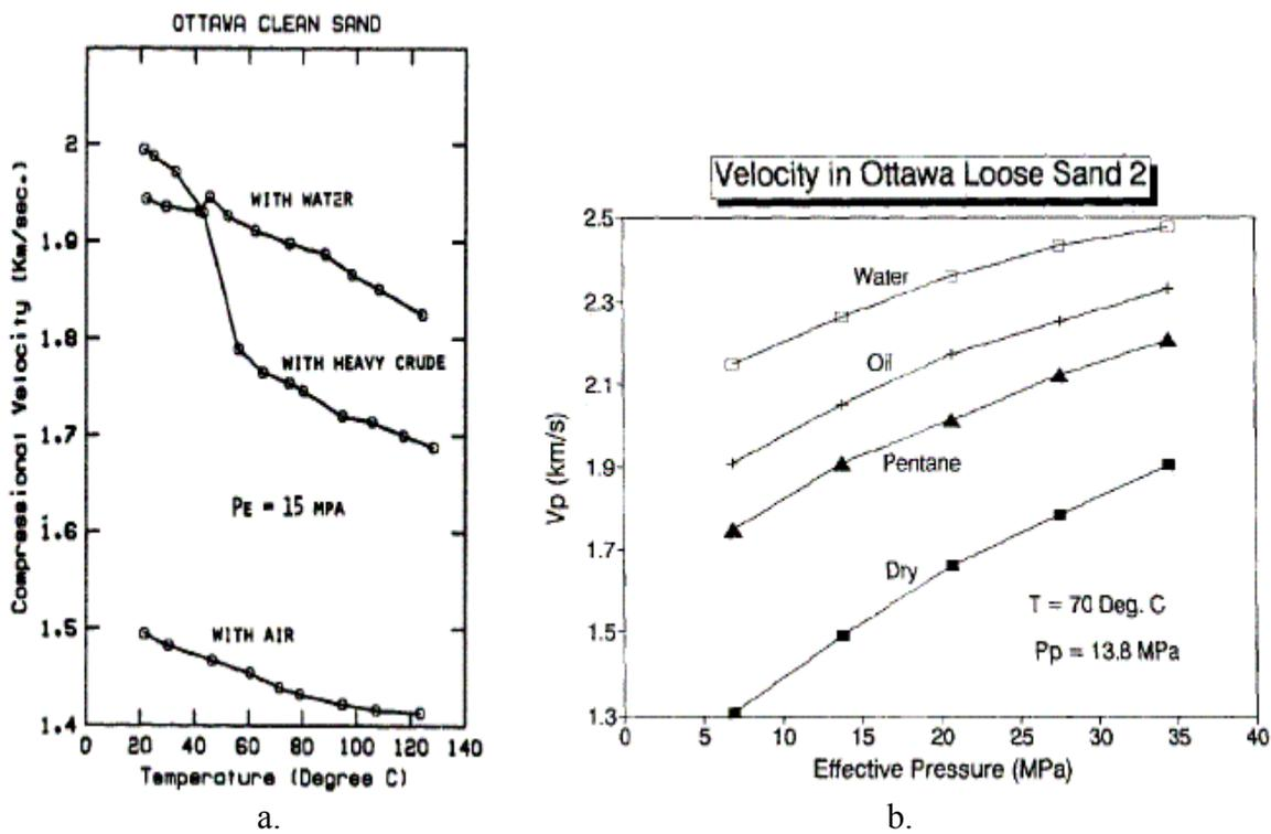
**Figure 2.3 Lab measured compressional and shear velocities for Ottawa unconsolidated sand. a.  $V_p$  vs.  $T$ , effective pressure  $P_e=15$  MPa, after Wang and Nur, 1986, b.  $V_p$  vs.  $P_e$ ,  $T=70^\circ\text{C}$ , after Wang et al, 1991.**
