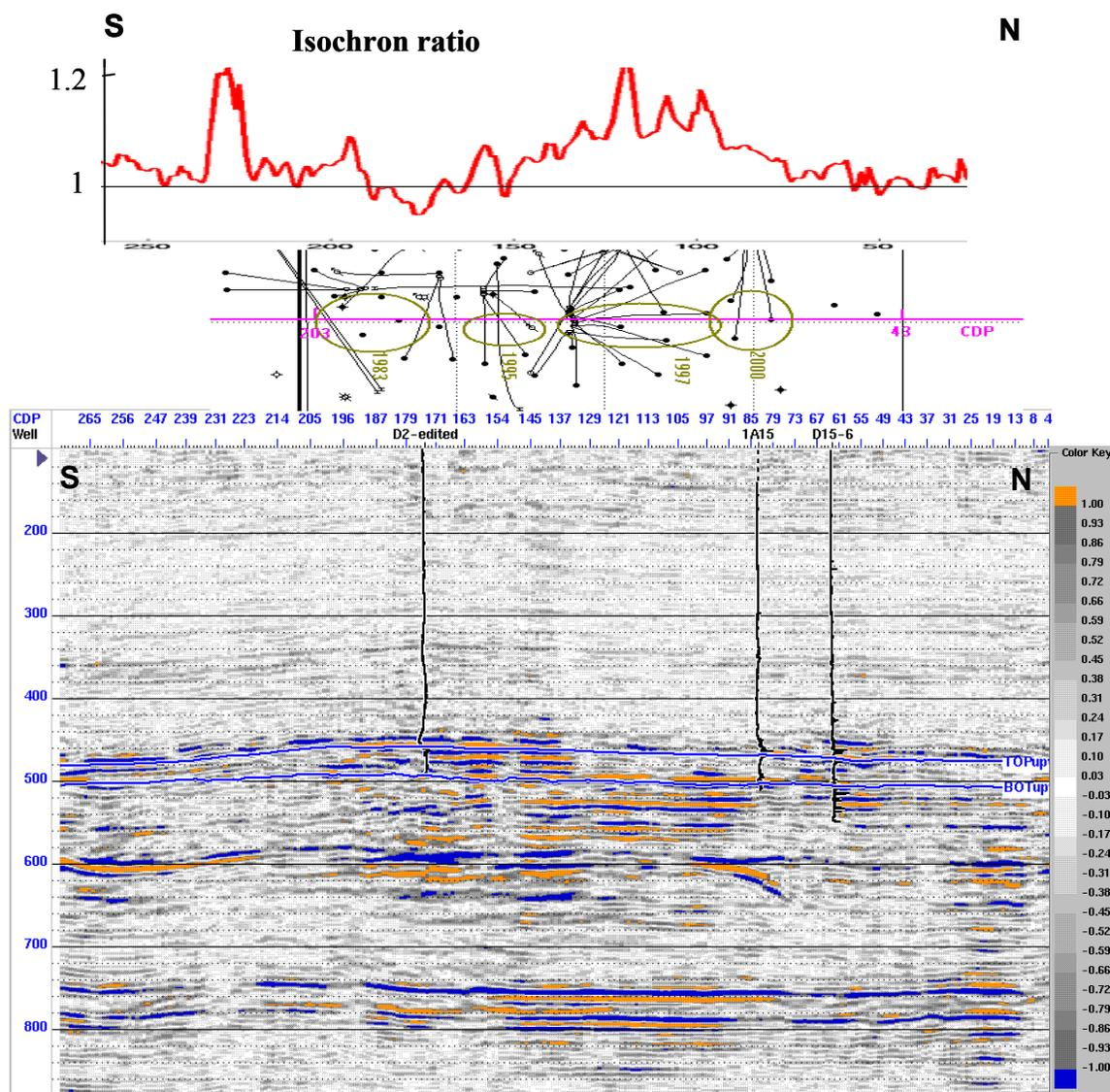
**Figure 3.9.** Difference from two mean window scaling (bottom, in relative scale from  $-1$  to  $1$ ) with well activities (middle, circles mark the drilling time) and isochron ratio (top, which is the isochron of the 2000 survey divided by the one from the 1991 survey).
