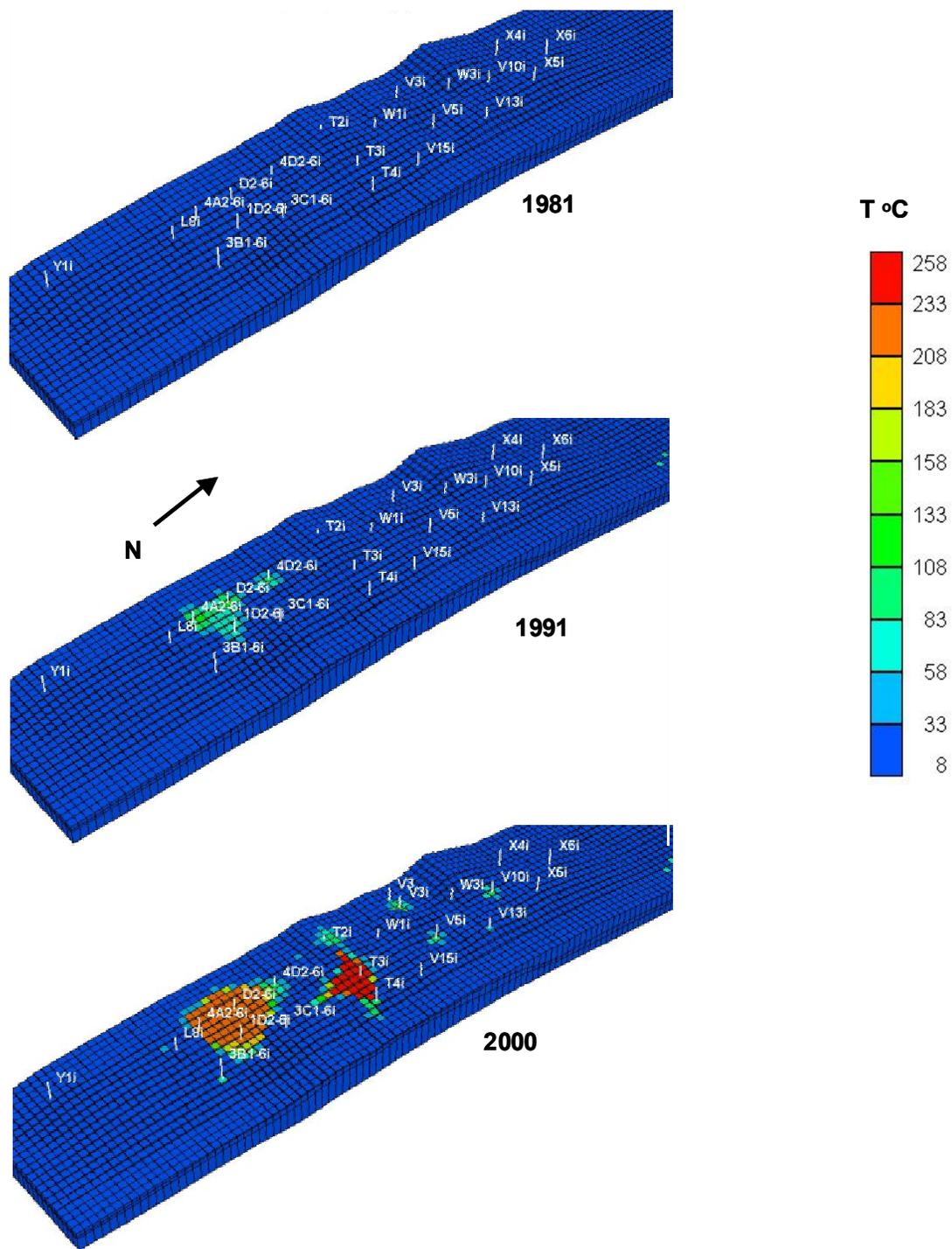
Figure 4.4 Temperature distributions from reservoir simulation at three dates.
