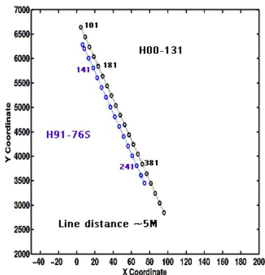
**Figure 3.1 Relative locations between line H00-131 and H91-76S (The scale is not the same in X and Y directions).**
