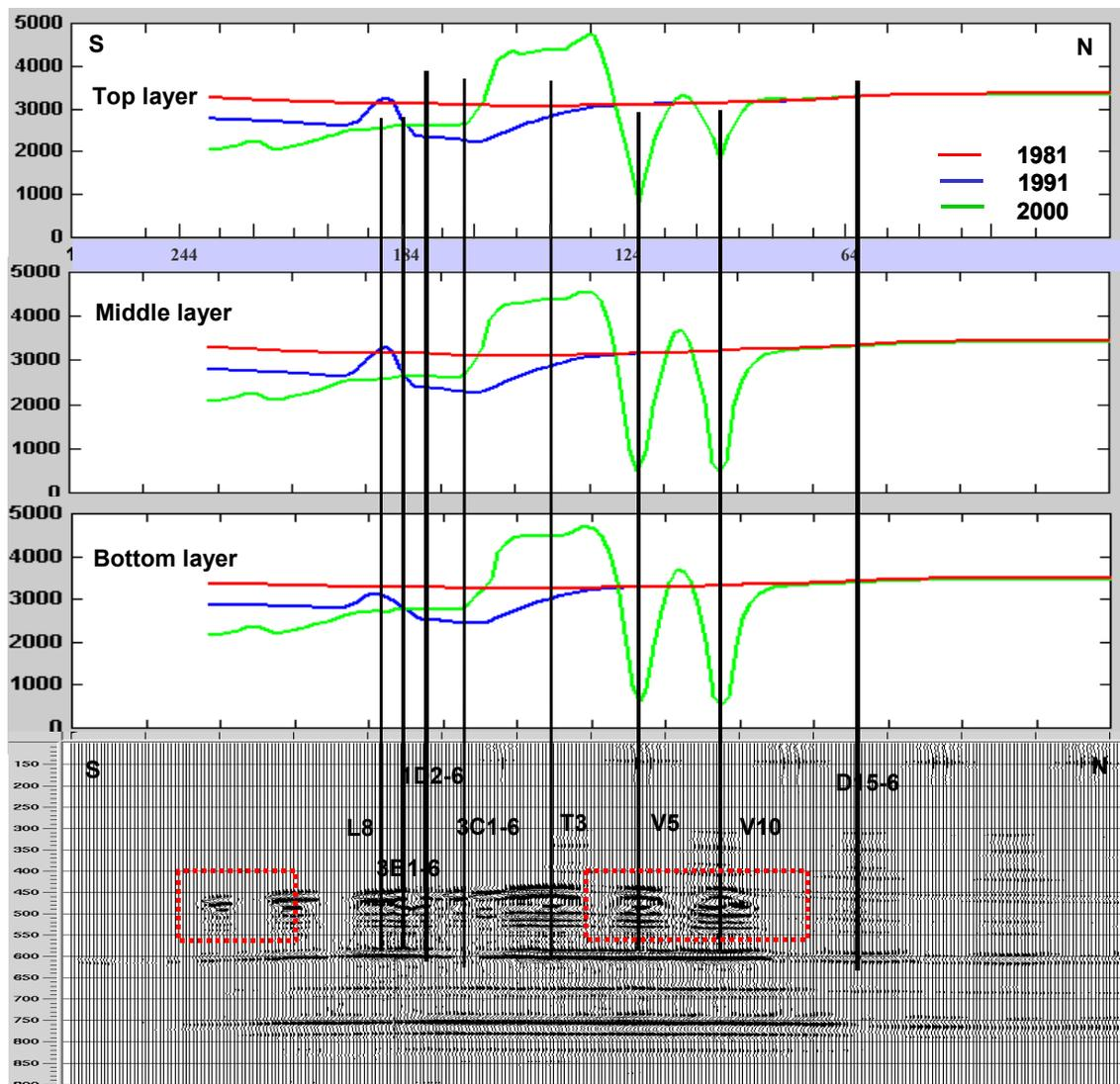
**Figure 6.4 Reservoir pressure distribution in the three layers (up) and the synthetic seismic difference section (down).**
