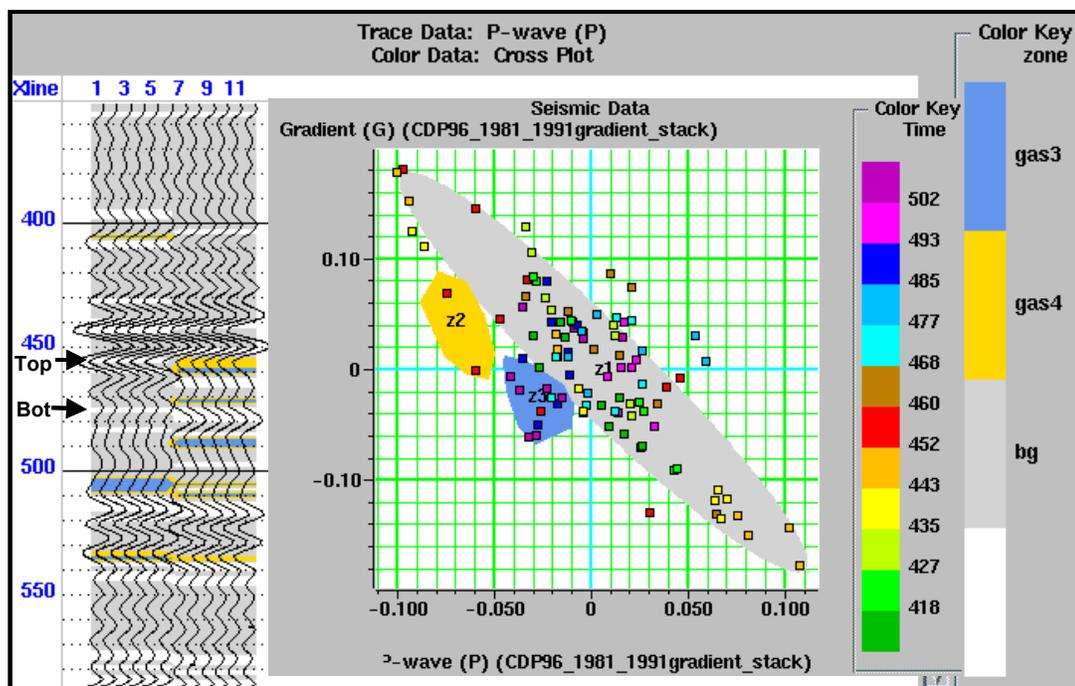
**Figure 6.9** AVO analysis of the synthetic logs. The left wiggle traces are intercept stacks. Traces 1 to 5 are repeated traces for pre-production and traces 6 to 10 are repeated traces for post-production. The colour key time is the time in ms. The colour key zone indicates class 3 gas (blue), class 4 gas (yellow), and back ground mud-rock line (grey).
