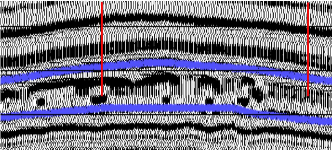
**Figure 5.8 Enlarged final migrated stack of the 2000 synthetic seismic section**
