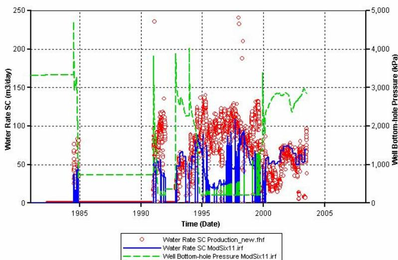
**Figure A.4 History matching results of water rate and bottom hole pressure for well 3B1-6. The red dots are the water rate in standard condition from the history file. The blue line is the water rate in standard condition from the simulation output. The green dash line is the well bottom-hole pressure from the simulation output (there is no pressure history file).**
