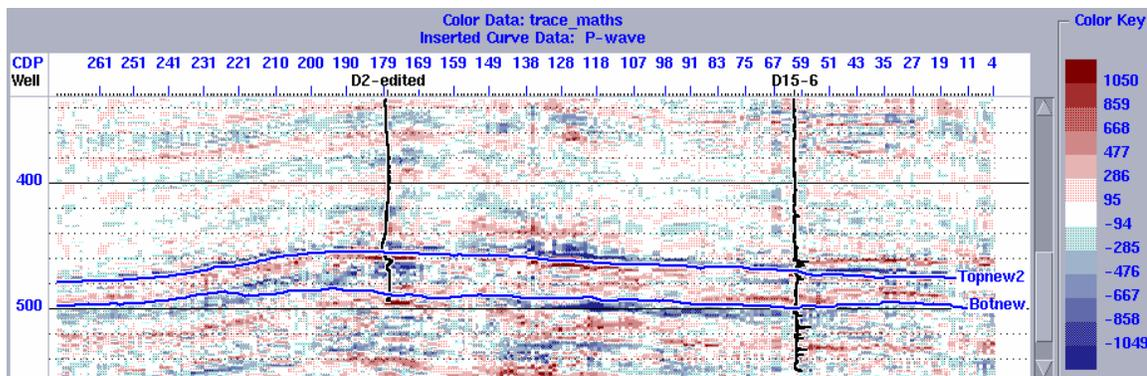
**Figure 6.18** The impedance difference (1991 impedance minus 2000 difference). The circled areas have largest values.
