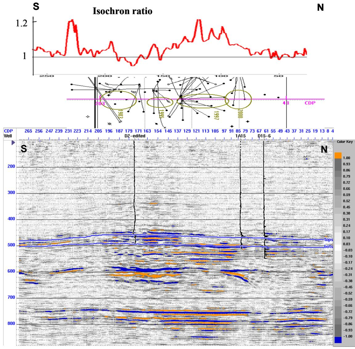
Figure 3.8. Difference from surface consistent scaling (bottom, in relative scale from -1 to 1) with well activities (middle, circles mark the drilling time) and isochron ratio (top, which is the isochron of the 2000 survey divided by the one from the 1991 survey).
