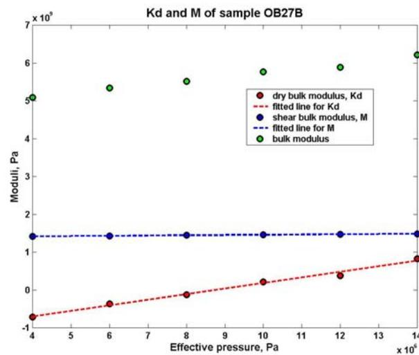
**Figure 2.7 Dry bulk modulus and shear modulus and the fitted lines for sample OB27B.**
