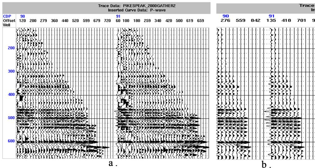
Figure 6.11 The original gathers of the 2000 survey with a bin size of 20 m. b. The common offset stacks generated by stacking every 5 CDPs and the offset bin size is 50 m.
