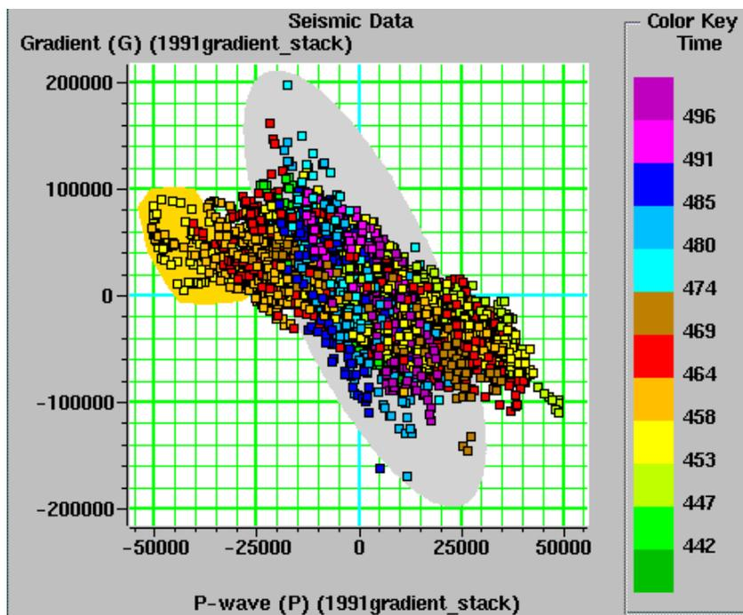
Figure 6.12 Cross plot of the 1991 seismic survey 100 ms around reservoir top.
