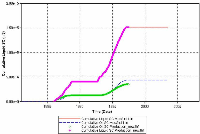
**Figure. A.1 History matching results of cumulative liquid and cumulative oil production for well L8 in standard condition. The pink dots are the cumulative liquid productions from the history file. The red line is the cumulative liquid production from the simulation output. The green dots are the cumulative oil production from the history file. The blue dash line is the cumulative oil production from the simulation output.**
