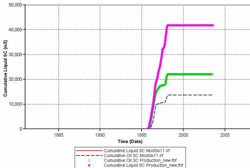
**Figure. A.7 History matching results of cumulative liquid and cumulative oil production for well T3 in standard condition. The pink dots are the cumulative liquid productions from the history file. The red line is the cumulative liquid production from the simulation output. The green dots are the cumulative oil production from the history file. The blue dash line is the cumulative oil production from the simulation output.**
