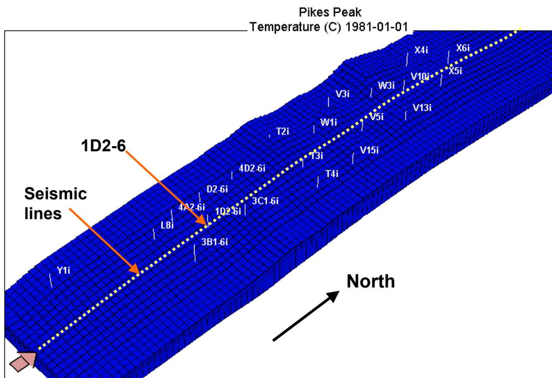
**Figure 4.1 Reservoir geometry, production wells, and time-lapse seismic line location.**
