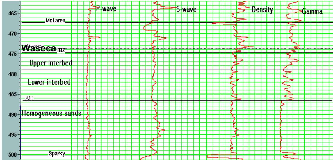
Figure 1.5 Logs from well 1A15-6 (median filtered). The partial logs from 465 to 500 m are shown here.
