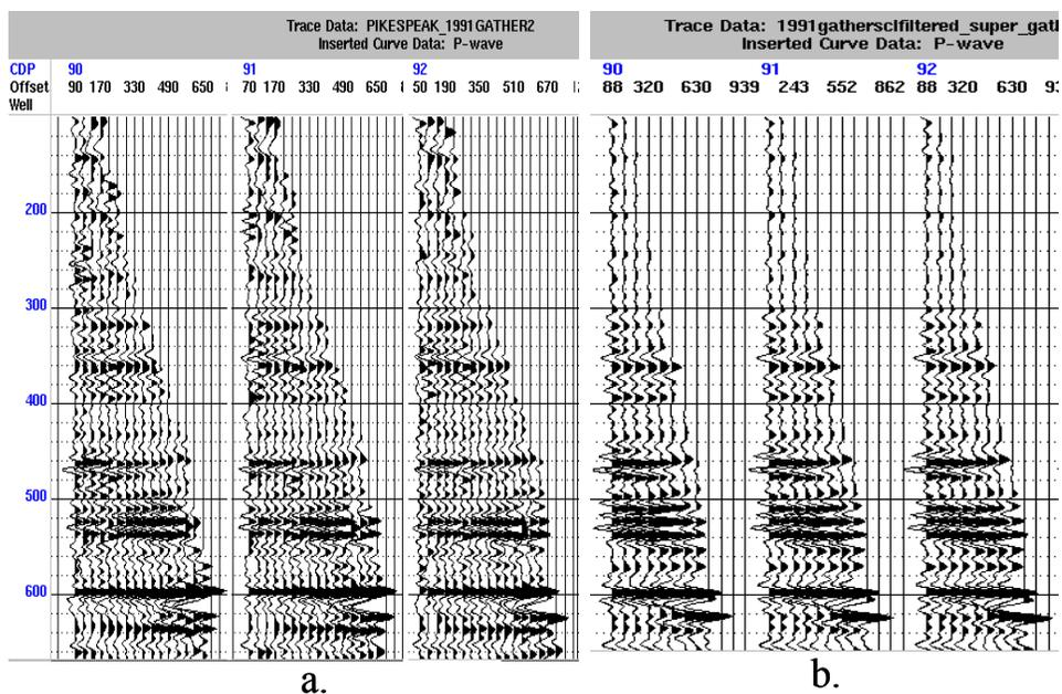
Figure 6.10 a. The original gathers of the 1991 survey with a bin size of 20 m. b. The common offset stacks generated by stacking every 5 CDPs and the offset bin size is 50 m.
