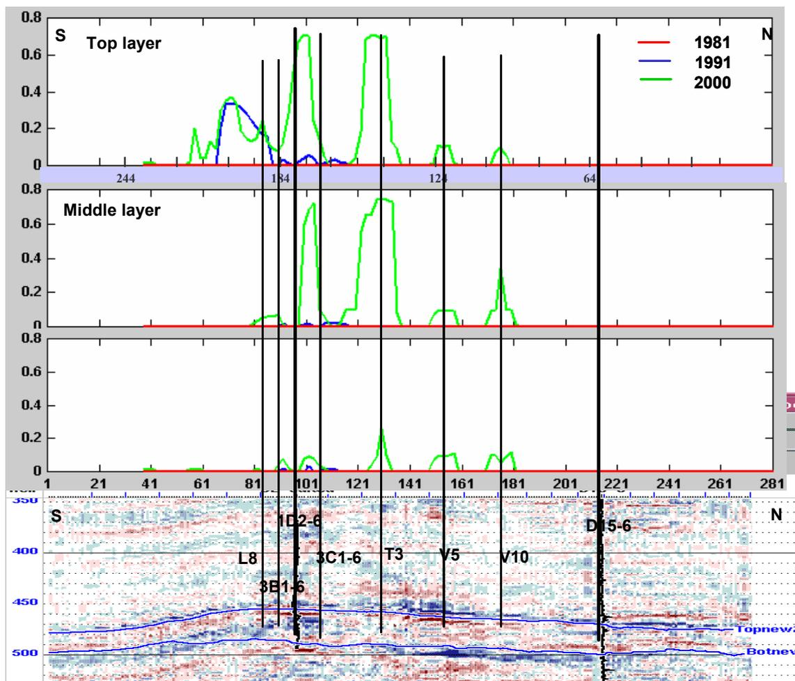
**Figure 6.19: The impedance difference vs. gas saturation from reservoir simulation.**
