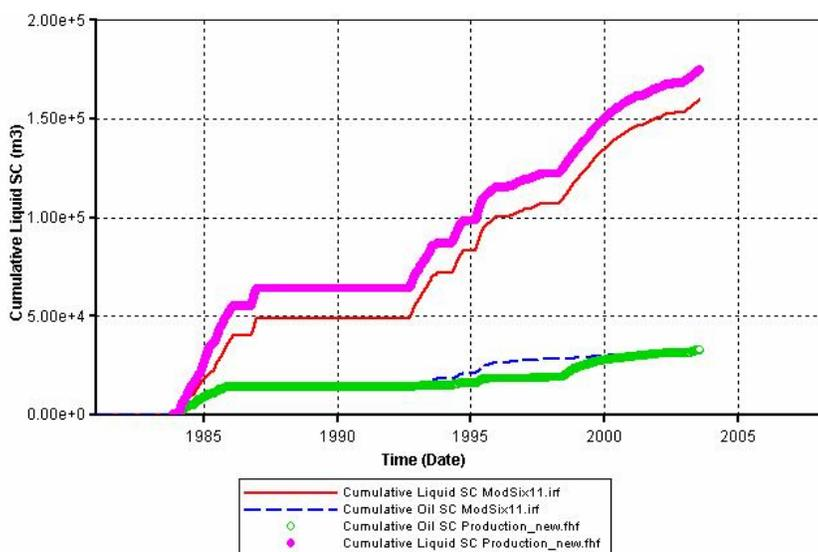
**Figure 4.2** History matching results of the cumulative liquid and cumulative oil production for well 1D2-6 in standard condition. The pink dots are the cumulative liquid productions from the history file. The red line is the cumulative liquid production from the simulation output. The green dots are the cumulative oil production from the history file. The blue dash line is the cumulative oil production from the simulation output.
