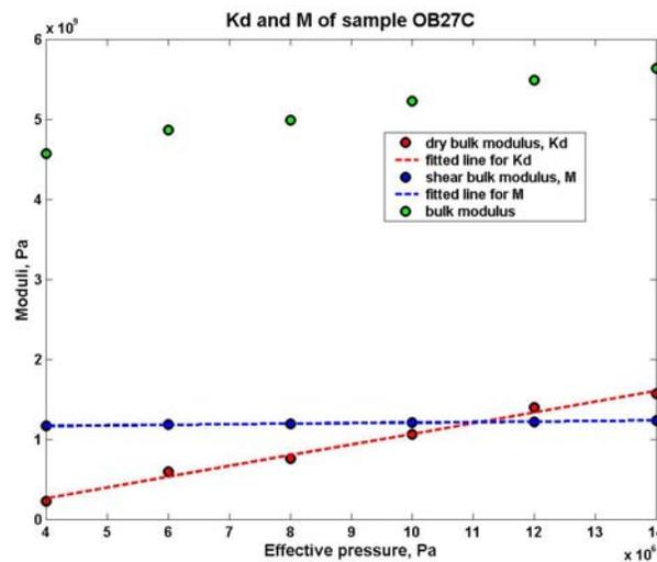
**Figure. 2.8 Dry bulk modulus, shear modulus and the fitted lines for sample OB27C.**
