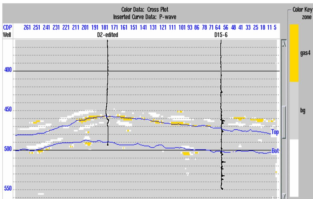
Figure 6.15 Cross section of the 2000 seismic AVO analysis.
