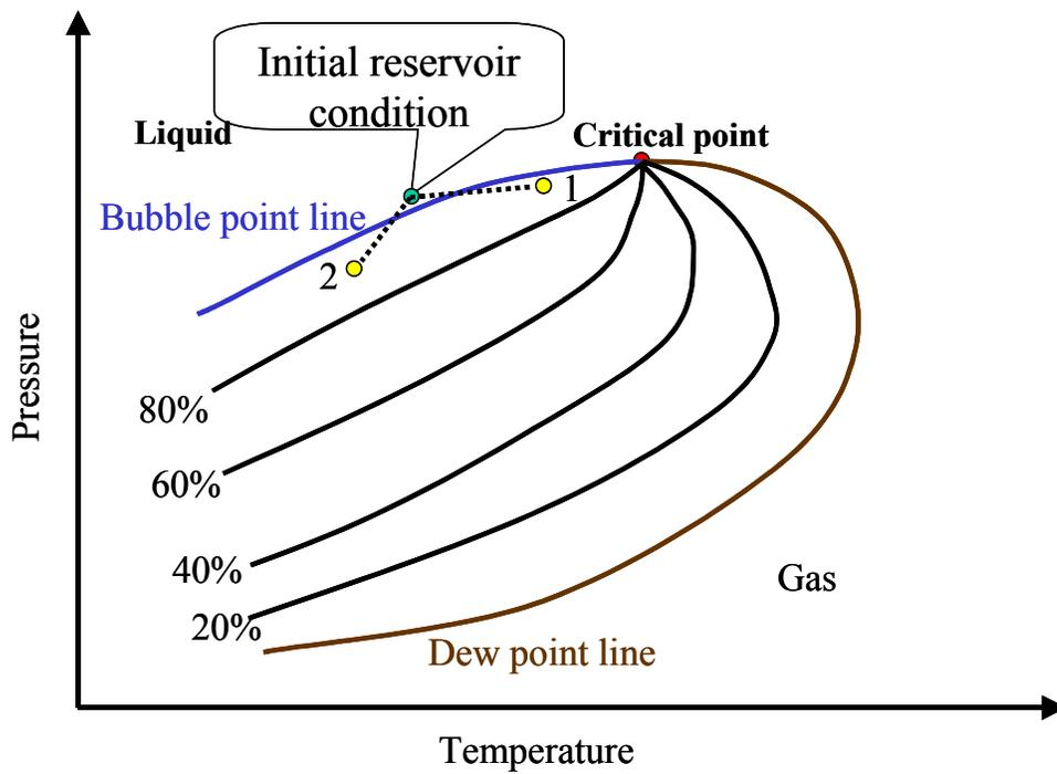
**Figure 4.7 Hydrocarbon phase diagram in the pressure-temperature plane with contours of liquid oil saturation relative to gas.**
