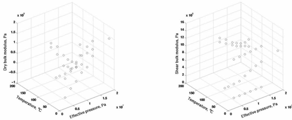
**Figure. 2.9 Lab obtained  $K_d$  (left) and  $\mu$  (right) in effective pressure and temperature space.**
