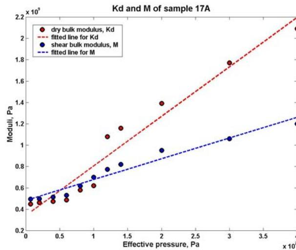
**Figure 2.4 Dry bulk modulus and shear modulus and the fitted lines for sample 17A.**
