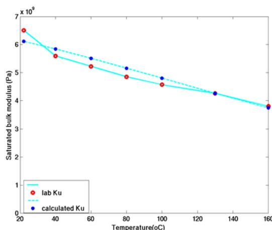
**Figure 2.10 Calculated saturated bulk moduli vs. lab derived saturated bulk moduli.**
