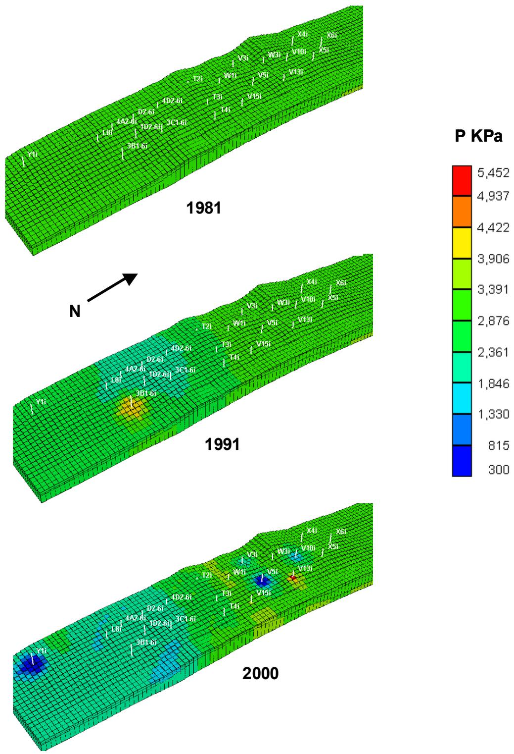
Figure 4.5 Pressure distributions from reservoir simulation at three dates.
