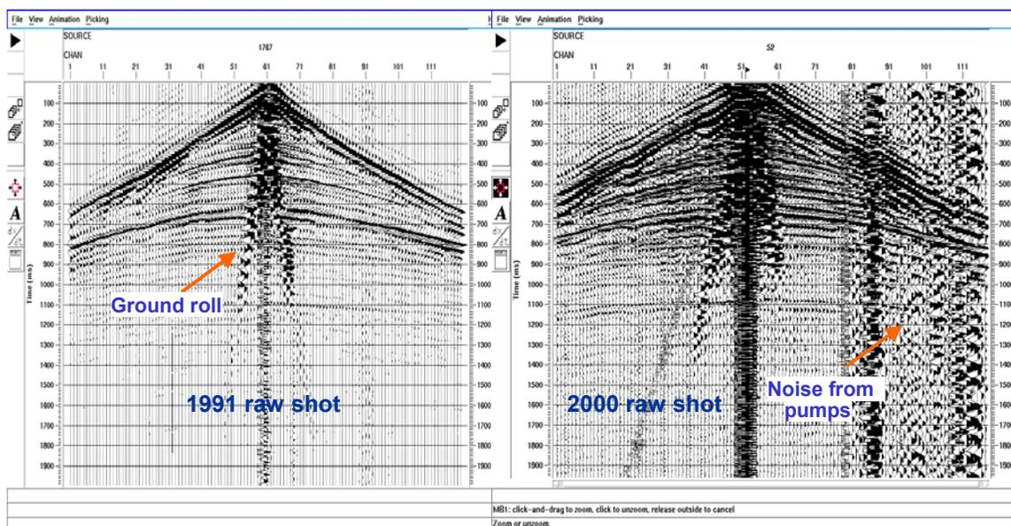
**Figure 3.2** The raw shot from 1991 survey (left) and 2000 survey (right).
