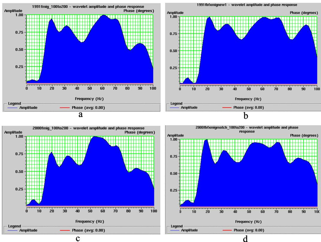
**Figure 3.3 Amplitude spectra before and after post-stack balance. a & c: amplitude spectrum with pre-stack partial spectrum balance for the 1991 and 2000 survey respectively; b & d: amplitude spectrum with pre-stack partial spectrum balance and post-stack spectrum balance for the 1991 and 2000 survey respectively.**
