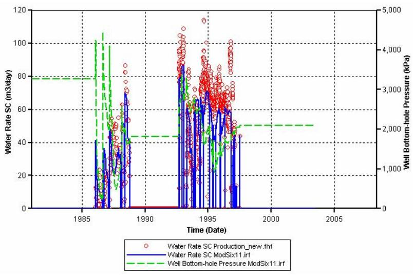
**Figure A.2 History matching results of water rate and bottom hole pressure for well L8. The red dots are the water rate in standard condition from the history file. The blue line is the water rate in standard condition from the simulation output. The green dash line is the well bottom-hole pressure from the simulation output (there is no pressure history file).**
