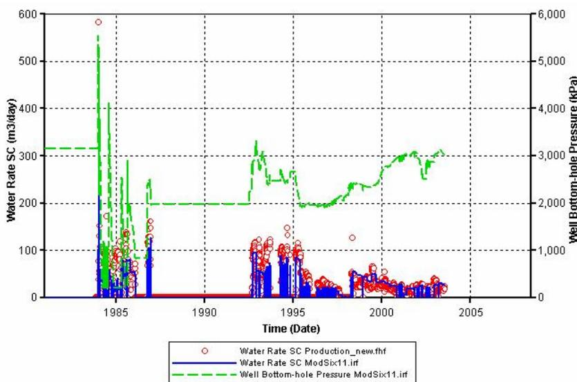
**Figure 4.3** History matching results of the water rate and the bottom hole pressure for well 1D2-6. The red dots are the water rate in standard condition from the history file. The blue line is the water rate in standard condition from the simulation output. The green dash line is the well bottom-hole pressure from the simulation output (there is no pressure history).
