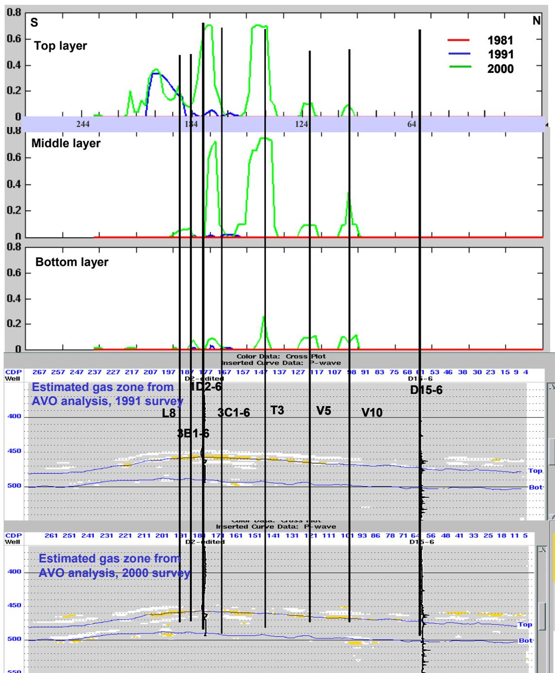
Figure 6.16 The comparison of AVO derived gas zone and the gas saturation from the reservoir simulation. The vertical lines are well positions.
