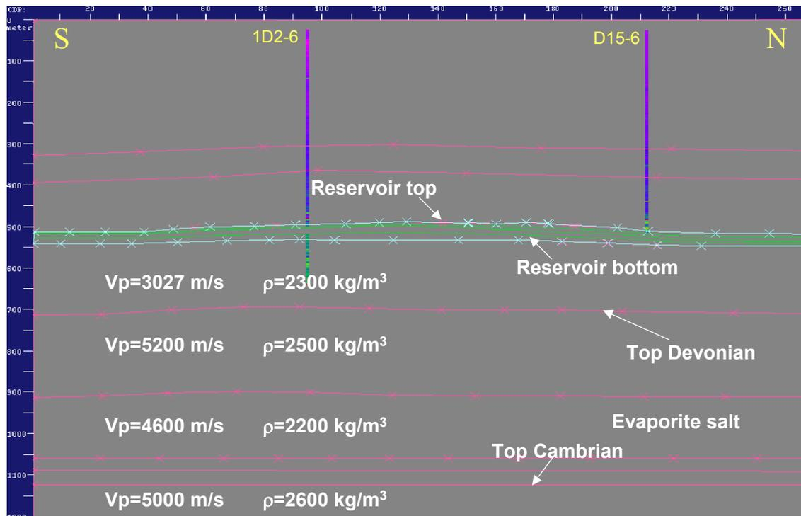
**Figure 5.1 Synthetic seismic model. Above the reservoir velocity and density was interpolated along the structure using well logs at well 1D2-6 and well D15-6, inside reservoir the values were calculated using the output of reservoir simulation and the rock physics procedure, and below the reservoir are average values of well logs from adjacent wells.**
