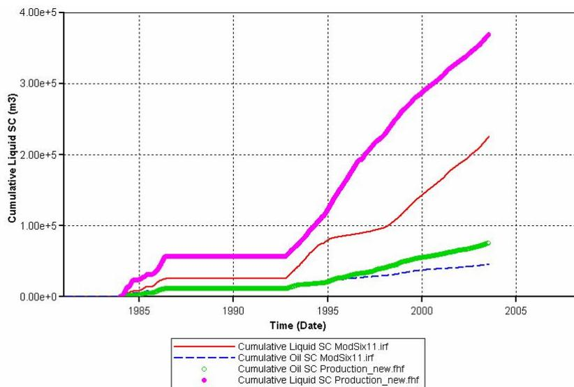
**Figure. A.5 History matching results of cumulative liquid and cumulative oil production for well 3C1-6 in standard condition. The pink dots are the cumulative liquid productions from the history file. The red line is the cumulative liquid production from the simulation output. The green dots are the cumulative oil production from the history file. The blue dash line is the cumulative oil production from the simulation output.**
