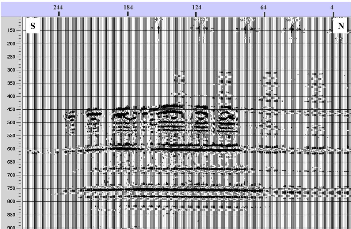
Figure 5.9 The synthetic seismic difference section, the 2000 synthetic section minus the 1991 synthetic section.
