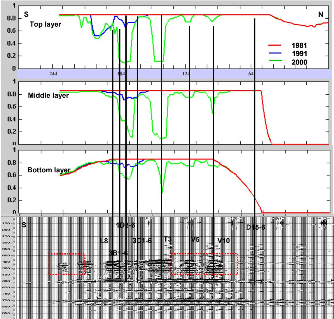
Figure 6.7 Reservoir oil saturation in the three layers (up) and the synthetic difference section (down).
