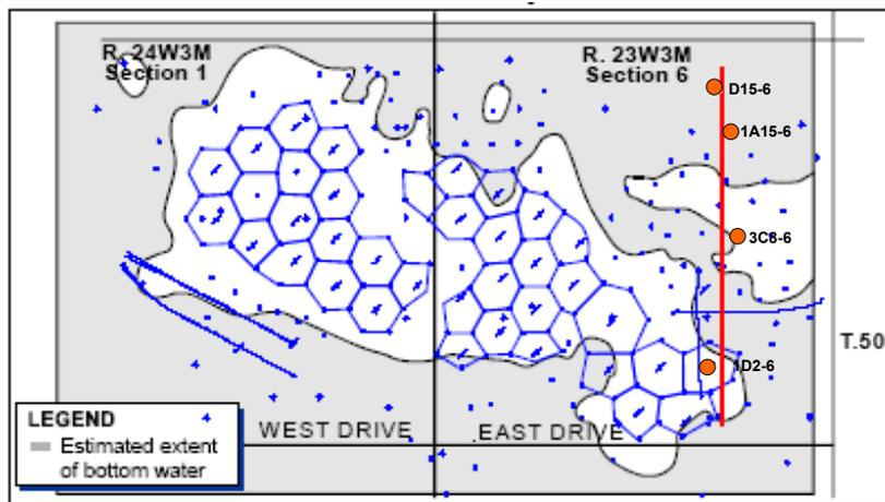
**Figure 1.4** Map of the time-lapse seismic survey location (red line) (modified from Wong et al, 2001). The honey-comb shape is seven point steam drive pattern. Most wells around seismic line are CCS wells.
