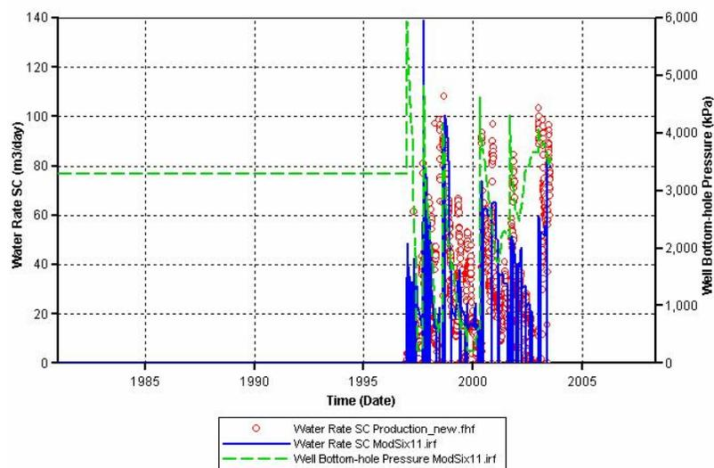
**Figure A.10 History matching results of water rate and bottom hole pressure for well V5. The red dots are the water rate in standard condition from the history file. The blue line is the water rate in standard condition from the simulation output. The green dash line is the well bottom-hole pressure from the simulation output (there is no pressure history file).**
