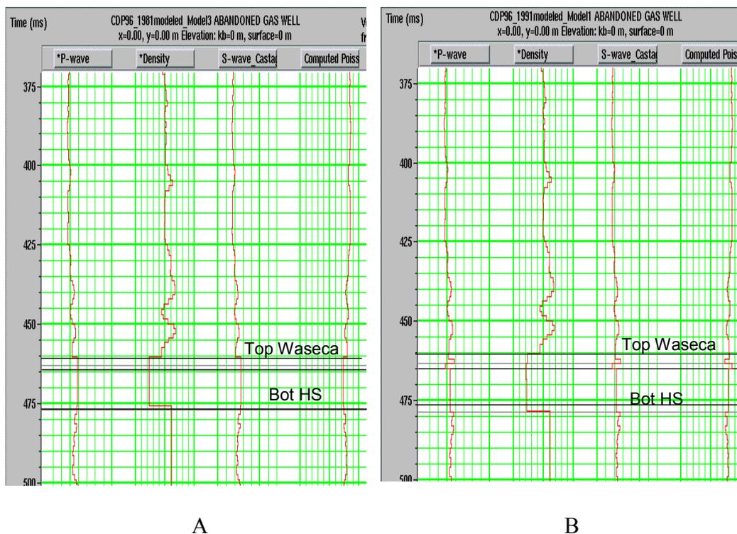
**Figure 6.8 Synthetic logs from velocity and density models calculated from reservoir simulation output. A: synthetic logs before production. B: synthetic logs after production.**
