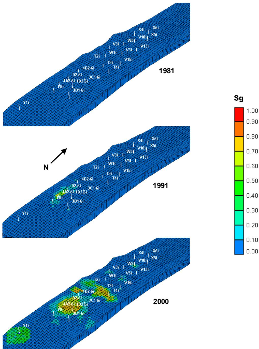
Figure 4.6 Gas saturation distributions from reservoir simulation at three dates.
