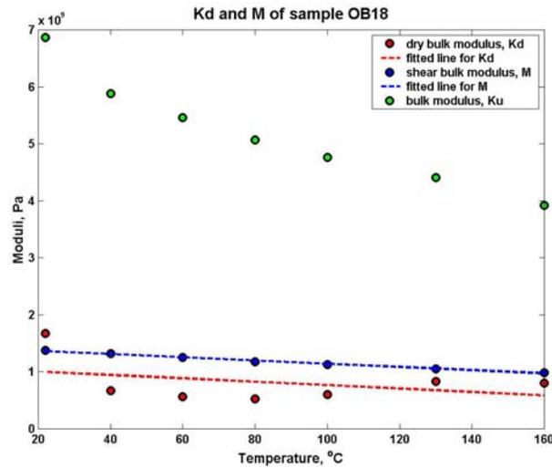
**Figure 2.6 Dry bulk modulus and shear modulus and the fitted lines for sample OB18.**
