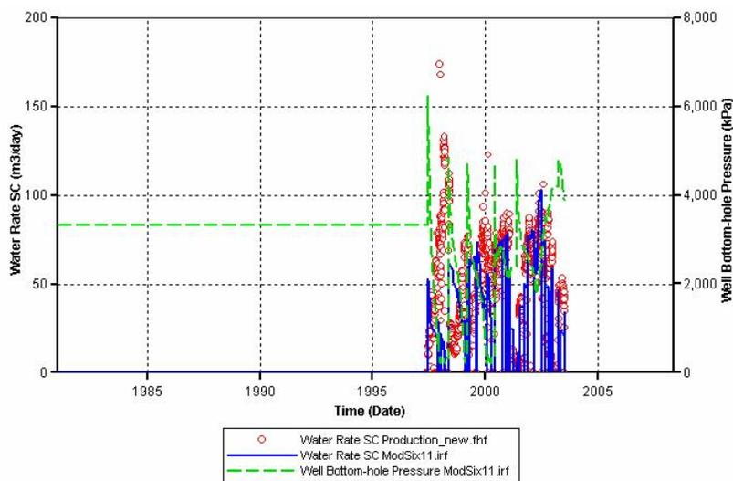
**Figure A.12 History matching results of water rate and bottom hole pressure for well V10. The red dots are the water rate in standard condition from the history file. The blue line is the water rate in standard condition from the simulation output. The green dash line is the well bottom-hole pressure from the simulation output (there is no pressure history file).**
