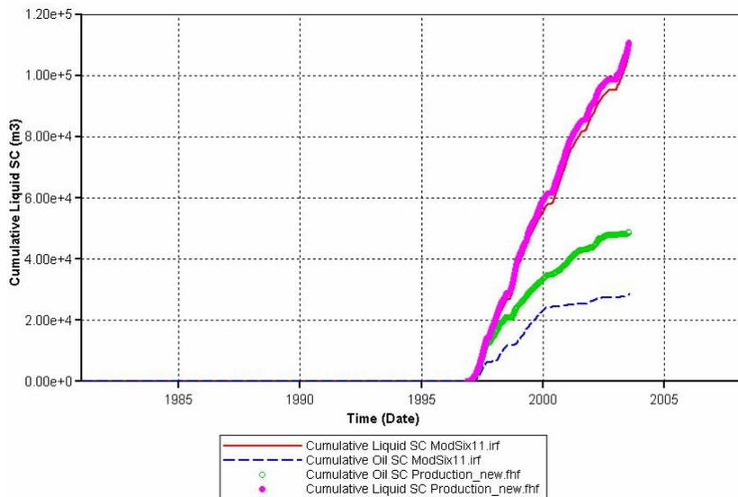
**Figure. A.9 History matching results of cumulative liquid and cumulative oil production for well V5 in standard condition. The pink dots are the cumulative liquid productions from the history file. The red line is the cumulative liquid production from the simulation output. The green dots are the cumulative oil production from the history file. The blue dash line is the cumulative oil production from the simulation output.**
