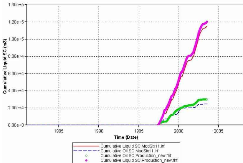
**Figure A.11 History matching results of cumulative liquid and cumulative oil production for well V10 in standard condition. The pink dots are the cumulative liquid productions from the history file. The red line is the cumulative liquid production from the simulation output. The green dots are the cumulative oil production from the history file. The blue dash line is the cumulative oil production from the simulation output.**
