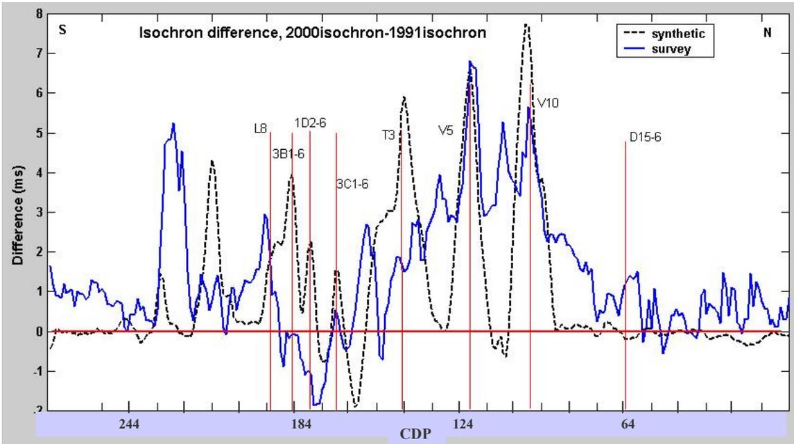
Figure 6.3 Isochron difference comparison. The CDP numbers for the seismic survey sections were converted to the synthetic seismic CDP number for easy comparison.
