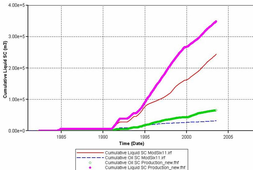
**Figure. A.3 History matching results of cumulative liquid and cumulative oil production for well 3B1-6 in standard condition. The pink dots are the cumulative liquid productions from the history file. The red line is the cumulative liquid production from the simulation output. The green dots are the cumulative oil production from the history file. The blue dash line is the cumulative oil production from the simulation output.**
