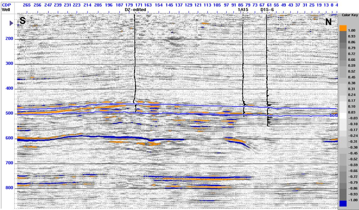
Figure 5.10 The seismic survey difference section, the 2000 final processed section minus the 1991 final processed section.
