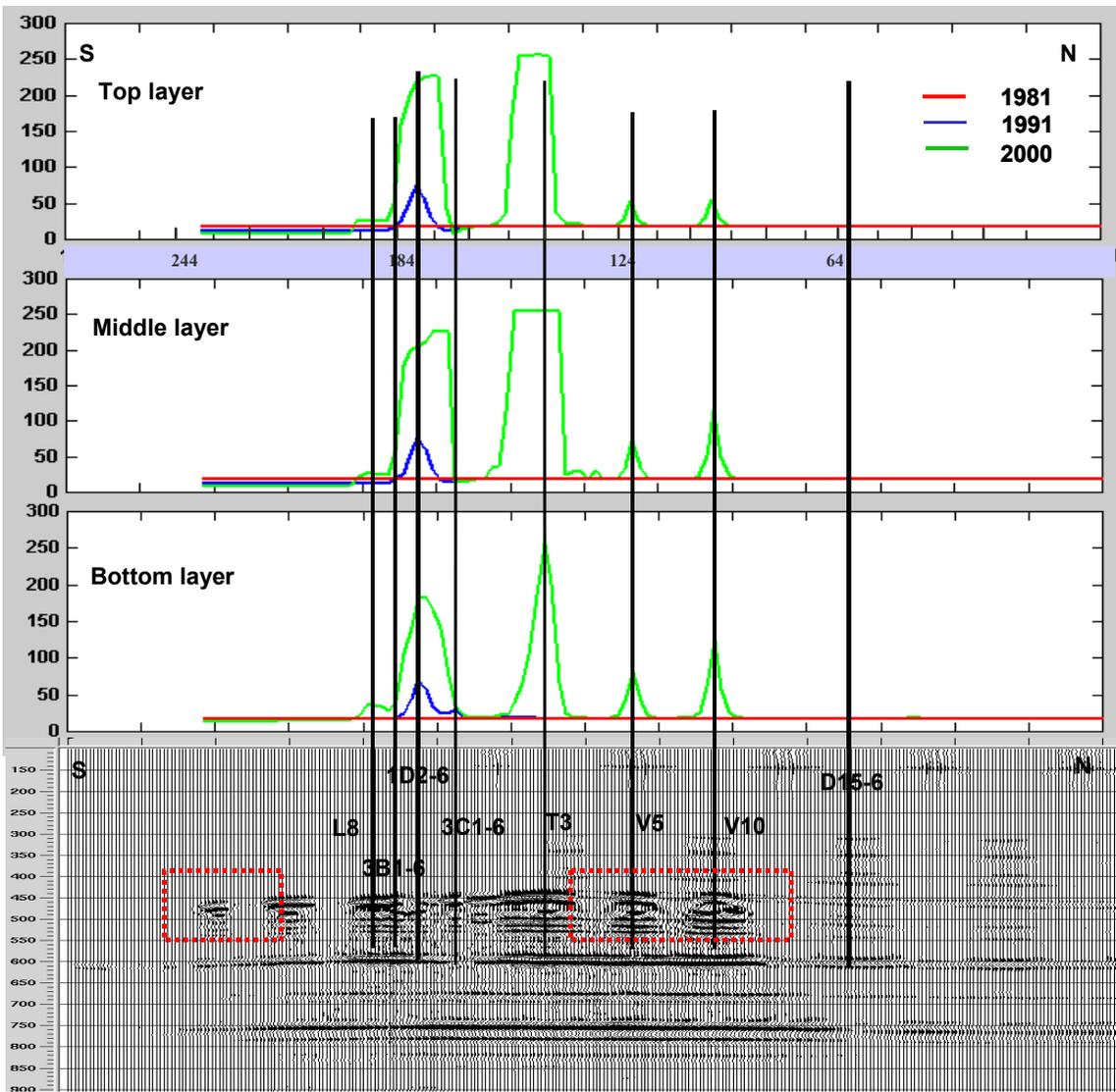
Figure 6.6 Reservoir temperature in the three layers (up) and the synthetic difference section (down).
