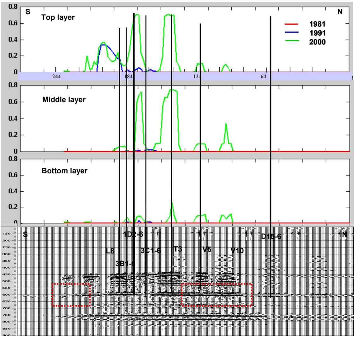
Figure 6.5 Reservoir gas saturation in the three layers (up) and the synthetic difference section (down).
