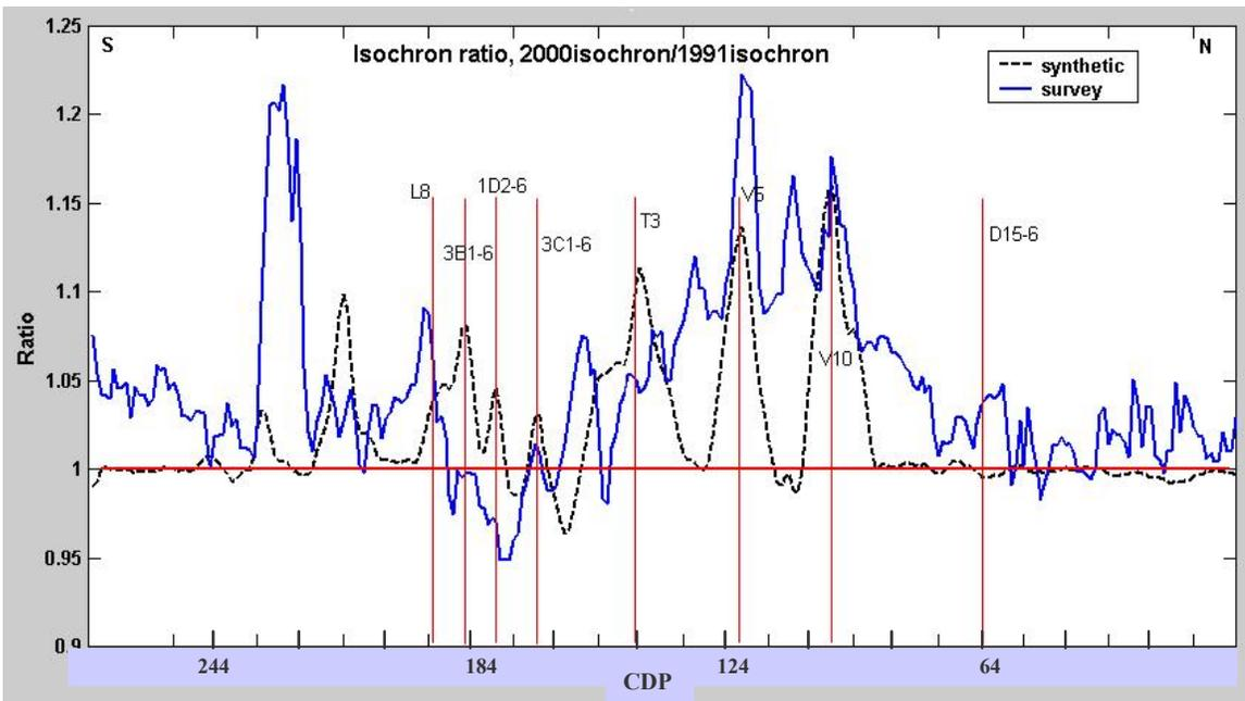
Figure 6.2 Isochron ratio comparison. The CDP numbers for the seismic survey sections were converted to the synthetic seismic CDP number for easy comparison.
