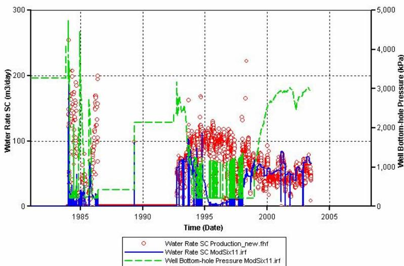
**Figure A.6 History matching results of water rate and bottom hole pressure for well 3C1-6. The red dots are the water rate in standard condition from the history file. The blue line is the water rate in standard condition from the simulation output. The green dash line is the well bottom-hole pressure from the simulation output (there is no pressure history file).**
