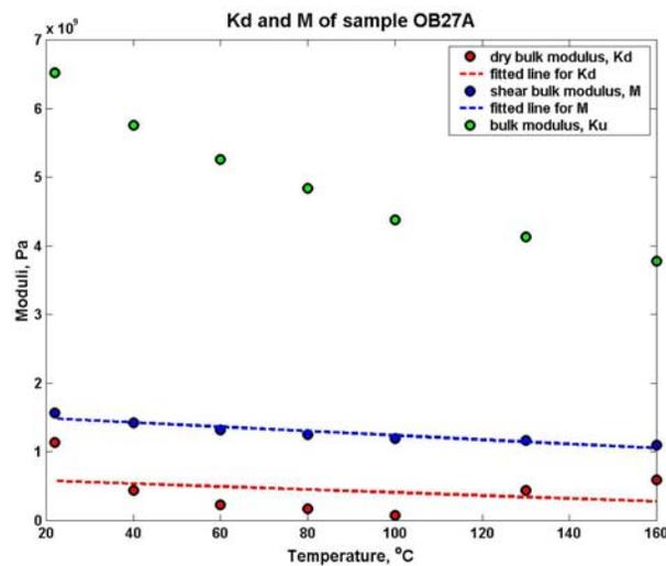
**Figure 2.5 Dry bulk modulus and shear modulus and the fitted lines for sample OB27A.**
