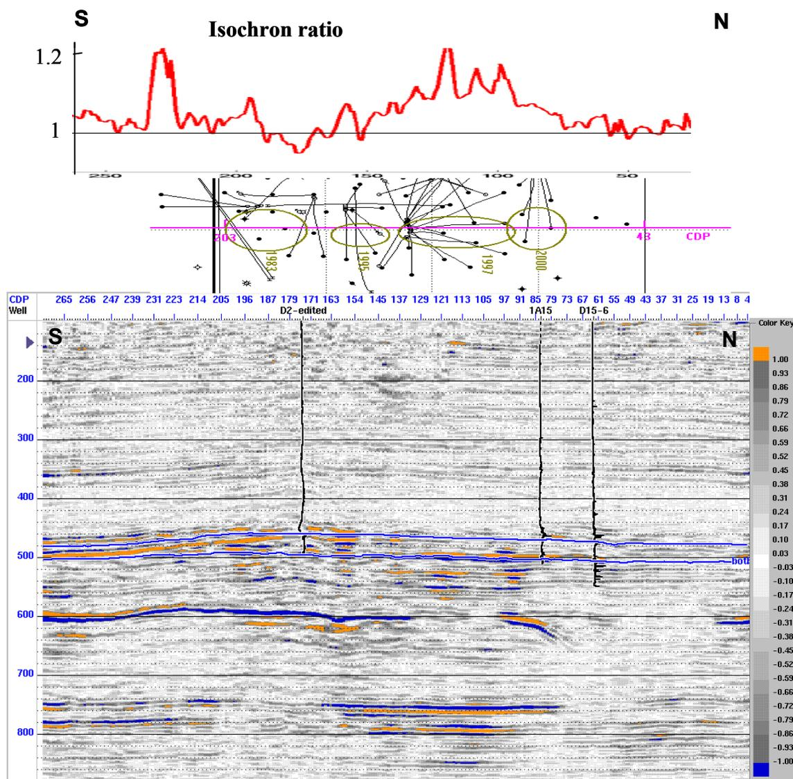
**Figure 3.7** Difference section from conventional scaling (bottom, in relative scale from  $-1$  to  $1$ ) with well activities (middle, circles mark the drilling time) and isochron ratio (top, which is the isochron of the 2000 survey divided by the one from the 1991 survey).
