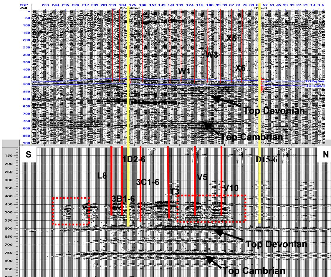
**Figure 6.1** The difference sections between the 2000 stack and the 1991 stack from real seismic survey (up) and synthetic seismic modeling (down).
