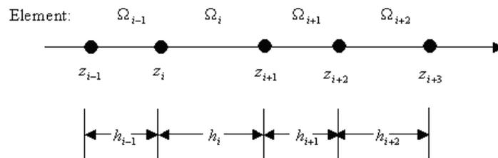
Figure 3.1 The discretization along the  $z$  direction by FEM.
