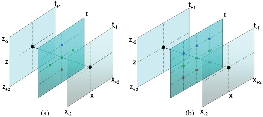
Figure 2.1 FD and FE-FD operators: (a) conventional 2<sup>nd</sup> order FD operators; (b) 2<sup>nd</sup> order FE-FD operators.
