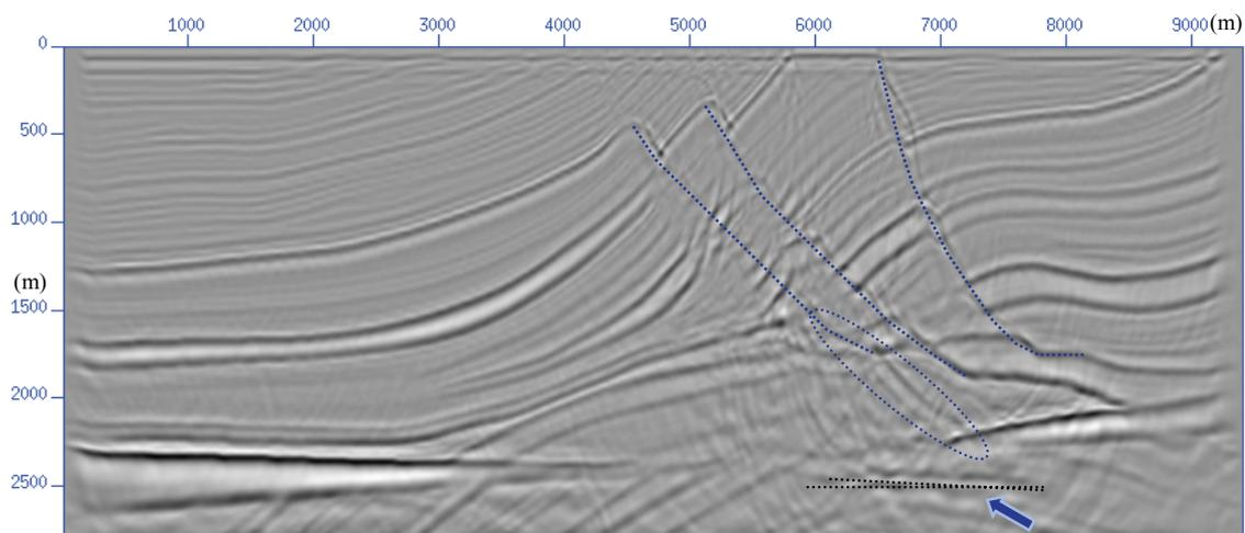
Figure 8.12 Isotropic implicit FD migration result with the vertical velocity shown in Figure 8.10. The fault planes are not in their correct positions, delineated by blue curves; the diffraction energy can't be focused; the anticline is distorted (dashed ellipse); and the objective target zone (dashed black lines) obliquely moves up.
