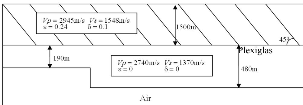
Figure 5.14 Model of an isotropic reef with an anisotropic overburden from the Foothills Research Project showing the 45° dipping anisotropic overburden above horizontal reflectors. The Plexiglas layer is isotropic.
