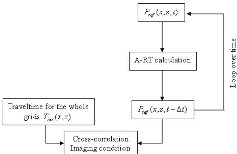
Figure 5.7 The wavefield extrapolation scheme for prestack anisotropic reverse-time migration
