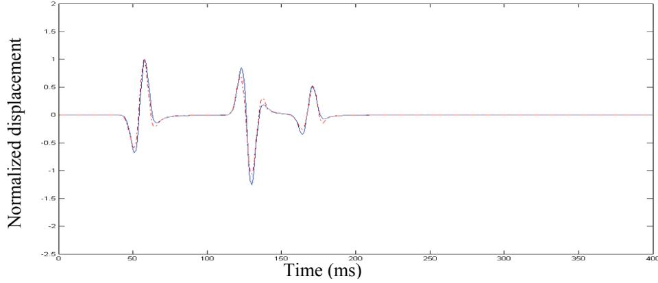
Figure 3.5 Seismogram at the given observer position (Table 3.1). The solid blue line represents the analytical solution, and the dashed red line represents the numerical solution by the FE-FDM.
