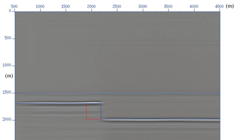
Figure 5.19 Prestack anisotropic reverse-time migration result from the reef model with an exact velocity model and Thomsen parameters. Anisotropic migration provides a correct image, and the events exactly fit the interfaces.
