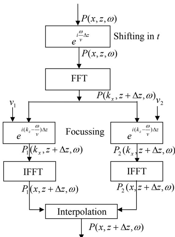
Figure 4.3 The extrapolation scheme for PSPI.
