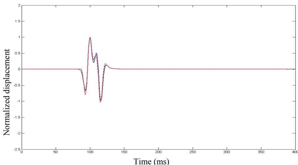
Figure 3.9 Seismogram at the given observer position (Table 3.2). The solid blue line is the analytical solution and the dashed red line is the numerical solution from FE-FDM with irregular grids.
