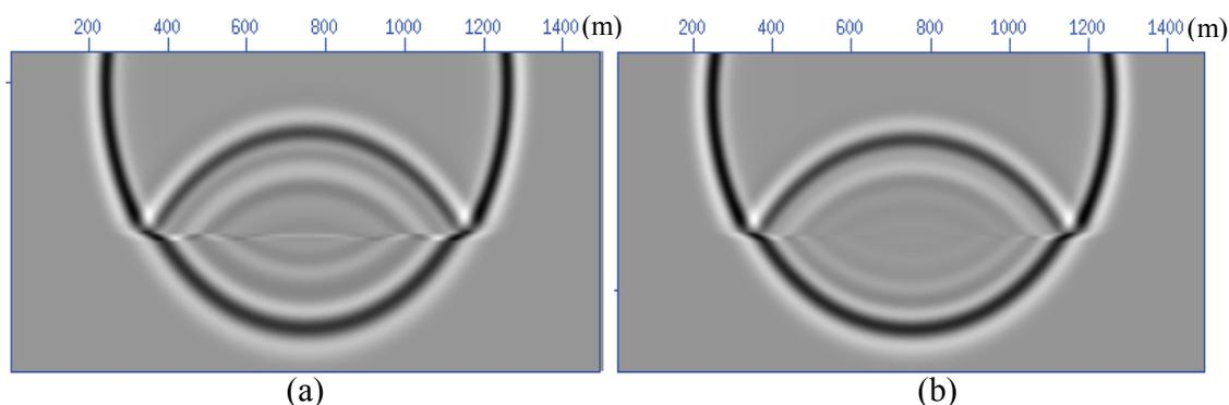
Figure 3.11 (a) Snapshot of the wavefield ( $t=0.15s$ ) with the regular grids, and (b) snapshot of the wavefield ( $t = 0.15s$ ) with the irregular grids.
