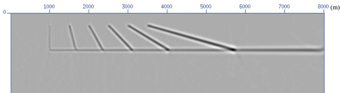
Figure 8.5 Migration result from the anisotropic implicit FD method with 4<sup>th</sup> order accuracy coefficients obtained using the optimized method.
