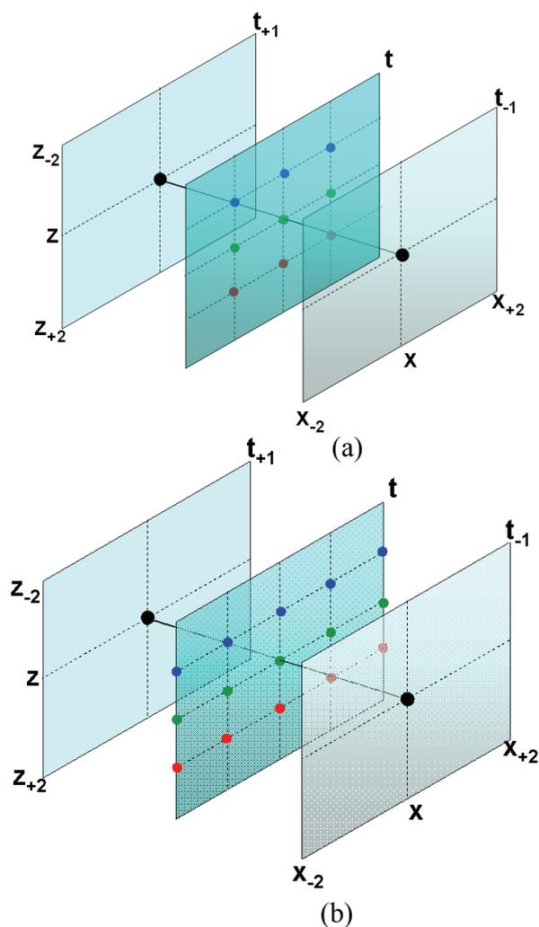
Figure 3.3 The grid computation in the space and time domains; (a) is the  $2^{\text{nd}}$  order accuracy finite-difference in the  $x$  direction with the linear element along the depth direction; (b) corresponds to the  $4^{\text{th}}$  order accuracy finite-difference in the  $x$  direction.
