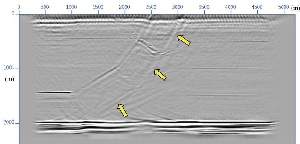
Figure 7.20 Prestack anisotropic reverse-time migration result from the TTI thrust model.
