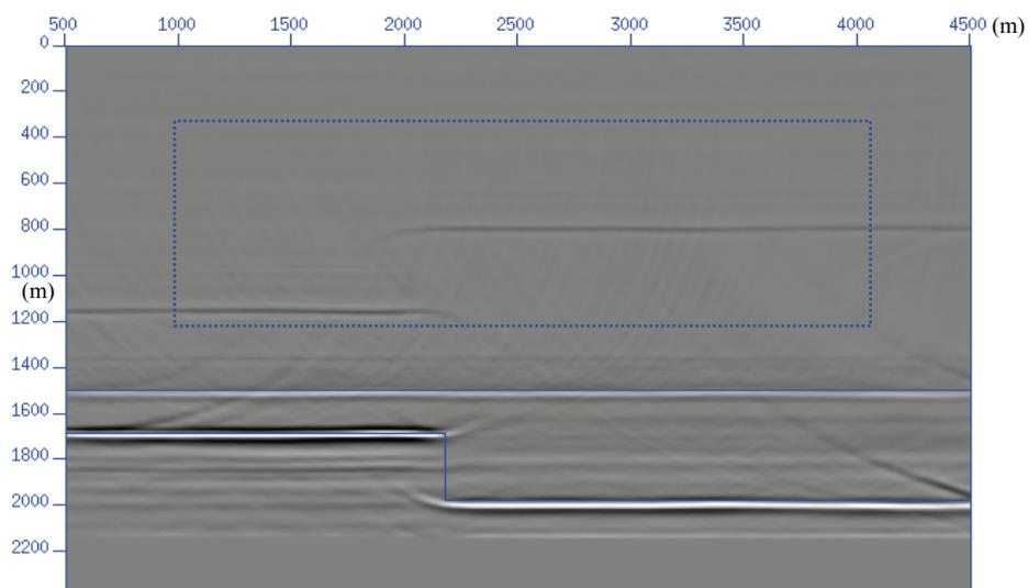
Figure 5.17 Anisotropic migration result from the reef model with an exact velocity model and Thomsen parameters. Anisotropic migration provides a correct image, and the events exactly fit the interfaces.
