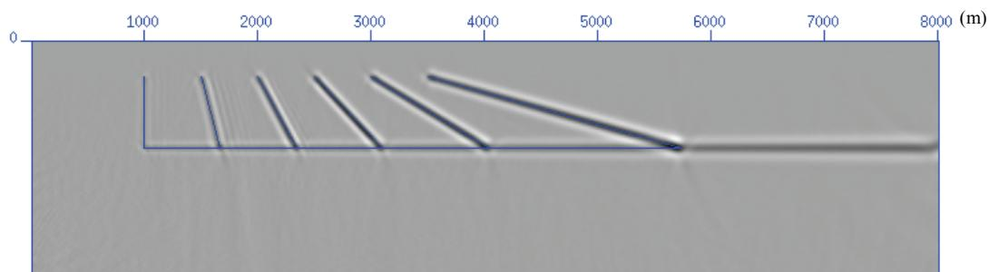
Figure 8.8 Migration result from the anisotropic implicit FD method with 4<sup>th</sup> order accuracy coefficients obtained through the optimized method.
