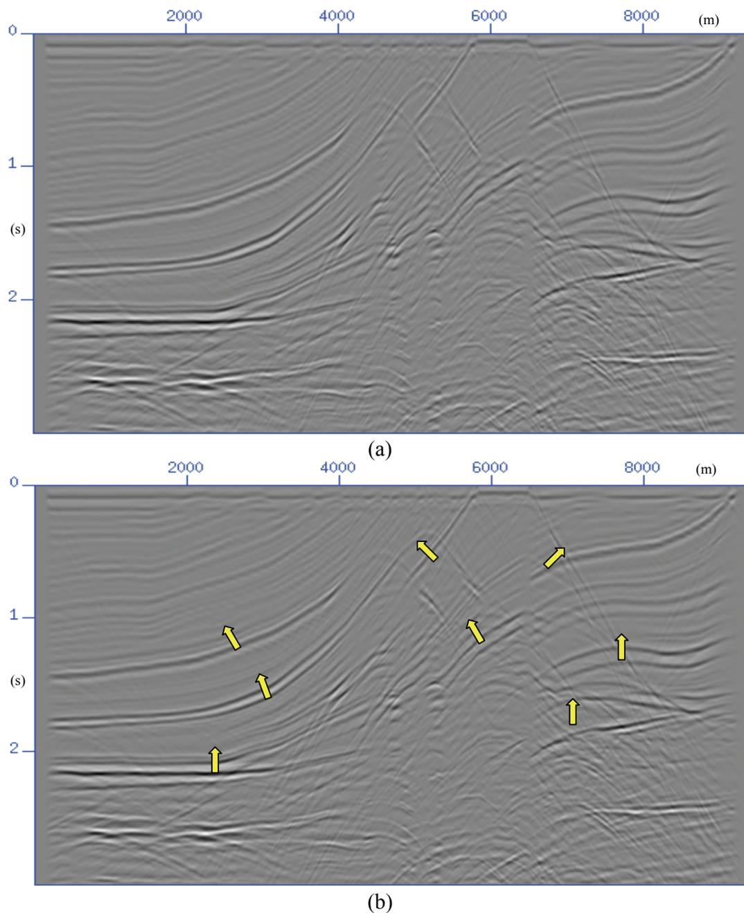
Figure 8.11 Zero-offset seismic sections from the pseudo-spectral method: (a) isotropic synthetic data based on the acoustic wave equation; (b) anisotropic synthetic data based on the anisotropic P-wave equation (Du et al., 2005). All the events from the anisotropic modelling in subfigure (a) move up due to the effect of anisotropy when compared with those from the isotropic modelling in subfigure (b), as indicated by the yellow arrows.
