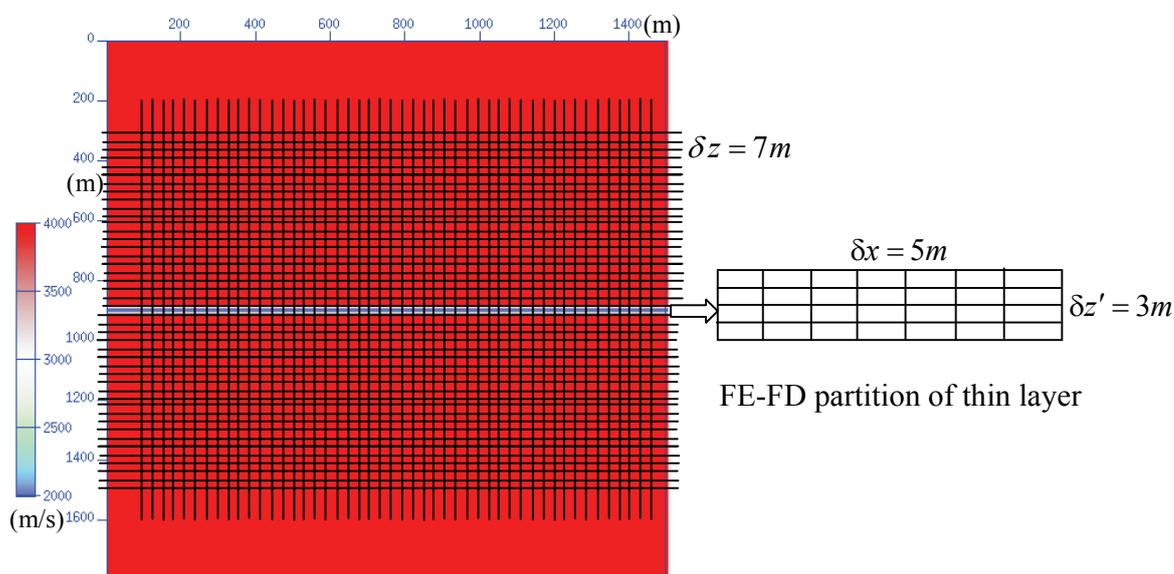
Figure 3.10 The velocity model and the grid partitions.
