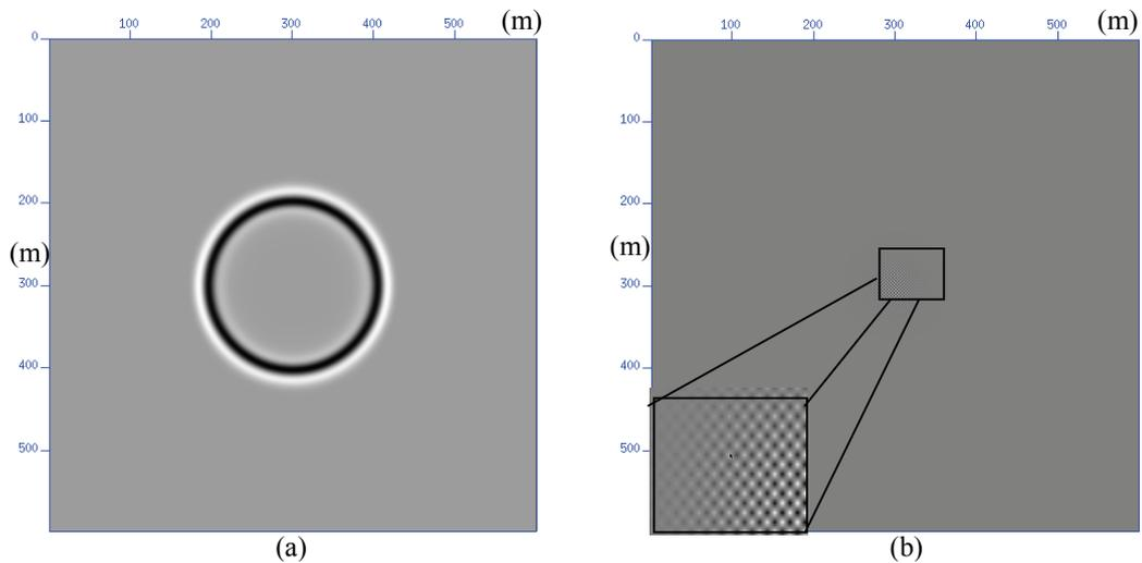
Figure 3.8 Modelling results from the FDM and FE-FDM methods. (a) Modelling by FE-FDM with 2<sup>nd</sup> order accuracy in the spaces. (b) Same modelling by 2<sup>nd</sup> order central FDM.
