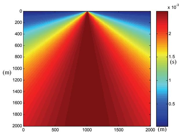
Figure 3.19 The traveltime absolute difference between the analytical and finite-difference solutions.
