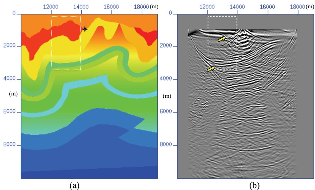
Figure 4.10 (a) Velocities used for migrating the shot shown in Figure 4.7; (b) the migration of the shot gather using the prestack SSF method. The yellow arrows shown in (b) indicate the imaging quality for shallow structures.
