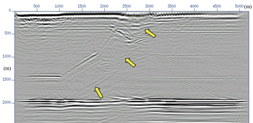
Figure 7.15 Prestack anisotropic PSPI depth migration result from the TTI thrust model.
