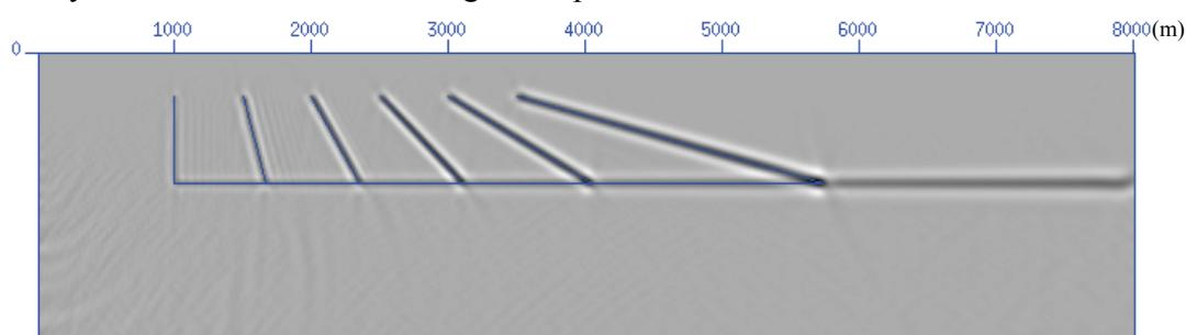
Figure 8.9 Migration result from the anisotropic implicit FD method with 6<sup>th</sup> order accuracy coefficients obtained through the optimized method.
