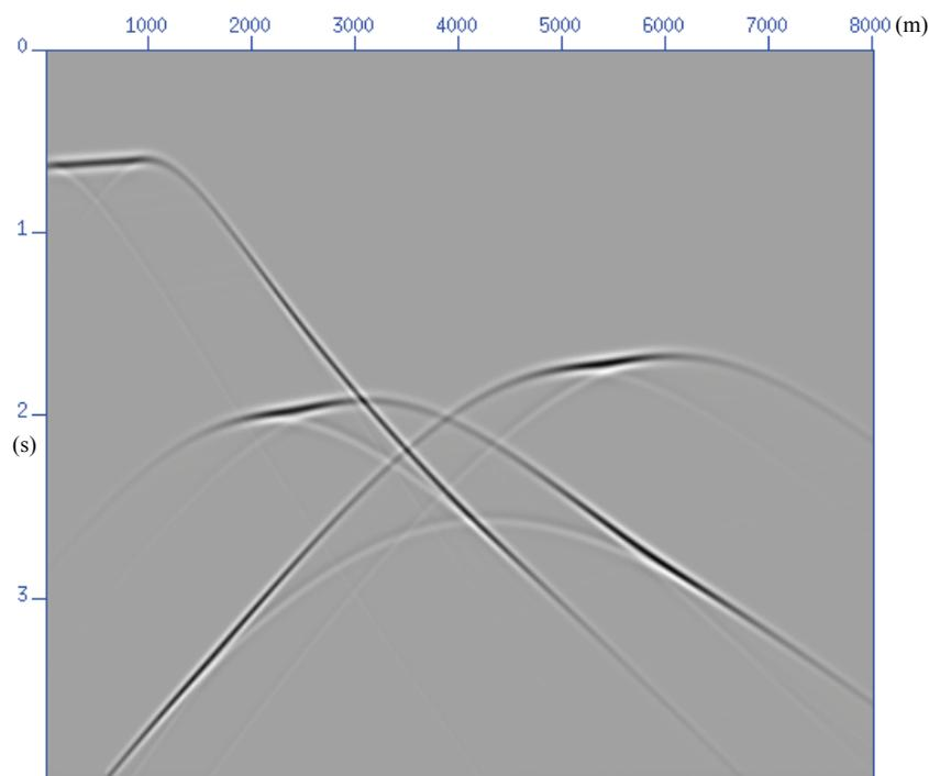
Figure 6.6 Synthetic zero-offset seismogram obtained using an SU routine from the Center for Wave Phenomena (CWP) for the structural model shown in Figure 6.5 in tilted TI media.
