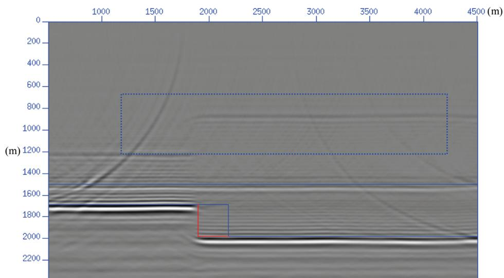
Figure 5.16 Isotropic reverse-time migration result for the reef model. The measured velocity along the vertical direction for the anisotropic overburden and the exact velocity of the isotropic layer are used. The isotropic migration images the reef edge  $\sim 350$  m left of its true position. The blue lines represent the true reef interface while the red lines denote the misplaced migration position.
