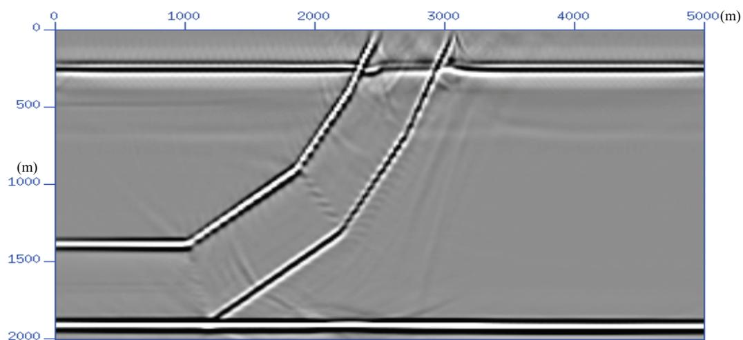
Figure 7.29 The prestack anisotropic RT migration result with correct velocity and anisotropy parameters.
