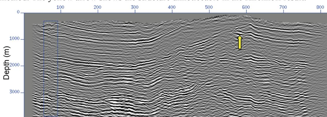
Figure 4.16 The result of prestack SSF depth migration with a constant velocity of 4,200m/s after elevation correction with filed statics. The dashed blue rectangle shows the phenomena of traces “shaking”, and the arrow indicates the changed shape of the reflection event when compared with the results in Figures 4.13 and 4.14.
