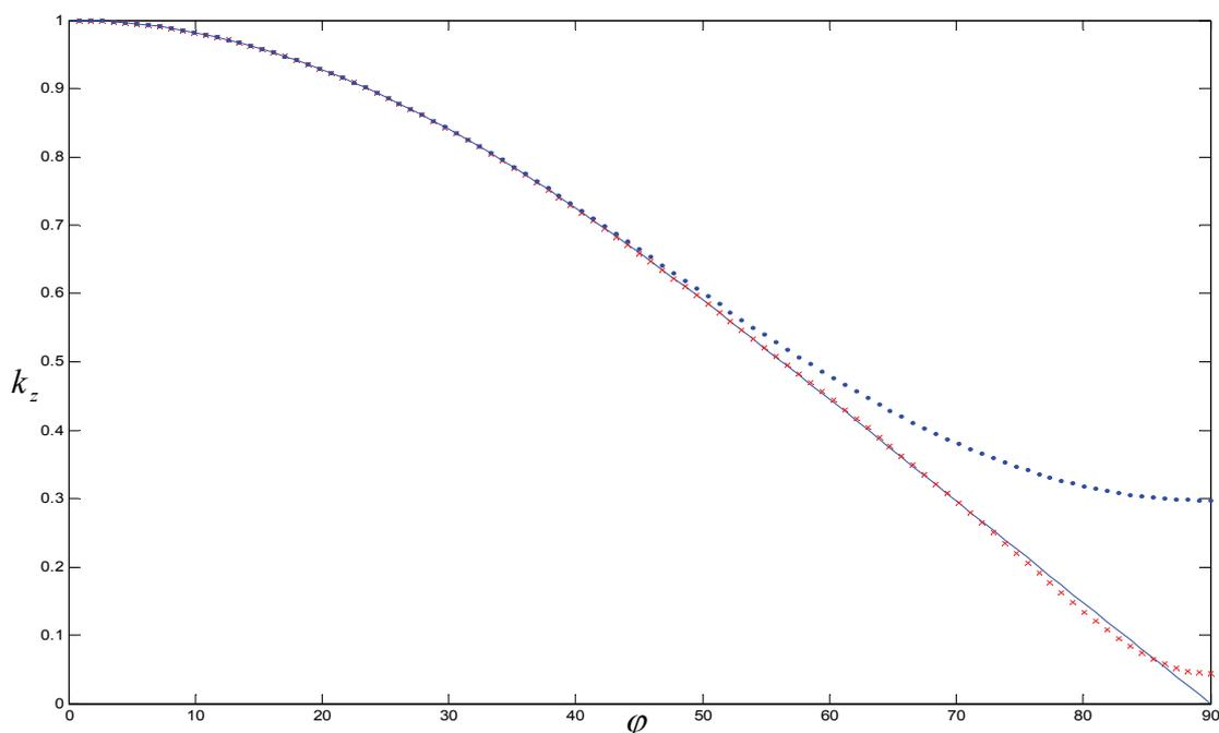
Figure 8.2 The relationship curve of the vertical wavenumber versus phase angle for anisotropy parameters  $\varepsilon = 0.2$ ,  $\delta = 0.1$  in Figure 8.1: blue solid line is the true dispersion relation; blue dashed point is the approximation dispersion by Taylor-series analysis; line indicated by red crosses is the approximation dispersion by the 4<sup>th</sup> order optimization.
