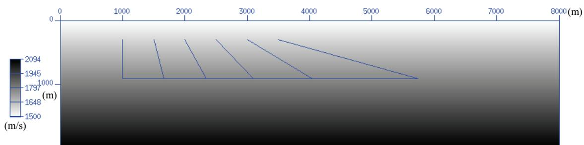
Figure 8.15 Vertical variable velocity  $v(x, z) = 1,500 + 0.3z$  (m/s).
