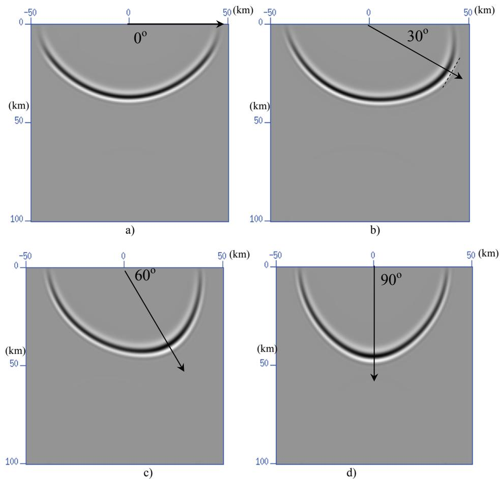
Figure 5.8 P-wave impulse response. (a), (b), (c) and (d) correspond to the results from symmetry axis tilt angles of  $0^\circ$ ,  $30^\circ$ ,  $60^\circ$ , and  $90^\circ$  as indicated by the arrows. The vertical velocity of the P-wave is 3,500m/s and that of the SV-wave is 1,500m/s. The homogenous medium has Thomsen parameters of  $\varepsilon = 0.25$  and  $\delta = 0.1$ .
