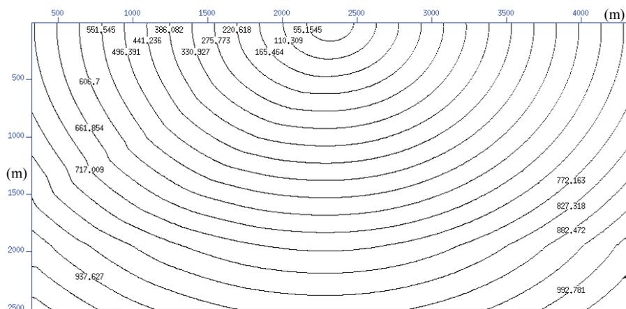
Figure 7.16 The traveltime contours ignoring the anisotropic effect when the source position is located at the centre of the model.
