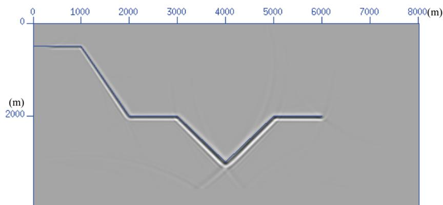
Figure 5.13 Migration result from the anisotropic reverse-time migration method. The exact velocity model and Thomson parameters have been applied. The migration result exactly matches the true interfaces.
