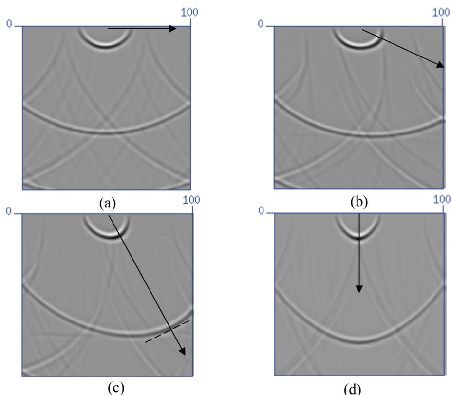
Figure 6.4 P-wave impulse responses. (a), (b), (c) and (d) correspond to the results of tilt angles of  $0^\circ$ ,  $30^\circ$ ,  $60^\circ$ , and  $90^\circ$  as indicated by the arrows.
