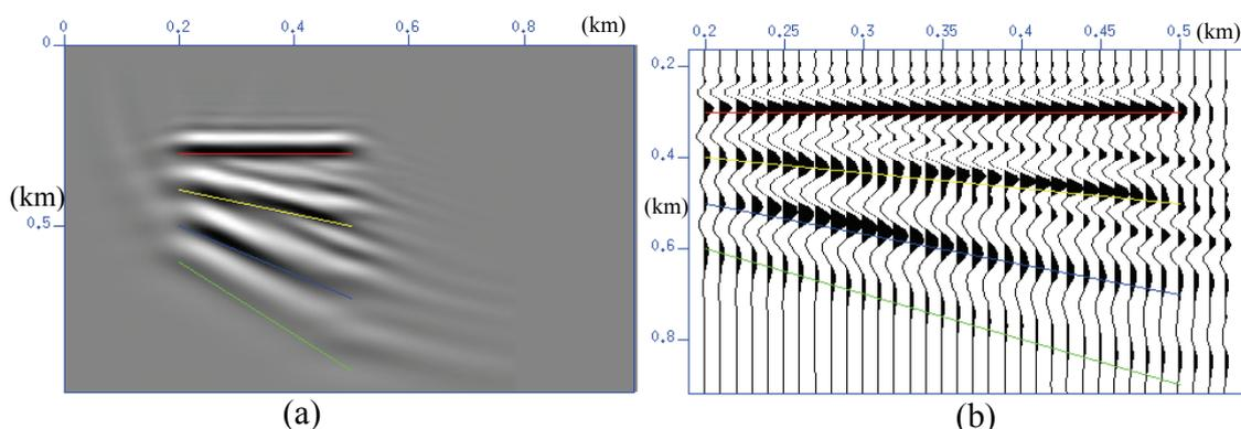
Figure 3.16 (a) A greyscale display of the reverse-time migration result ( $\Delta z = 0.15m$ ), and (b) a wiggle trace display.
