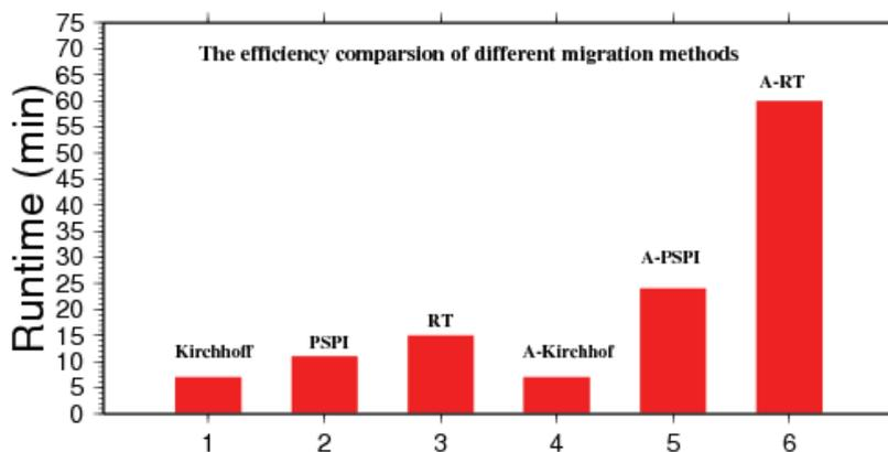
Figure 7.21 Efficiency comparison of the different methods used with the TTI thrust model (Prestack depth migration).
