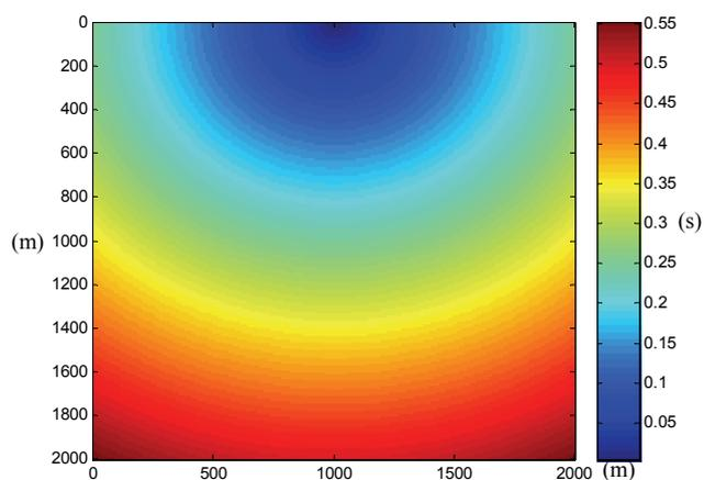
Figure 3.18 The traveltim contour in homogenous media with the upwind finite-difference solution.
