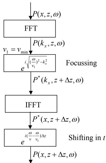
Figure 4.2 The extrapolation scheme for SSF.
