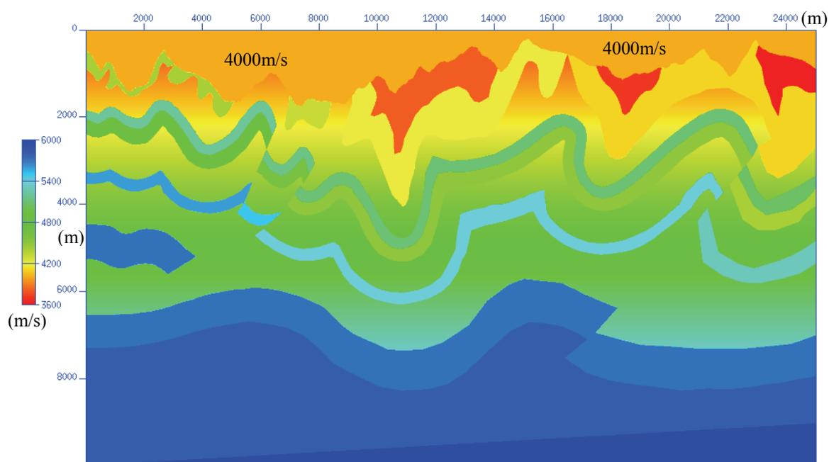
Figure 4.5 A velocity/depth model representative of northeastern British Columbia (after Gray and Marfurt, 1995). There is roughly 1600m of elevation relief along the seismic section.
