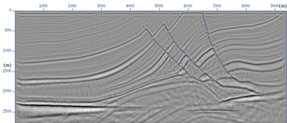
Figure 8.13 Anisotropic implicit FD migration result with the vertical velocity and anisotropy parameters in Figure 8.10. The fault planes are in accord with the true model as the anisotropic effect of the overburden is accounted for. The reflections are correctly migrated to their true positions, as is the target zone.
