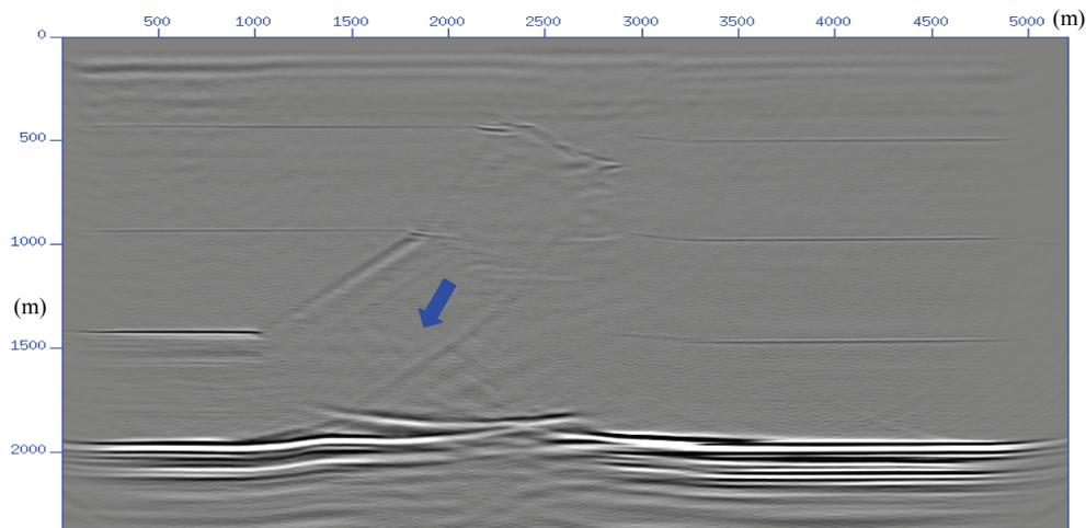
Figure 7.19 Prestack isotropic reverse-time migration result from the TTI thrust model.
