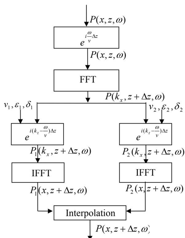
Figure 6.2 The wavefield extrapolation scheme for anisotropic PSPI.
