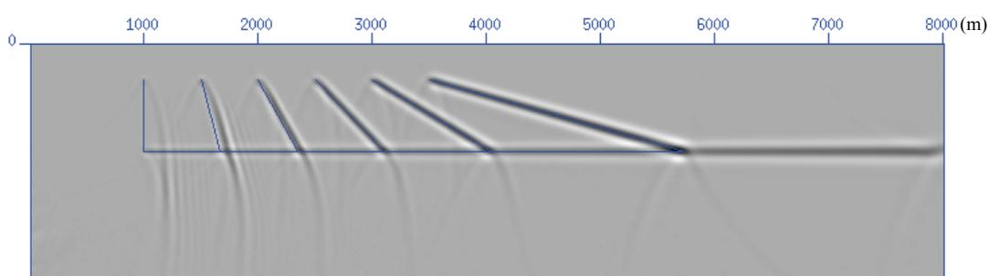
Figure 8.4 Migration result from the anisotropic implicit FD method with coefficients obtained using the Taylor-series expansion method.
