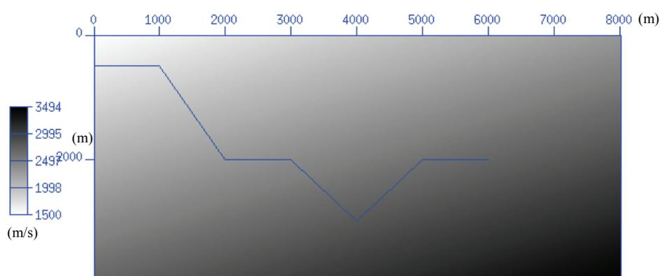
Figure 6.5 Variable velocity model with homogenous Thomsen parameters  $\varepsilon = 0.2$  and  $\delta = 0.1$ , and a tilt angle  $\phi = 60^\circ$ . P-wave velocities parallel to the axis of symmetry vary along the distance and depth as  $v(x, z) = 1,500 + 0.3z + 0.1x$  (m/s).
