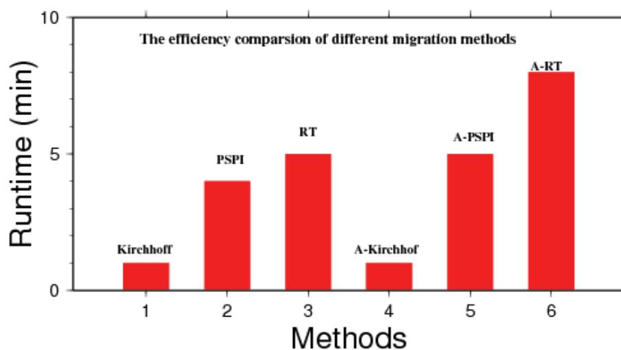
Figure 7.8 Efficiency comparison of the different methods (Post-stack depth migration).
