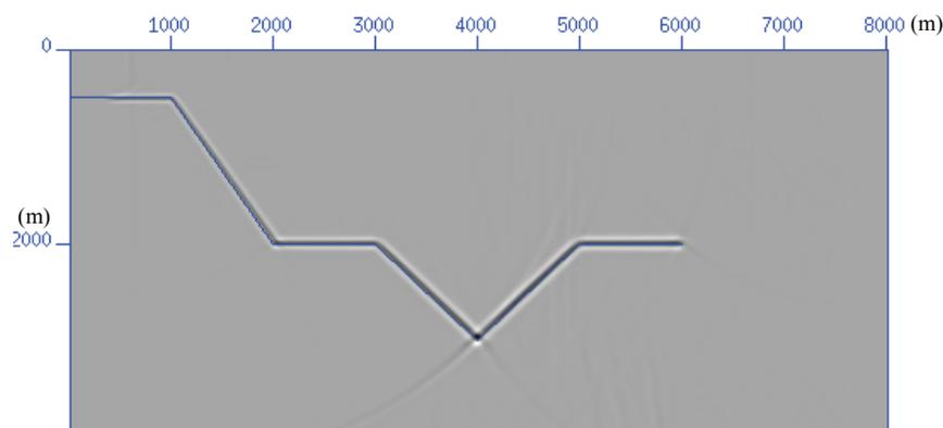
Figure 6.8 Migration result from the anisotropic PSPI migration method. The P-wave velocity model in Figure 6.5 is used taking into account the effect of anisotropy. The blue lines represent the true position of interfaces, and the true position exactly matches with the migration result of A-PSPI.
