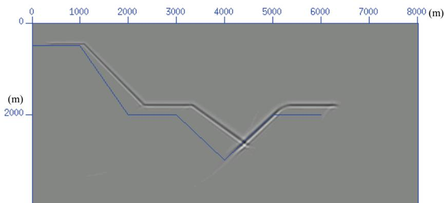
Figure 5.12 Migration result from the isotropic reverse-time migration method. The P-wave velocity model in Figure 5.10 is used without taking into consideration the effect of anisotropy. The blue lines represent the true position of interfaces.
