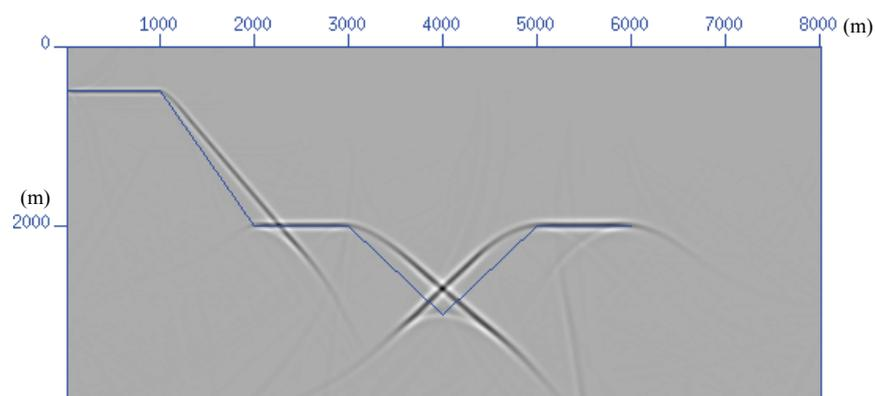
Figure 6.7 Migration result from the isotropic PSPI migration method. The P-wave velocity model in Figure 6.5 is used without considering the effect of anisotropy. The blue lines represent the true position of interfaces.
