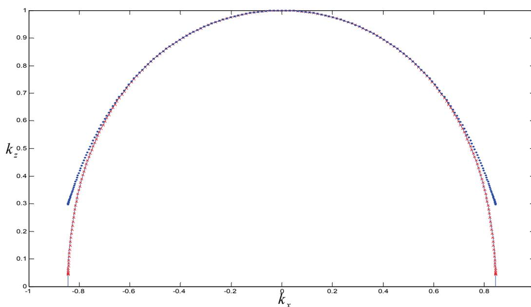
Figure 8.1 Dispersion relationship for anisotropy parameters  $\varepsilon = 0.2$ ,  $\delta = 0.1$ : blue solid line is the true dispersion relation; blue dashed point is the approximation dispersion by Taylor-series analysis; red cross is the approximation dispersion by the 4<sup>th</sup> order optimization.
