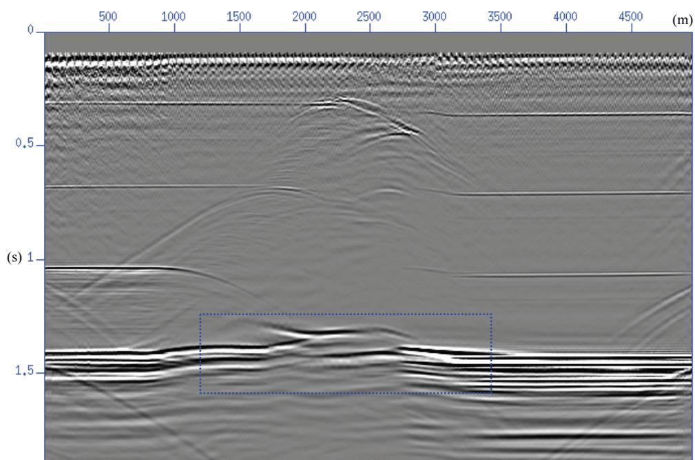
Figure 7.10 Zero-offset seismic section of the TTI thrust model.
