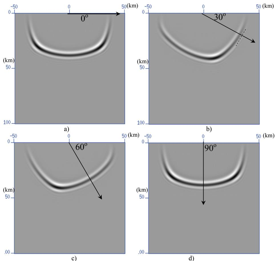
Figure 5.9 SV-wave impulse responses. (a), (b), (c) and (d) correspond to the results from symmetry axis tilt angles of  $0^\circ$ ,  $30^\circ$ ,  $60^\circ$ , and  $90^\circ$ . The velocities and Thomsen parameters are the same as those in Figure 5.8.
