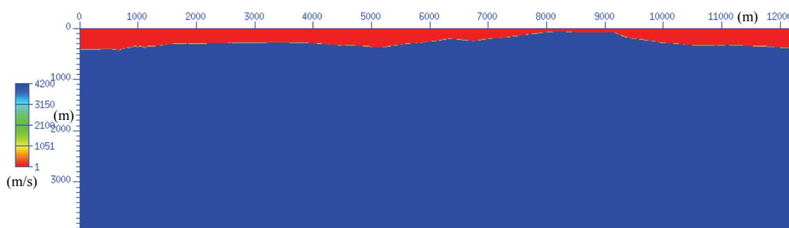
Figure 4.13 A constant velocity/depth model for real data depth migration. There is roughly 500m of elevation relief along the seismic section. The red colour denotes the air with velocity set as 1m/s.
