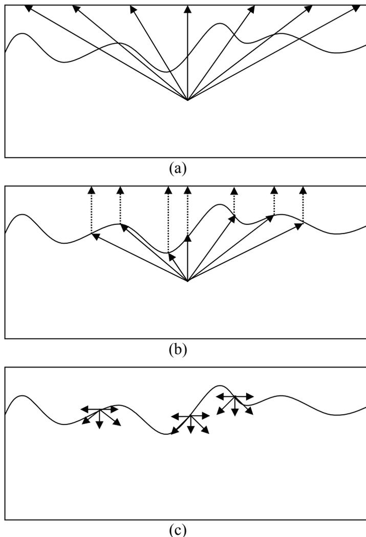
Figure 1.1 Schemes showing raypaths associated with (a) wave-equation datuming, (b) elevation static correction of a wavefield from a recording surface to a higher datum elevation, and (c) the migration from surface topography.
