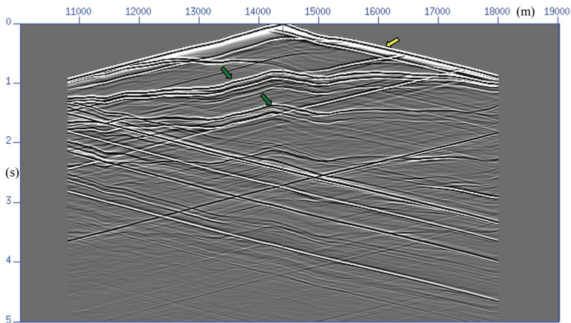
Figure 4.6 A shot gather located approximately at the mid-point of the model (14,500m position). The yellow arrow shows the uneven direct wave energy due to the effect of surface topography, and green arrows indicate reflections from the fault structures.
