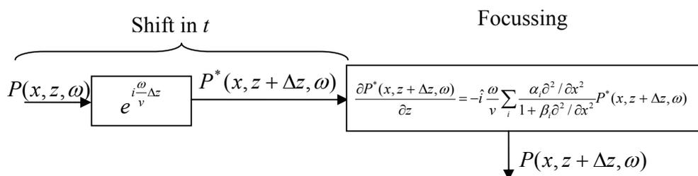
Figure 4.4 The extrapolation scheme for implicit finite-difference.
