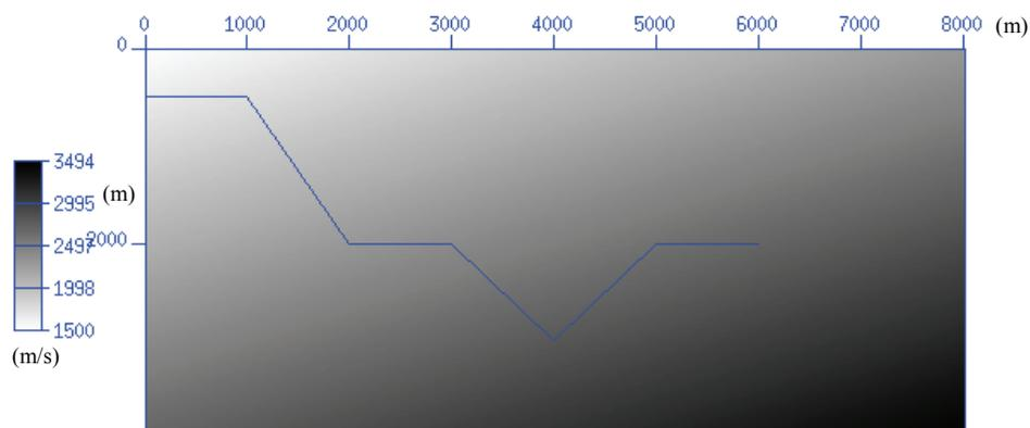
Figure 5.10 Variable velocity model with homogenous Thomsen parameters of  $\varepsilon = 0.2$  and  $\delta = 0.1$ , and a tilt angle  $\phi = 60^\circ$ . P-wave velocities parallel to the symmetry axis vary along the distance and depth as  $v(x, z) = 1,500 + 0.3z + 0.1x$  (m/s).
