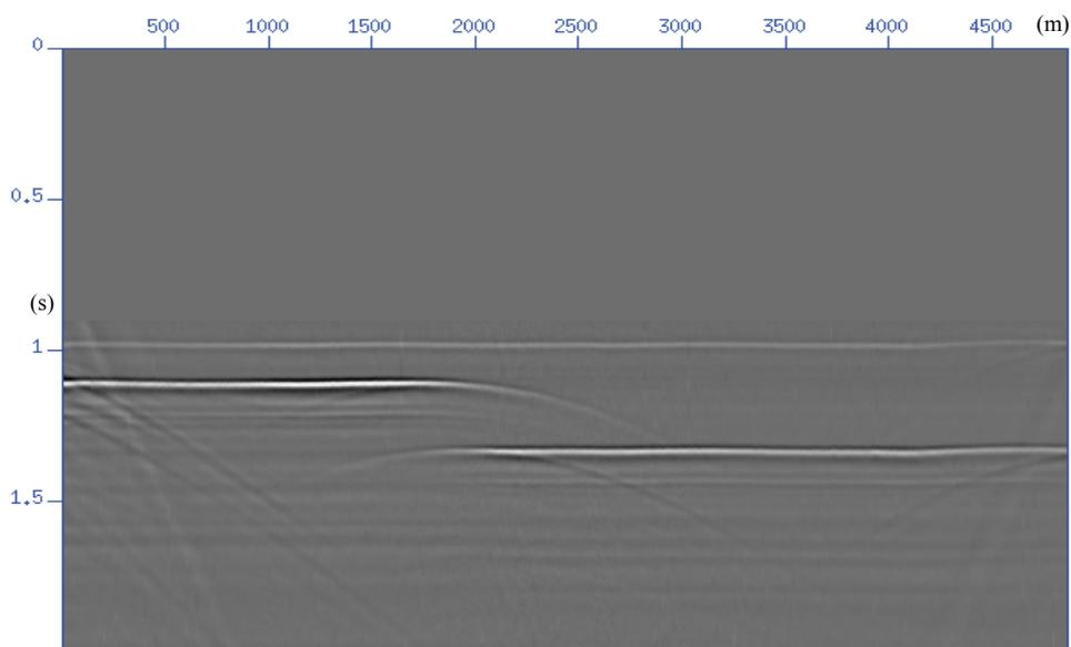
Figure 5.15 Seismic data acquired with coincident source and receiver (the true offset scales to about 200m).
