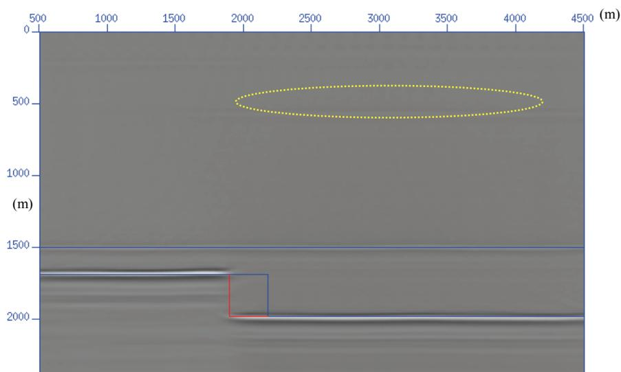
Figure 5.18 Prestack isotropic reverse-time migration result from the reef model. The measured velocity along the vertical direction for the anisotropic overburden and the exact velocity of the isotropic layer are used. The isotropic migration images the reef edge  $\sim 350$  m left of its true position. The blue lines represent the true reef interface while the red lines denote the misplaced migration position.
