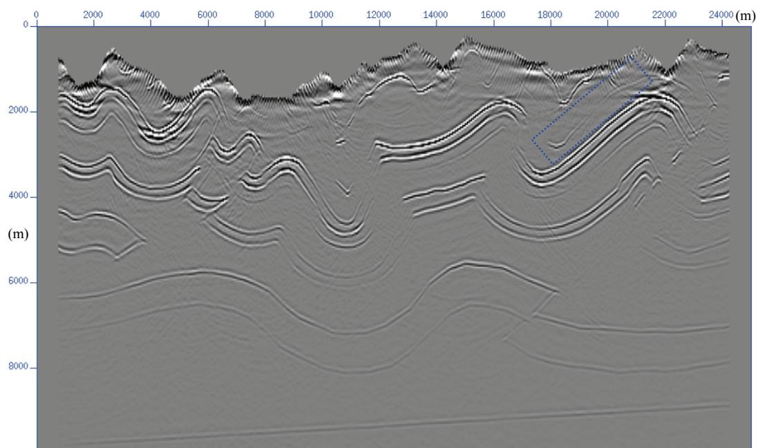
Figure 4.8 Result from the prestack PSPI migration. The blue rotated rectangle denotes the imaging of shallow structures for comparison with the SSF migration below.
