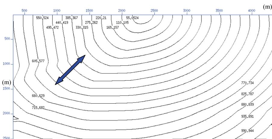
Figure 7.17 The traveltime contours showing the effect of anisotropy when the source position is located at the centre of the model.
