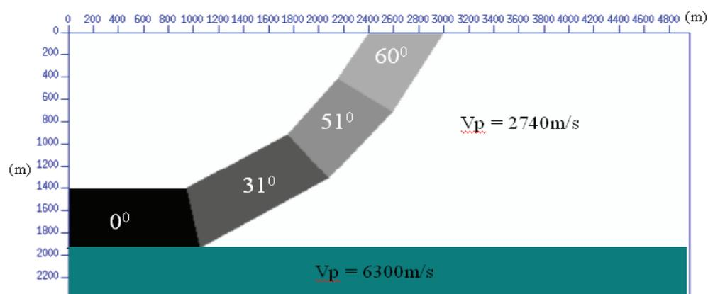
Figure 7.9 Model of an anisotropic thrust sheet embedded in an isotropic background with the same anisotropy parameters and different dipping angles.
