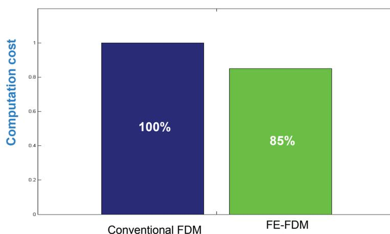
Figure 3.12 The computational efficiency comparison for modelling between FDM and FE-FDM.
