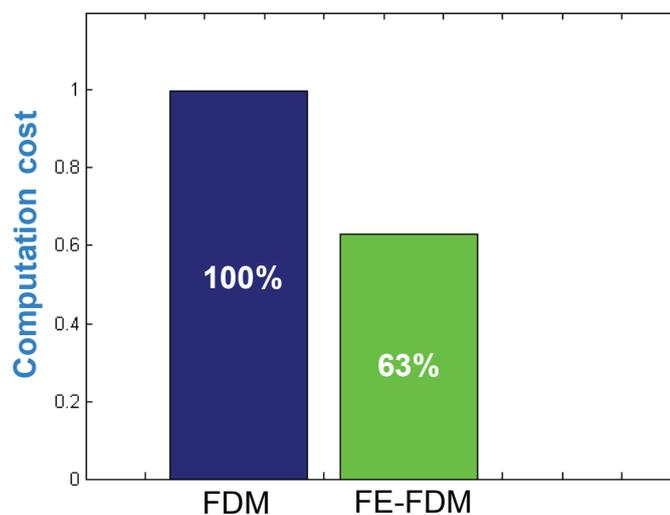
Figure 3.17 The computational efficiency comparison for reverse-time migration between FDM and FE-FDM.
