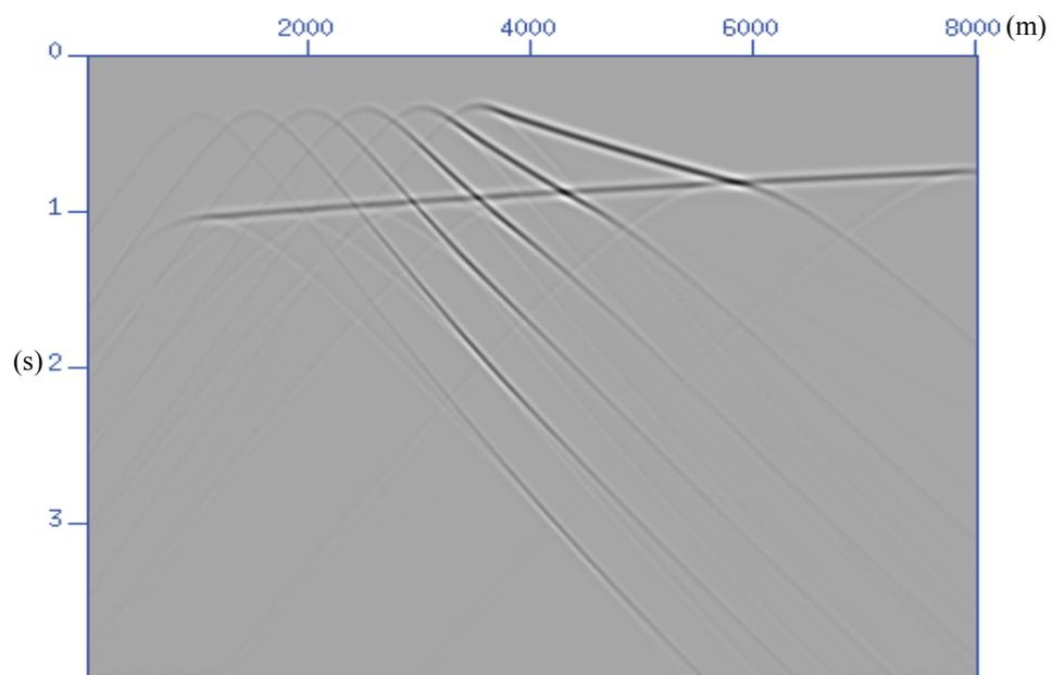
Figure 7.3 The synthetic data for six dipping reflectors in the model shown in Figure 7.2.
