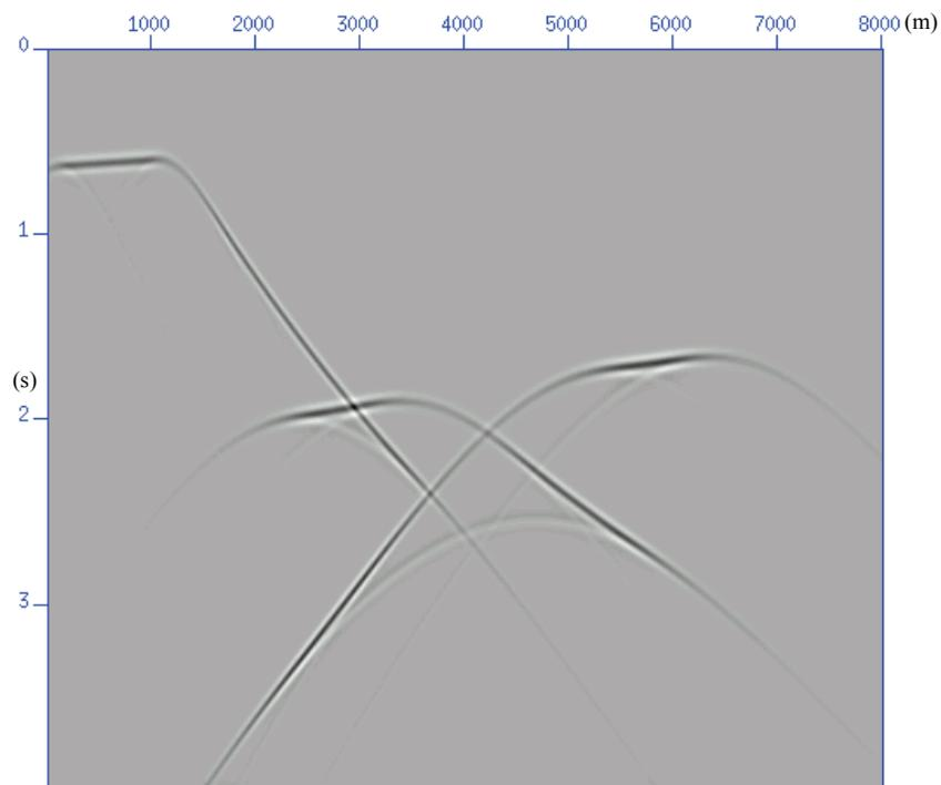
Figure 5.11 Synthetic zero-offset seismogram obtained using SU code from the Center for Wave Phenomena (CWP) for the structural model shown in Figure 5.10 of a tilted TI medium.
