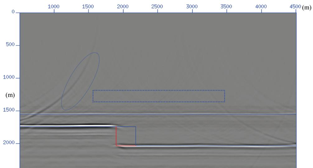
Figure 6.11 Post-stack isotropic PSPI migration result from the reef model.
