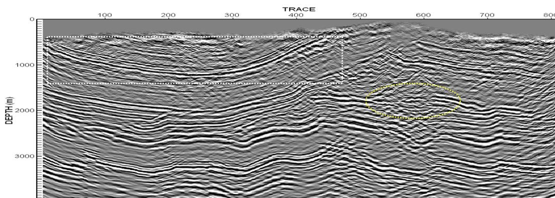
Figure 4.14 The result of prestack Kirchhoff depth migration with a constant velocity of 4,200m/s from surface topography. The dashed white rectangle and yellow ellipse shows the poor imaging quality when compared with the result from the prestack SSF method.
