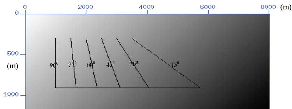
Figure 7.2 A variable velocity model with homogenous anisotropy parameters that consist of six dipping reflectors.
