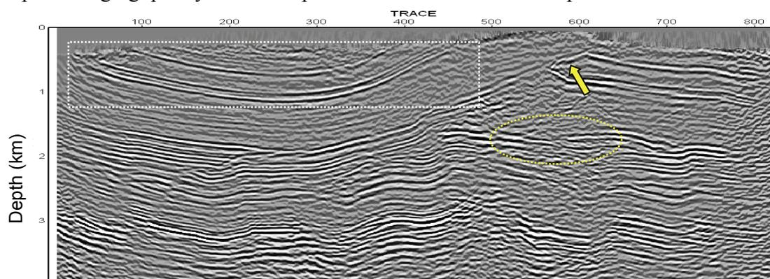
Figure 4.15 The result of prestack SSF depth migration with a constant velocity of 4,200m/s from surface topography. The dashed white rectangle and yellow ellipse shows the better imaging quality compared with the result from the prestack Kirchhoff depth method. The yellow arrow shows the structure unnoticeable in the Kirchhoff result.
