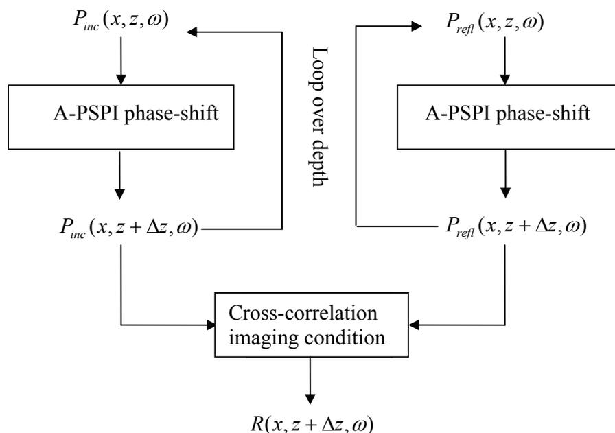
Figure 6.3 The procedure for prestack anisotropic PSPI.
