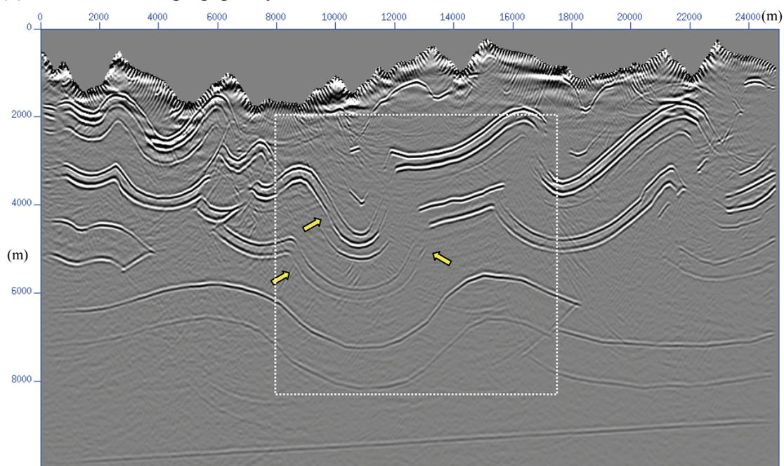
Figure 4.11 Result from the prestack implicit finite-difference migration. The white dashed rectangle delineates good fold structure imaging. The yellow arrows indicate more consistent fold structure imaging.
