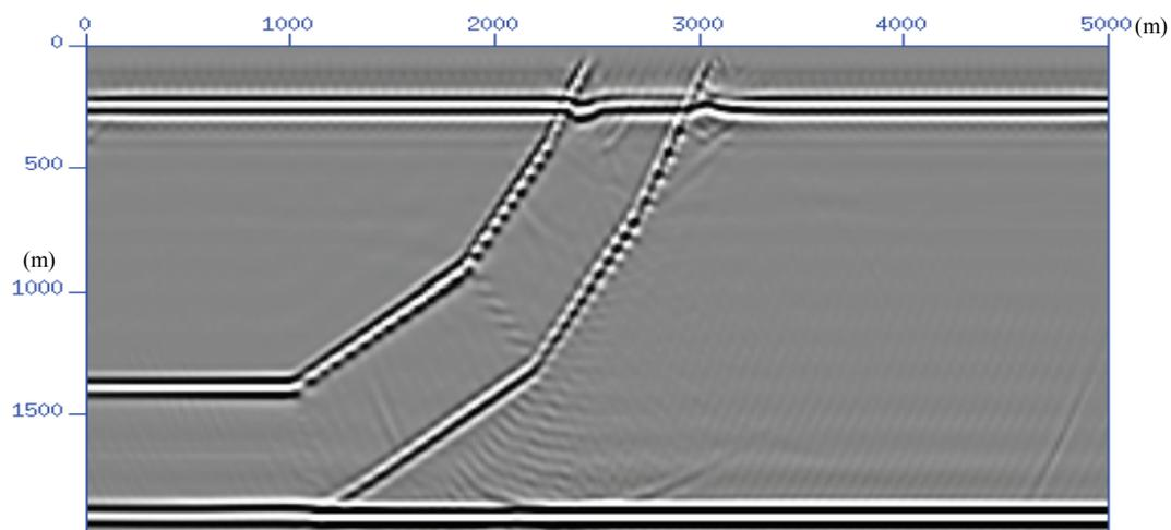
Figure 7.26 The prestack anisotropic PSPI migration result with correct velocity and anisotropy parameters.
