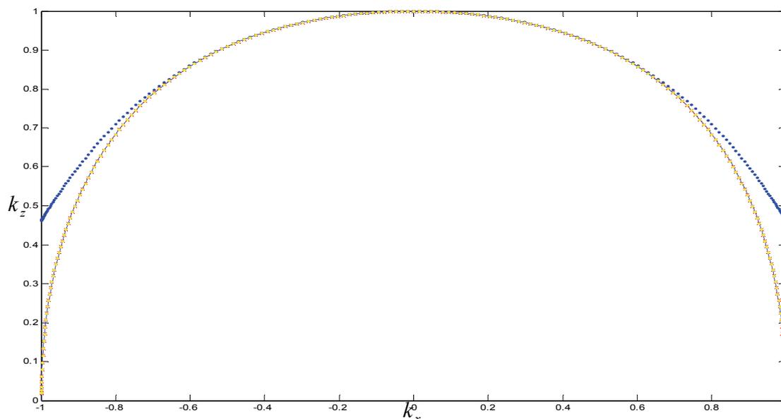
Figure 8.6 Dispersion relationship for anisotropy parameters  $\varepsilon = 0$ ,  $\delta = -0.2$ : blue solid line is the true dispersion relationship; blue dashed point is the approximation dispersion by Taylor-series analysis; line of red crosses is the approximation dispersion by the 4<sup>th</sup> order accuracy optimization; yellow dot that closely matches with red crosses is the approximation dispersion by the 6<sup>th</sup> order accuracy optimization.
