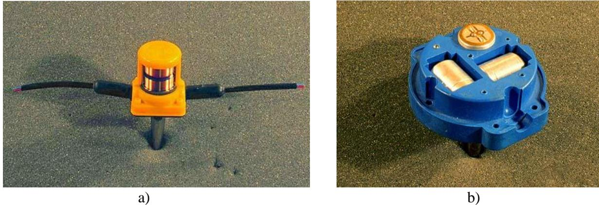
**Figure 2.3: Geophones used in seismic acquisition, a) single component geophone, and b) three component geophone. Taken from <http://www.crewes.org/ResearchLinks/ConvertedWave/page2.php>**
