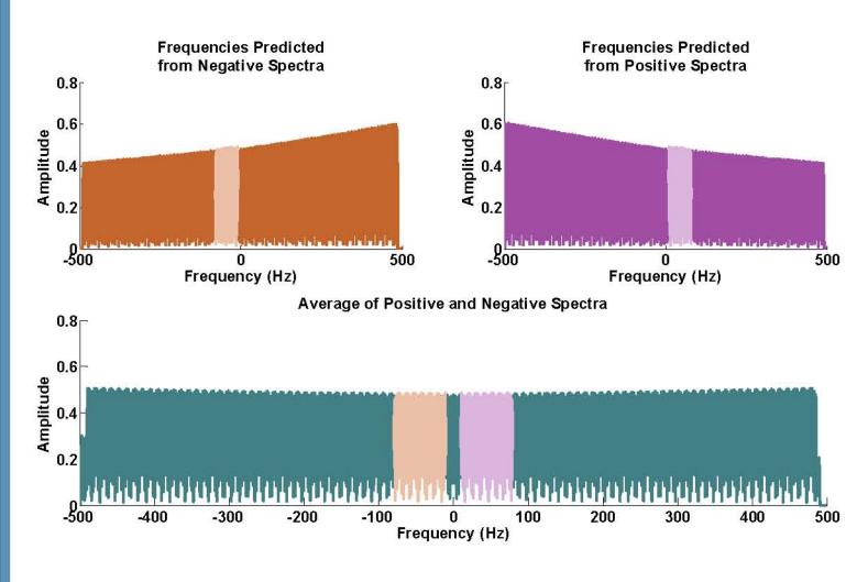
A band of frequencies is selected that has a flat spectrum. The prediction filters take this band of positive frequencies indicated in pink and predict frequency samples in the forward and backward direction. This is repeated with he negative band of frequencies. These results are then averaged to create the predicted spectrum indicated by teal in the figure to the left.
