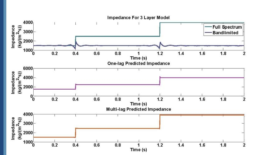
Fourier inverse transform is applied to the predicted frequency spectrum, we get the full band reflectivity in time. The recursion formula can then be used to invert for impedance, which the results are seen for the 3 layer model. Both methods were within 2% of the model impedance.
