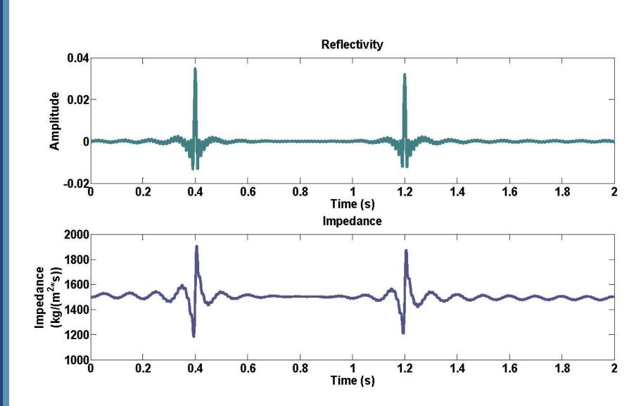
when time impedance is calculated bandlimited the reflectivity, the impedance curve has no trend to it only shows the location of the changes not the magnitude of them. illustrates importance of the Lowfrequencies.
