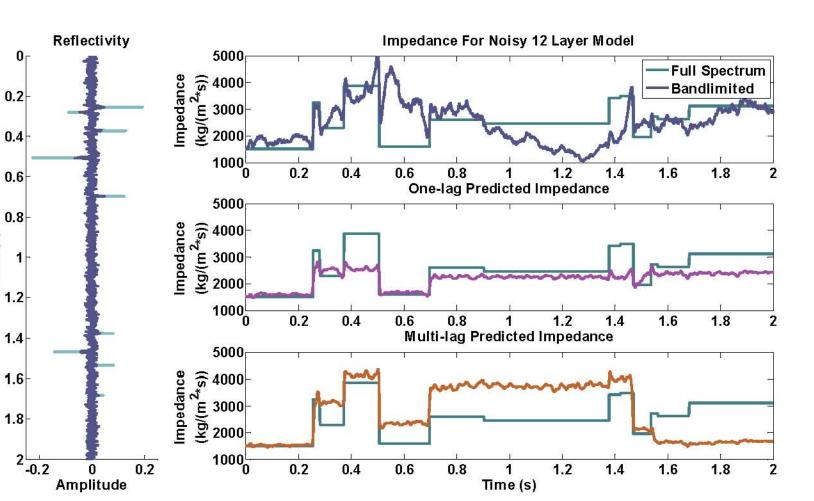
Noise was added to the twelve layer model and the results to the left were obtained. From these results it may seem that the multi-lag performs better on a noisy case but vigorous testing has showed that the inversion is sensitive to the amount of noise that is present. High signal to noise ratios produce the best results
