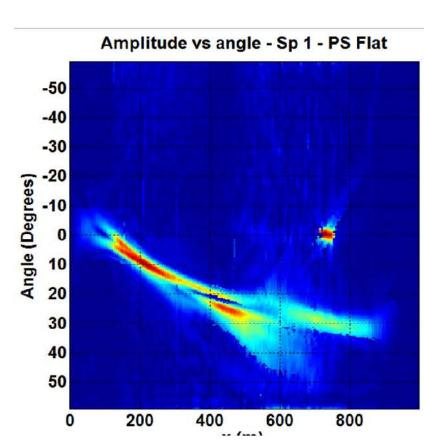
Amplitude as a function of the angle for all locations in the line. The source in shot 1. (a) PP wave. (b) PS wave. Notice the differences on the energy distribution and the smaller angles for PS.
