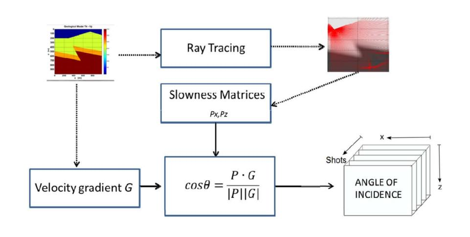
Ray tracing method scheme to obtain the angles of incidence from the velocity field.
