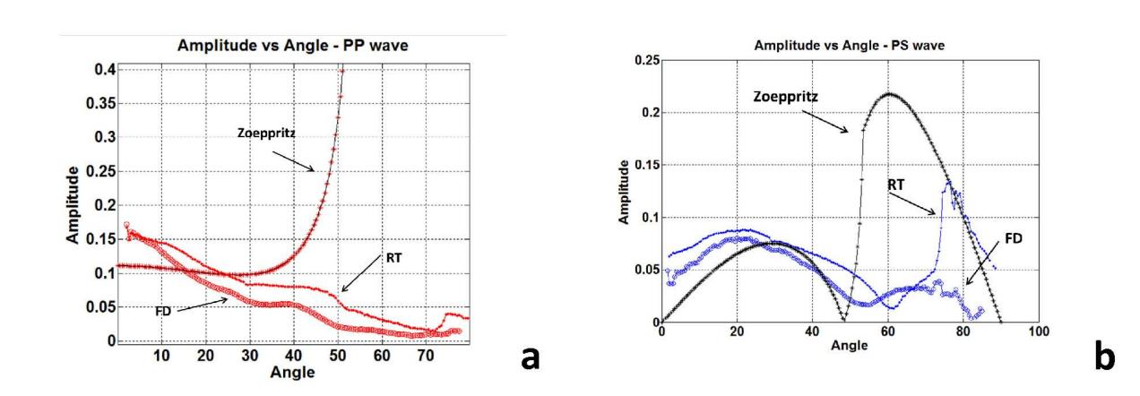
Amplitude vs. Angle of Incidence (a): PP, (b) PS RT: migration of ray tracing data. FD: migration of Finite Difference data, and the theoretical Zoeppritz calculation.
