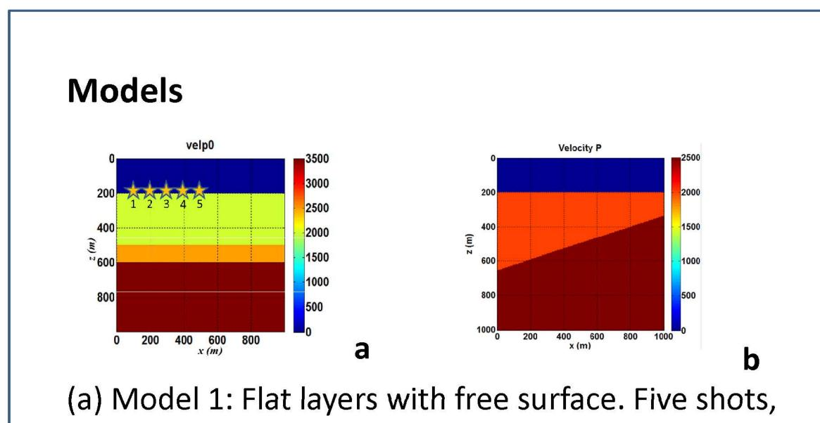
identified with stars, are located on the surface.(b) Model 2: dipping interface. The same shot distribution was used for both.
