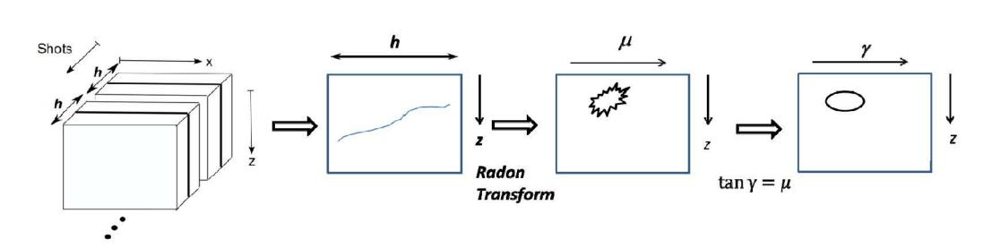
Extended imaging angle gather technique: It was applied the Radon Transform in the h-z (offset-depth) domain.
