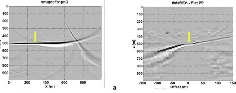
(a) The conventional migration section and (b) the extended image. The point shown by the arrows is the same one in both (offset zero and same x).
