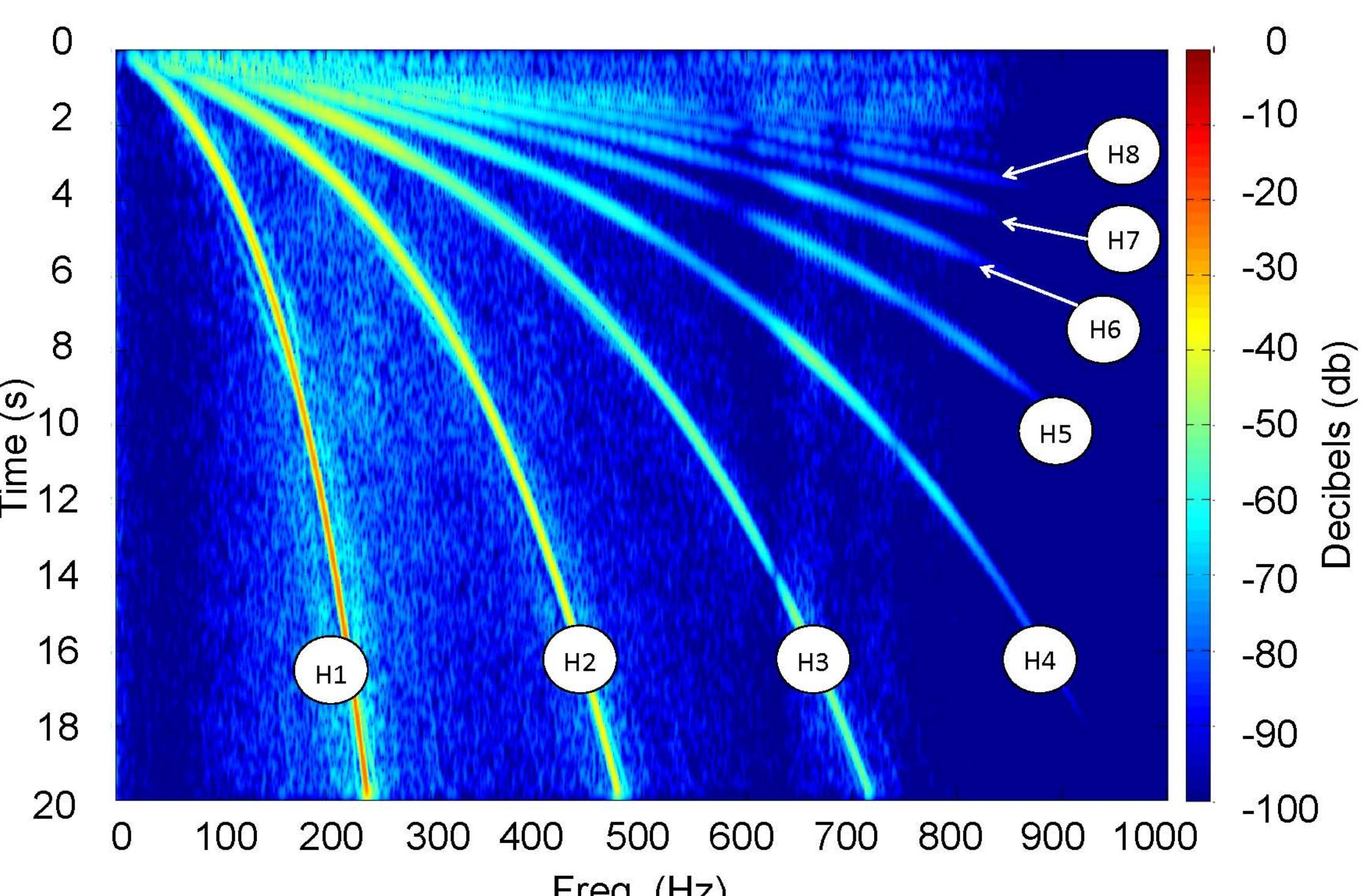
Figure 1. The Gabor spectrum of a typical high signal to noise ratio sweep from field data provide by StatOil.
