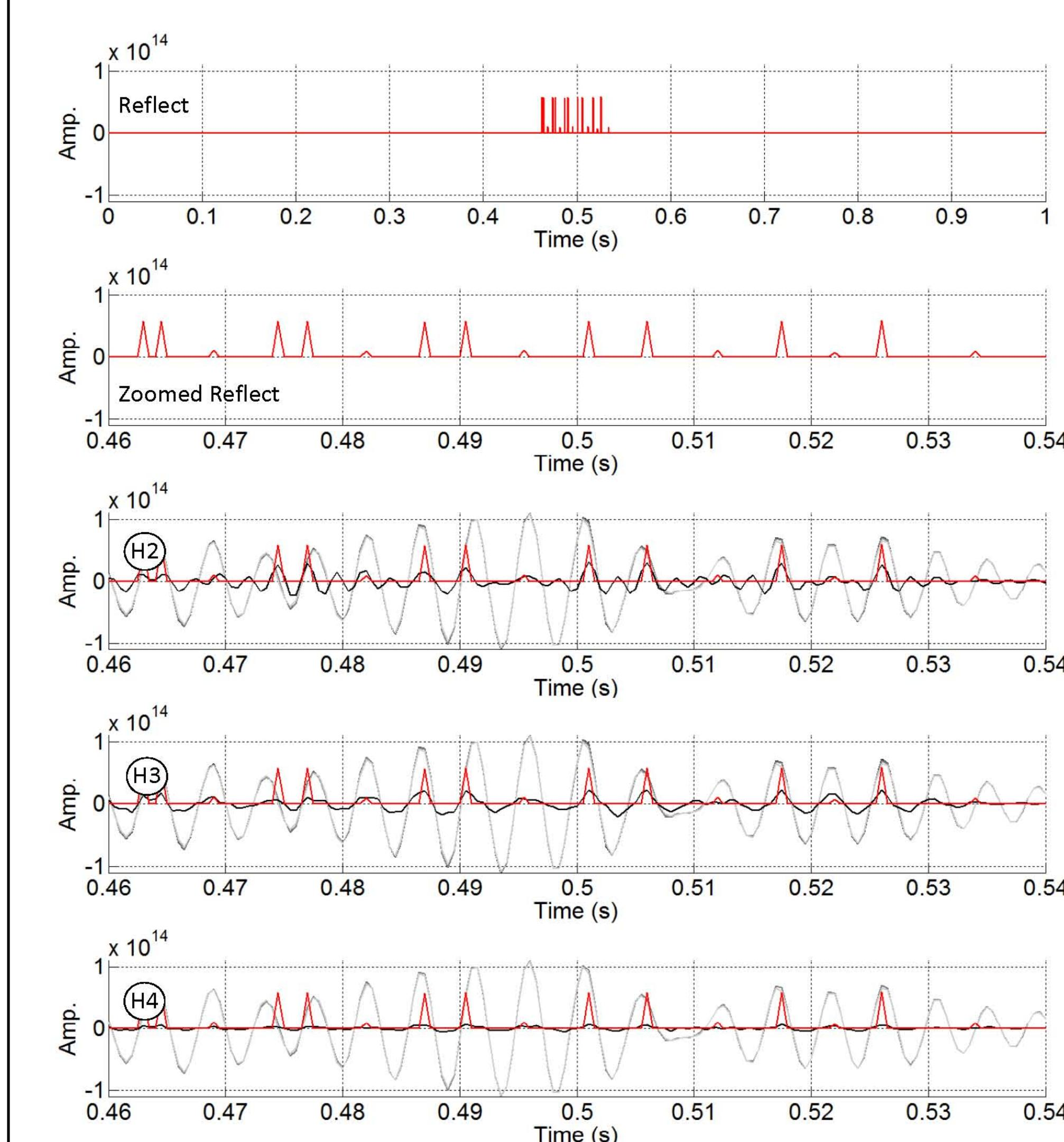
Figure 4. Synthetic trace correlated with H2, H3 and H4 to reveal to investigate better resolving power of harmonics.
