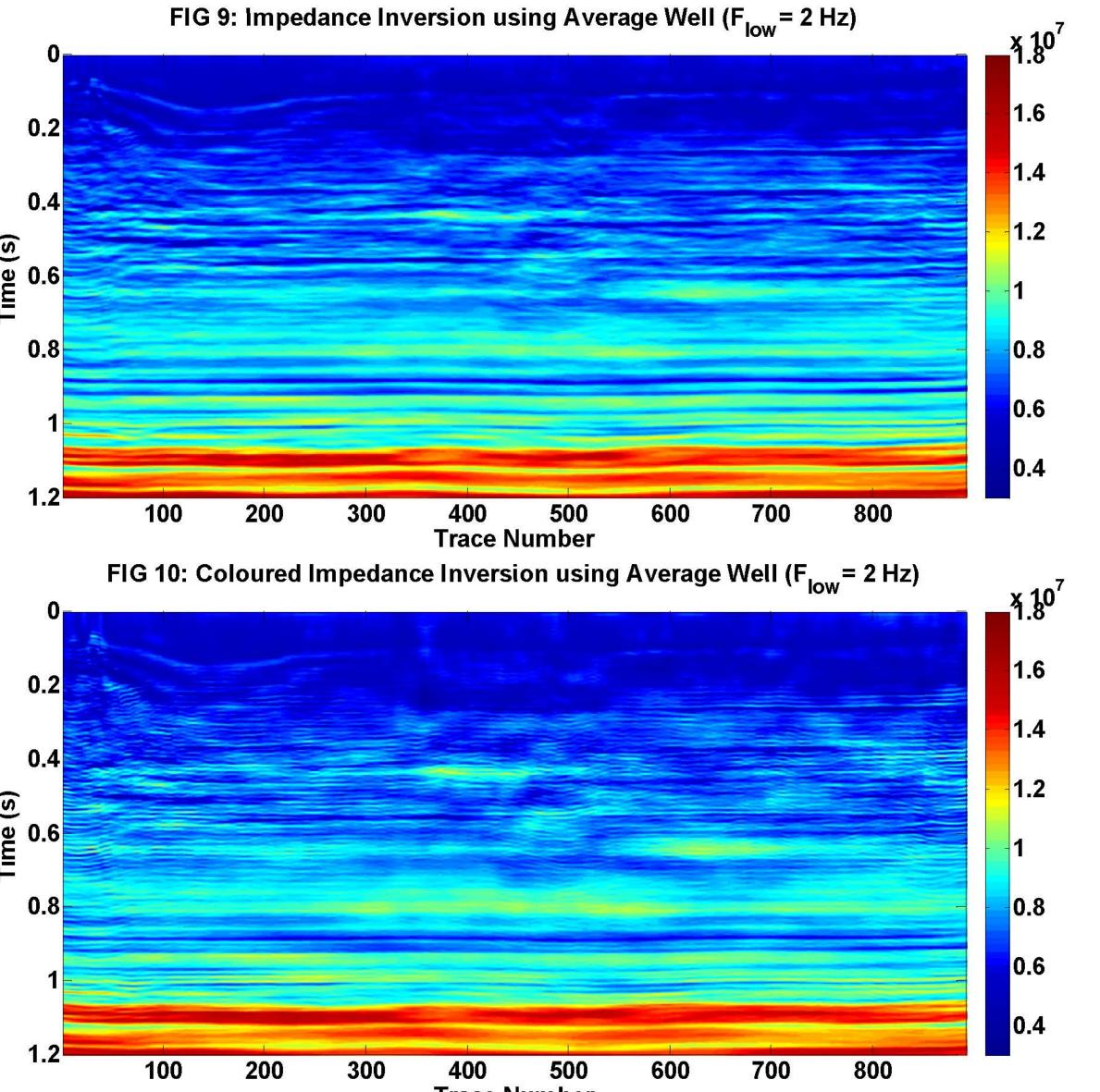
The BLIMP algorithm (Ferguson and Margrave, 1996) was used with a low-frequency cut-off of 2 Hz to compute the inversion in Figure 9 and the coloured inversion in Figure 10. The coloured inversion definitely contains more high frequencies although they do appear to be mostly noise.
