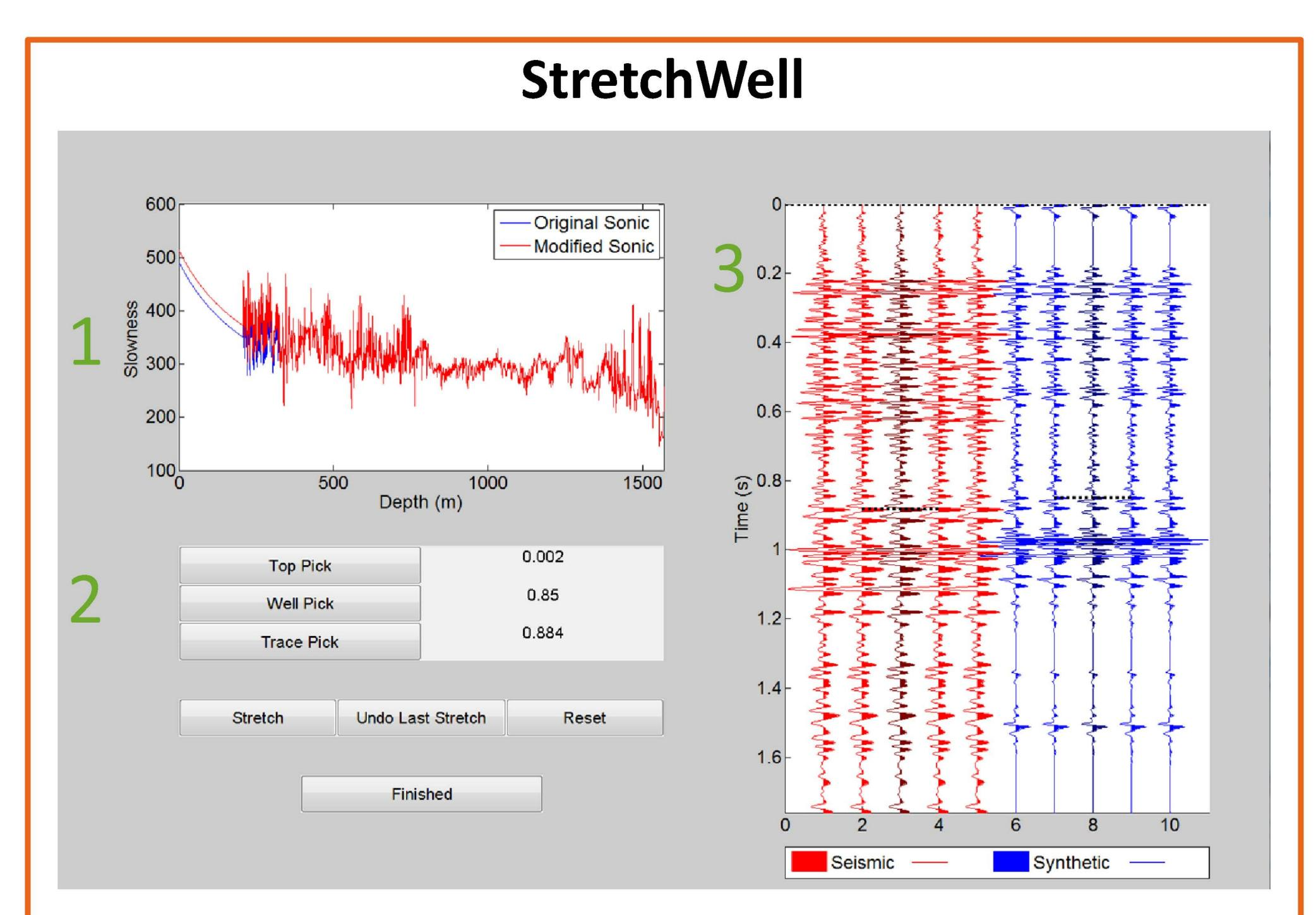
StretchWell modifies the sonic log allowing the synthetic to match the seismic in time.
