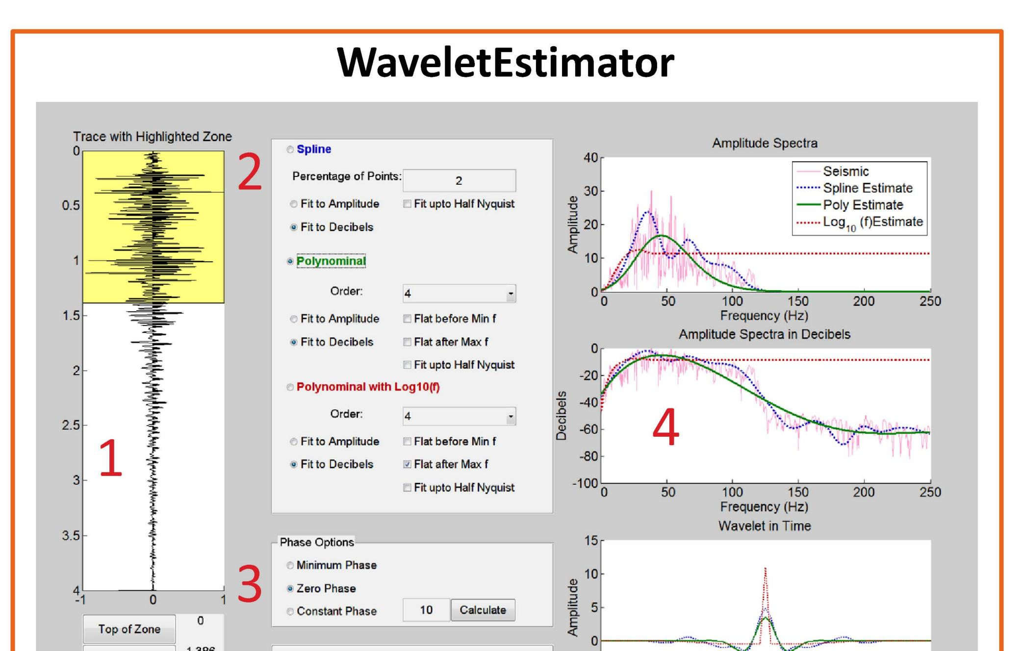
WaveletEstimator allows the user to design a wavelet using the amplitude spectra of a trace, well log or other data.
