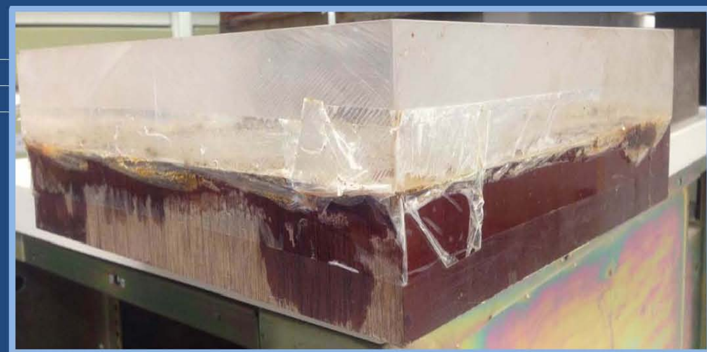
FIG. 1. A physical model consisting of a Phenolic layer under a Plexiglas layer, and representing a fractured reservoir overlaid by isotropic overburden. Laboratory to field scale is 1:10,000 in both length and time. Scaled thicknesses of Plexiglas and Phenolic layers are 480 m and 450 m respectively.
