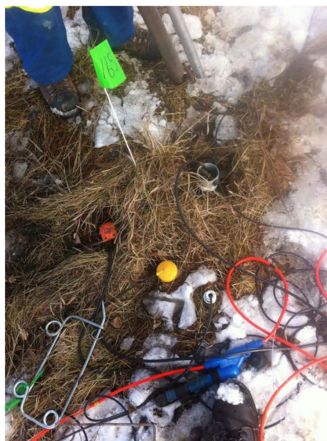
Figure 2: The sensors under test at station 165. The top of the ground screw appears slightly above and right of center. The comparable 3-component SM7 surface geophone is to the left in the orange case.
