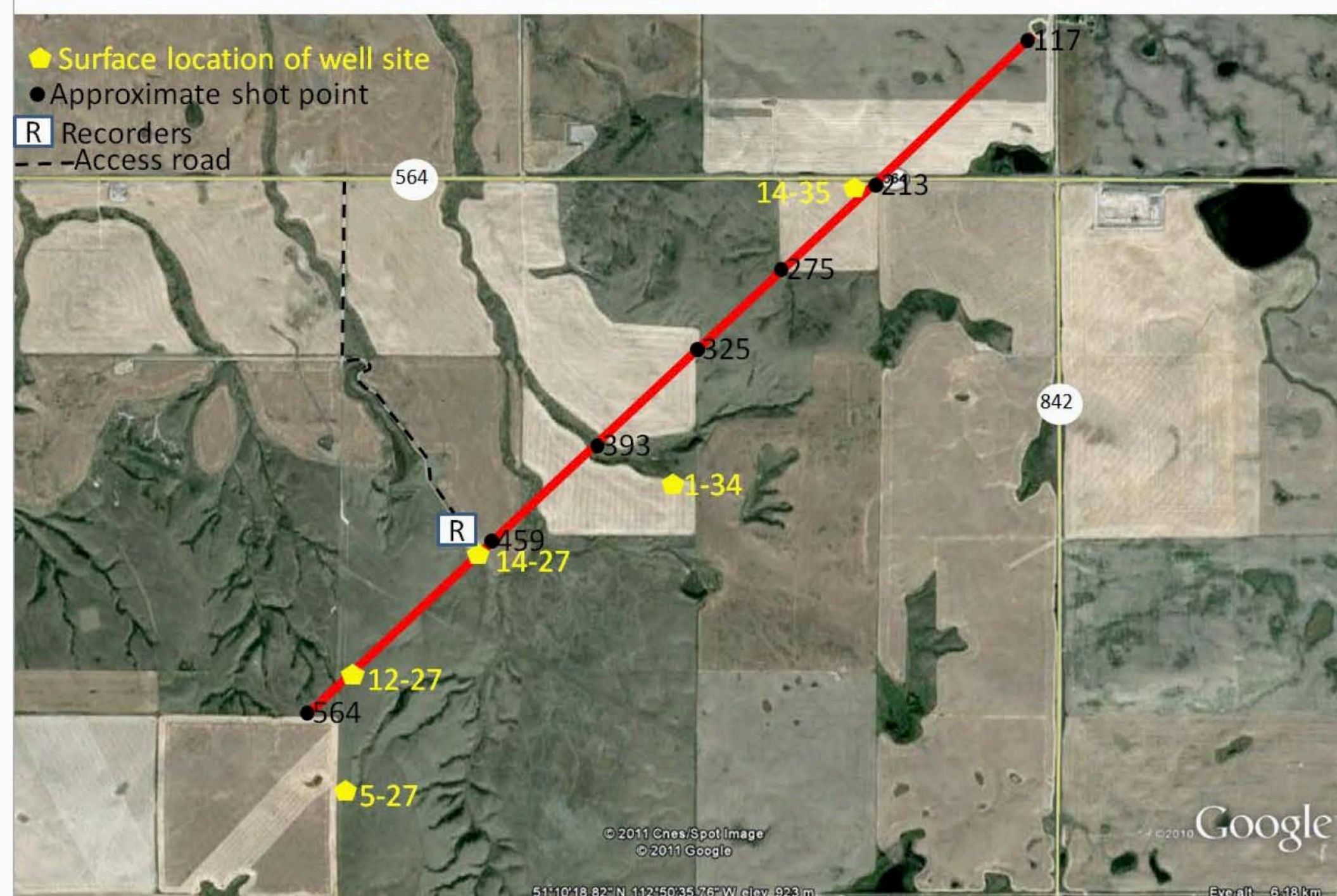
Figure 1. The 4.5 km Hussar seismic line is shown together with the locations of 5 wells with good logging suites, shot point locations, and the location of the recorders.
