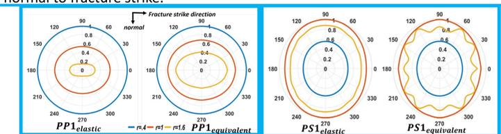
(5). Azimuthal polar plot of PP amplitude azimuthal anisotropy for elastic (left) and equivalent modeling (right), and PS amplitude azimuthal anisotropy from top of HTI layer
