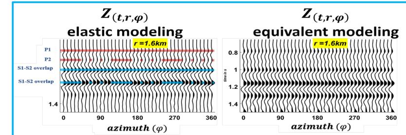
Fig 4a: Z-component azimuthal scans at source-receiver constant offset of 1.6km. The yellow labels are the azimuthal values in degree.
