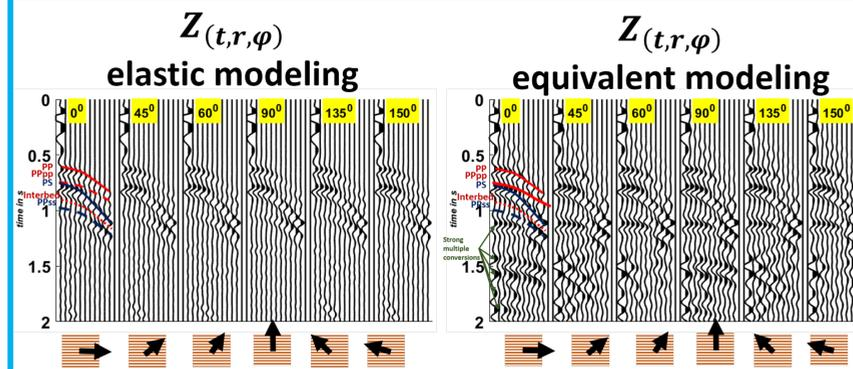
Fig 2a: Z component-radial scans at various fixed azimuths. The yellow labels are the azimuthal values in degree.
