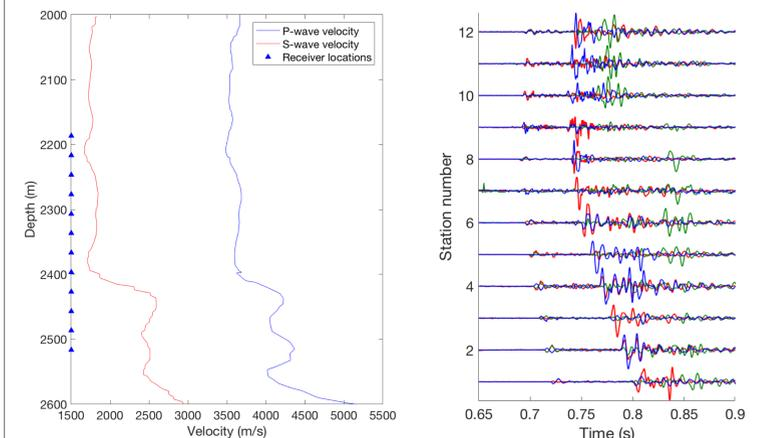
**Figure 4:** (a) Velocity model and receiver depths, (b) a  $M_W -1.3$  event 346 m away from the receiver well.
