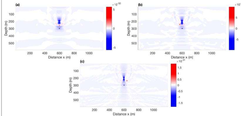
**Figure 1:** Source-term gradient as a function of frequency: (a) 30 Hz, (b) 60 Hz, (c) 120 Hz.
