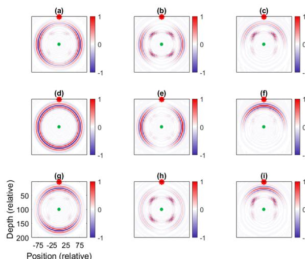
Figure: Fibre scattering radiation patterns for  $v_p$  (column 1),  $v_s$  (column 2), and  $\rho$  (column 3) for 70.5 degree (a)-(c), 35.2 degree (d)-(f), and 10 degree (g)-(i) helical fibres.
