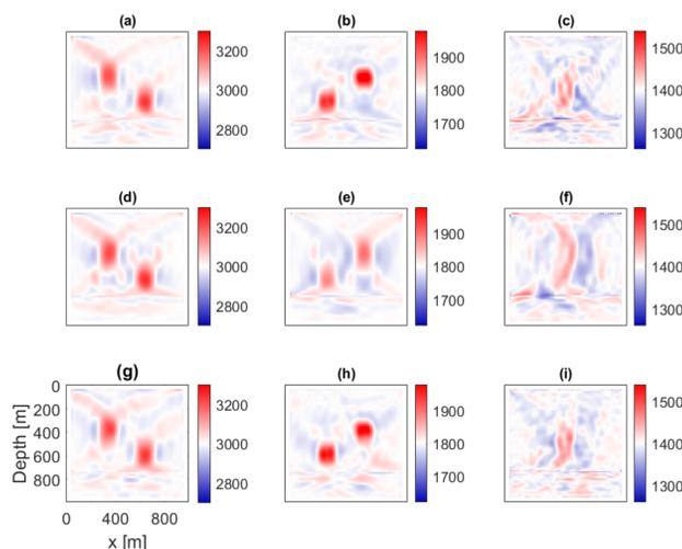
Figure: Inversion results from a toy model for  $v_p$  (column 1),  $v_s$  (column 2), and  $\rho$  (column 3) for 70.5 degree (a)-(c), 35.2 degree (d)-(f), and 10 degree (g)-(i) helical fibres.
