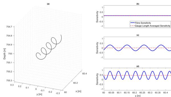
Figure: Helical fibre (a), and its sensitivity to  $\epsilon_{xx}$  (b),  $\epsilon_{xz}$  (c), and  $\epsilon_{zz}$  (d).
