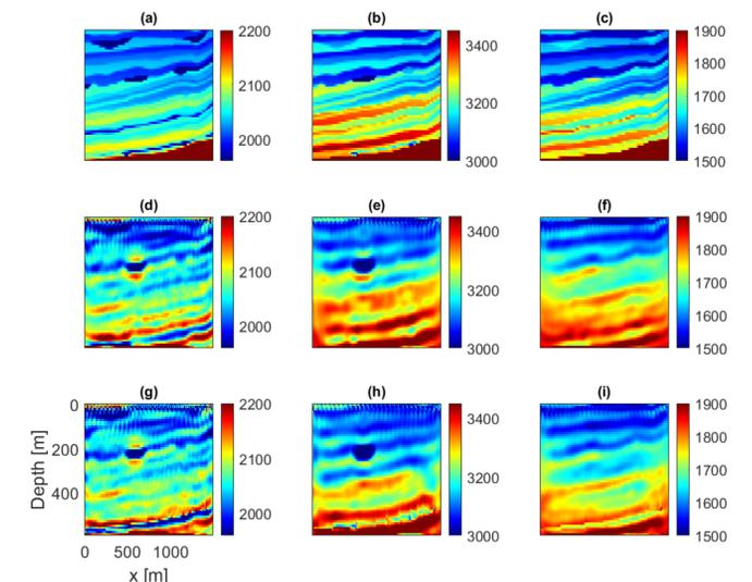
Figure: True models from a portion of the Marmousi2 model for  $\rho$ ,  $v_p$  and  $v_s$  in (a)-(c), inversion results using only geophones  $\rho$ ,  $v_p$  and  $v_s$  in (d)-(f), and inversion results using a fibre in a horizontal well and surface geophones for  $\rho$ ,  $v_p$  and  $v_s$  in (g)-(i).
