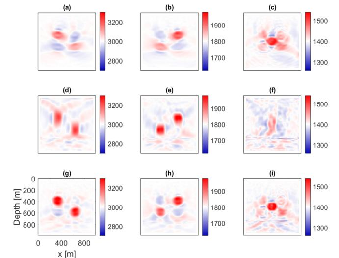
Figure: Inversion results from a toy model for  $v_p$  (column 1),  $v_s$  (column 2), and  $\rho$  (column 3) for reflection geophone data (a)-(c), strain data from a 10 degree helical fibre in a horizontal well (d)-(f), simultaneous inversion of reflection geophone data and strain data from a 10 degree helical fibre in a horizontal well (g)-(i).
