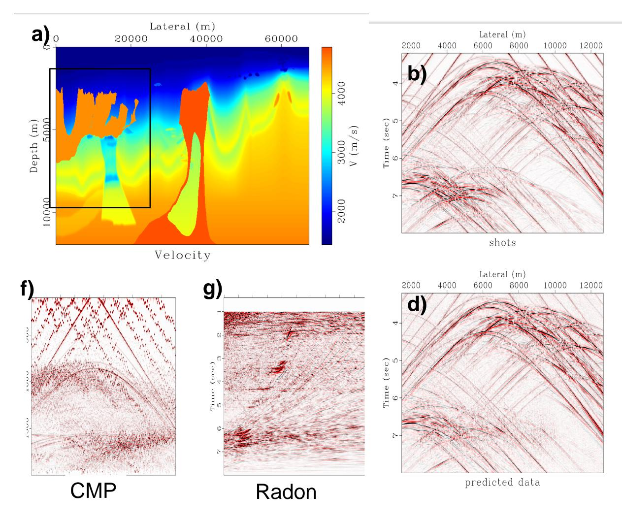
Example of deblending by inversion in a difficult data set. Although a hyperbolic Radon transform was used for all these examples, a more flexible transform may be necessary in complex cases. a) velocity, b) 5x supershot (blended), c) never-blended shot d) result of data fitting e) deblended shot, f) A pseudo-deblended CMP, g) Radon transform subpanel of f).
