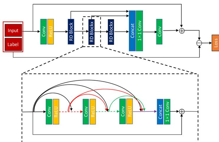
Figure 1: The architecture of the RdNet (modified from Zhang et al., 2018).
