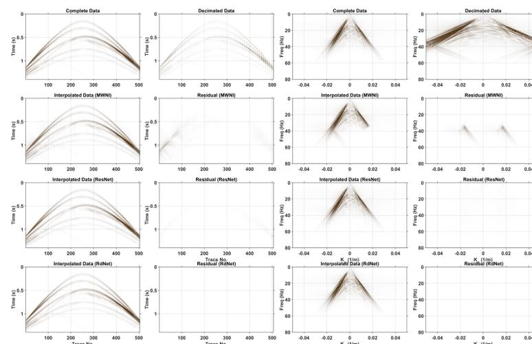
Figure 3: Interpolation results (for validation shot #12) with 1/3 of original trace interval. S/Ns for the reconstructed shot gathers are 14.7, 27.7 and 37.5 dB, respectively.
