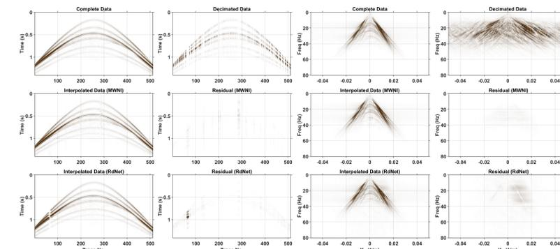
Figure 4: Interpolation results of validation shot #22 for the case of 50% missing traces. S/Ns for the reconstructed shot gather are 24.3 and 13.9, respectively.
