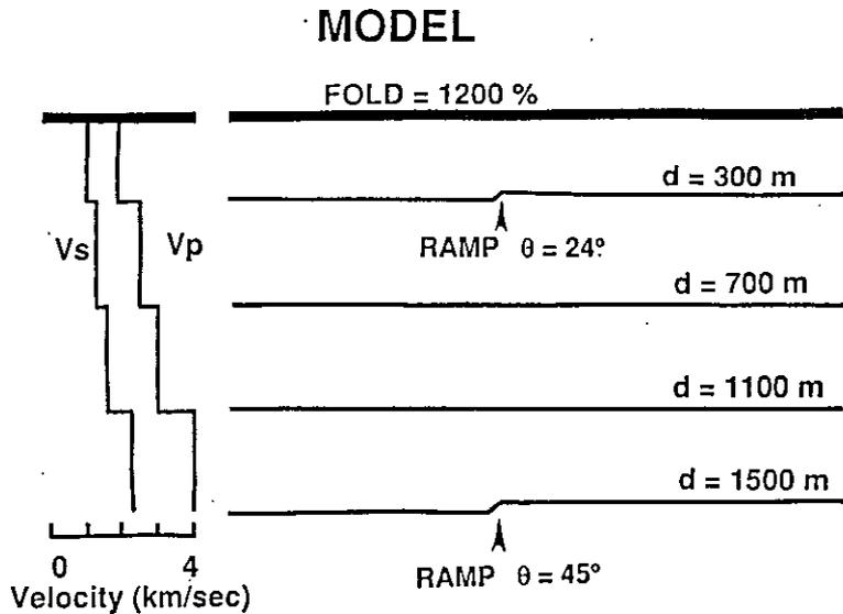
Fig. 6. Velocity model used to generate raytraced synthetic data.
