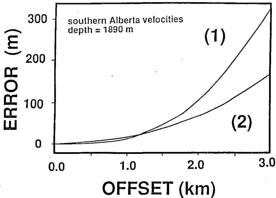
Fig. 4. Location error with offset of approximating formulae. Curve 1 is error incurred by using asymptote formula (equation 3). Curve 2 is error incurred by using algorithm of Tessmer et al.(1988) focussed for depth of 1890 metres. Error is defined as absolute difference in metres of location given by formulae and raytraced location.
