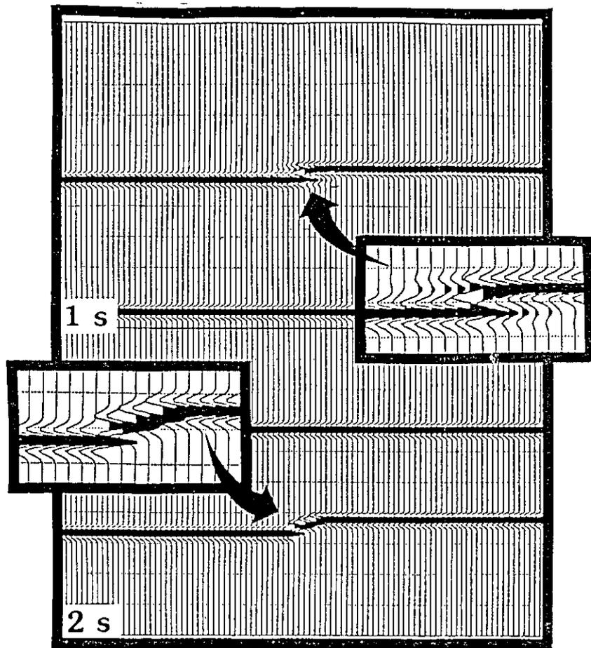
Fig. 7a. Results of stacking the model data gathered using the asymptote formula (equation 3). Note the smearing of the shallow event.
