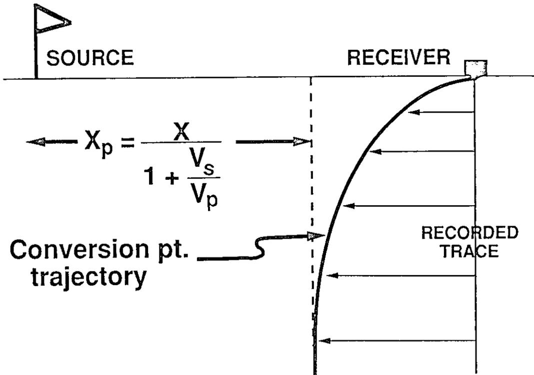
Fig. 5b. Schematic diagram illustrating depth-variant mapping. Each sample point of the moveout-corrected trace is mapped to its appropriate offset location.
