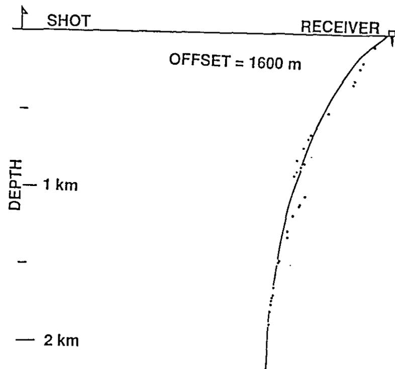
Fig. 2b. Offset locations of mode-conversion points determined by raytracing through southern Alberta velocity profile shown in Fig. 2a.
