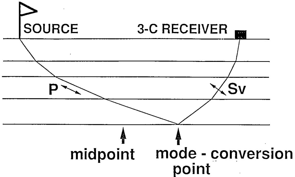
Fig. 1a. The raypath geometry of converted-wave data is nonsymmetrical in a flat and isotropic earth.
