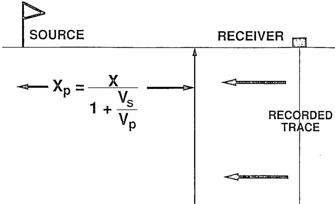
Fig. 5a. Schematic diagram showing gathering of converted-wave data in procedure analogous to compressional-wave gathering except some value (eg. asymptote value of conversion-point trajectory shown in Fig. 1b) is used in place of the midpoint.
