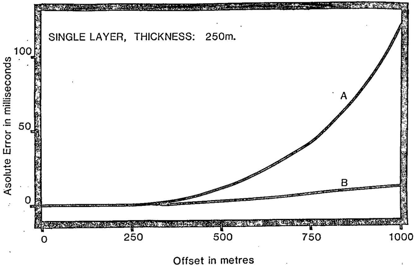
Fig. 3. Absolute error in milliseconds incurred by using equations (1) (Curve A) and (2) (Curve B) to moveout correct converted wave data from a single isotropic layer of thickness 250 metres. True travelttime was computed using raytracing.
