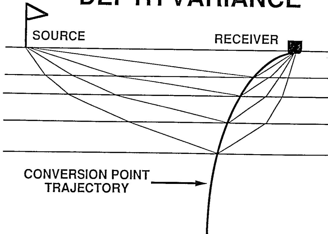
Fig. 1b. The offset locations of the mode-conversion points vary with depth.
