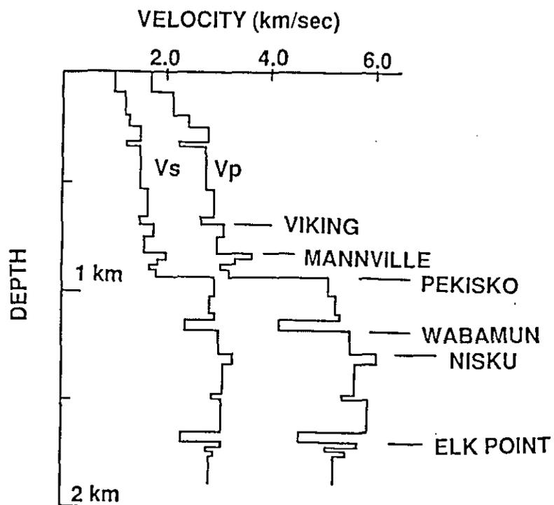
Fig. 2a. Southern Alberta velocity profile. Based on VSP measurements (after Geis et al., 1989)
