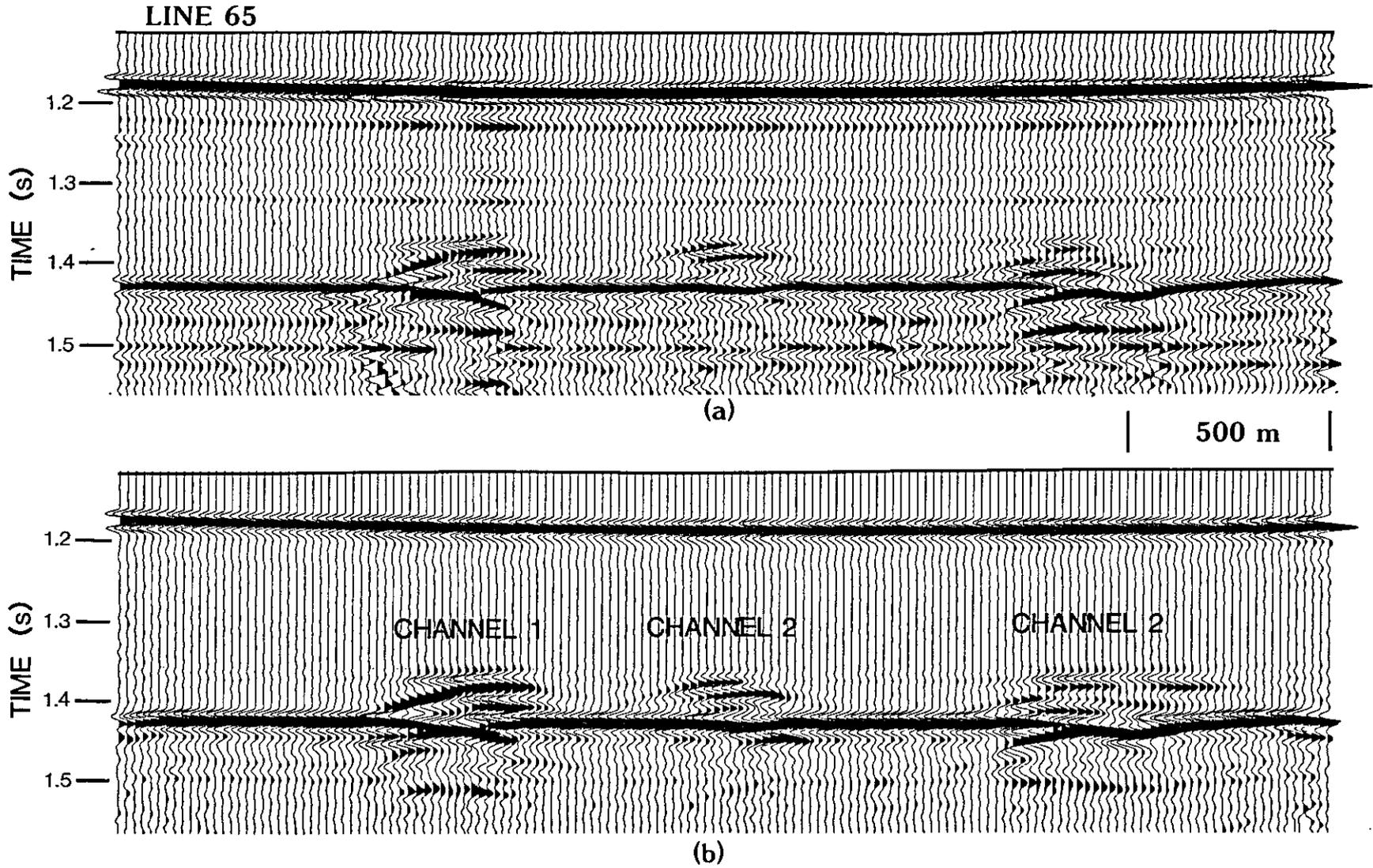
FIG. 4. Comparison between unmigrated (a) single-fold and (b) 15-fold seismic sections from Line 65 of the channel model.
