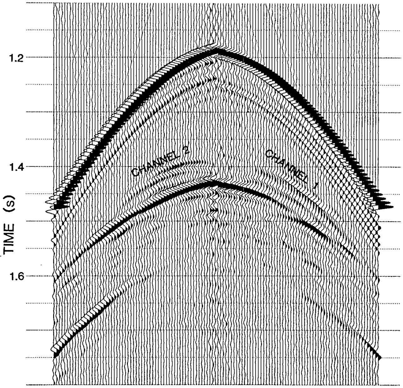
FIG. 2. Example of a shot gather from line 65, showing channel events.
