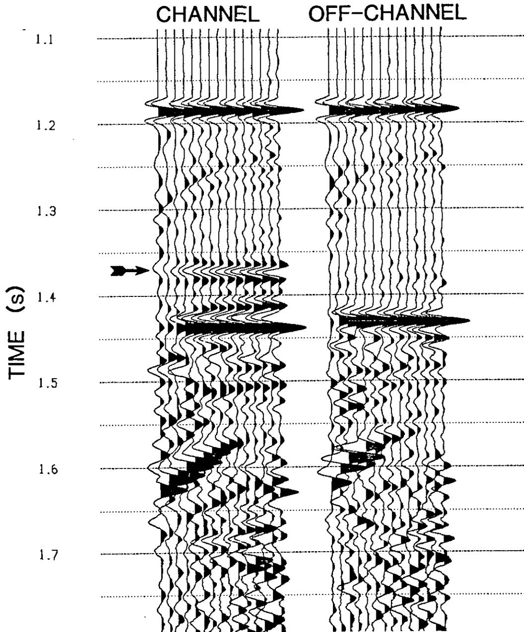
FIG. 3. NMO-corrected CDP gathers from on-channel and off-channel locations. The arrow marks the top of channel reflection. Note the significant amplitude of mode-converted energy at about 1.6 seconds.
