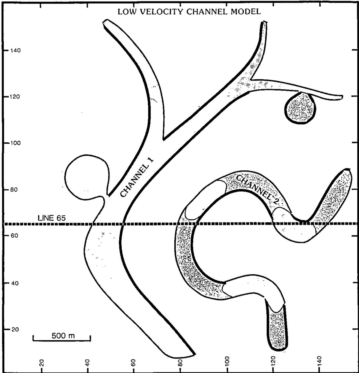
FIG. 1. Plan view of the channel model. The dot pattern shows thick channels and the stipple pattern shows thin channels.
