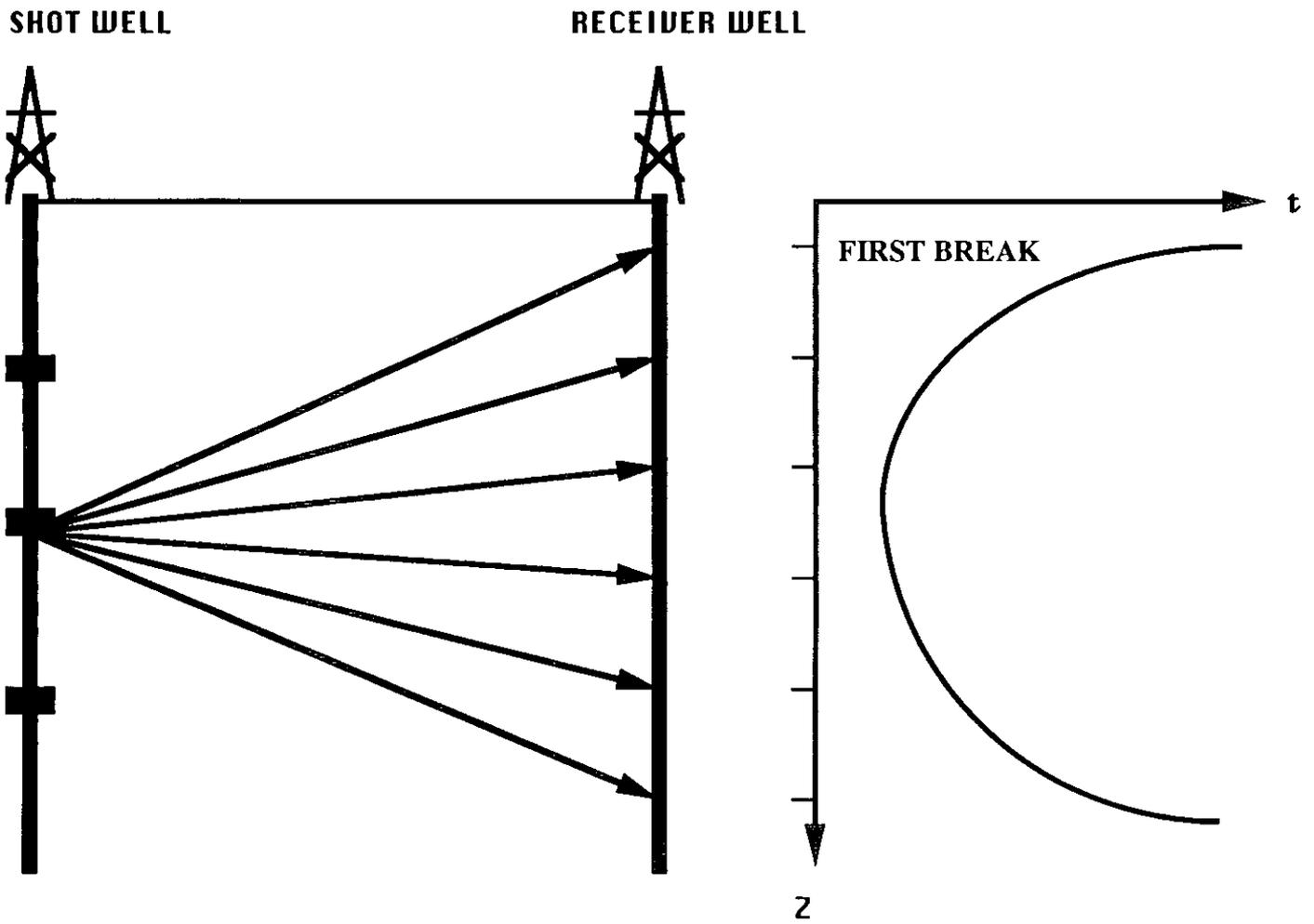
Fig. 1 The raypaths of the direct arrivals and their traveltime recorded in a typical crosswell seismic survey.
