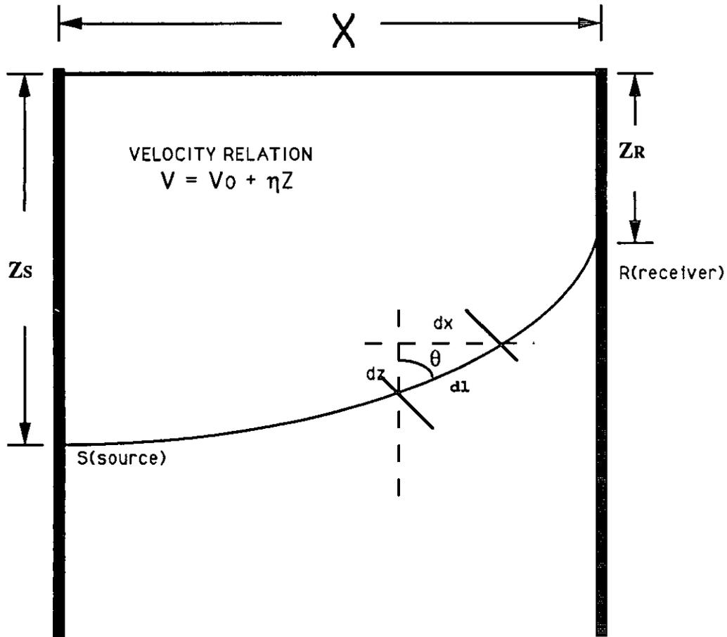
Fig. 2 Ray path of a seismic wave traveling from the source to the receiver.
