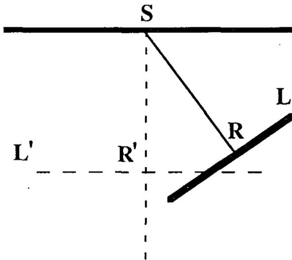
Fig. 1. The seismic profile is out of the plane of viewing
