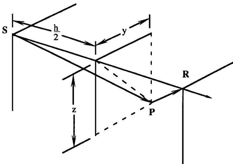
Fig. 7. Geometry of a point scatterer
