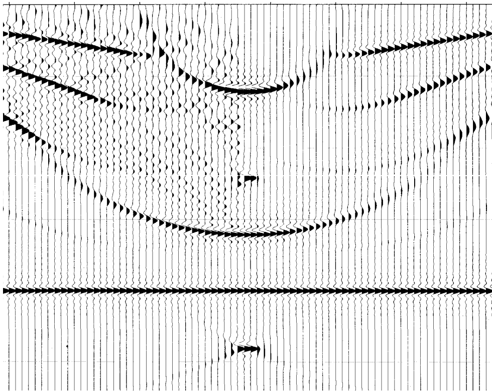
Fig. 9. A Kirchoff migration on a synthetic model with the an anti-aliasing filter applied to right side, while the left side id aliased.
