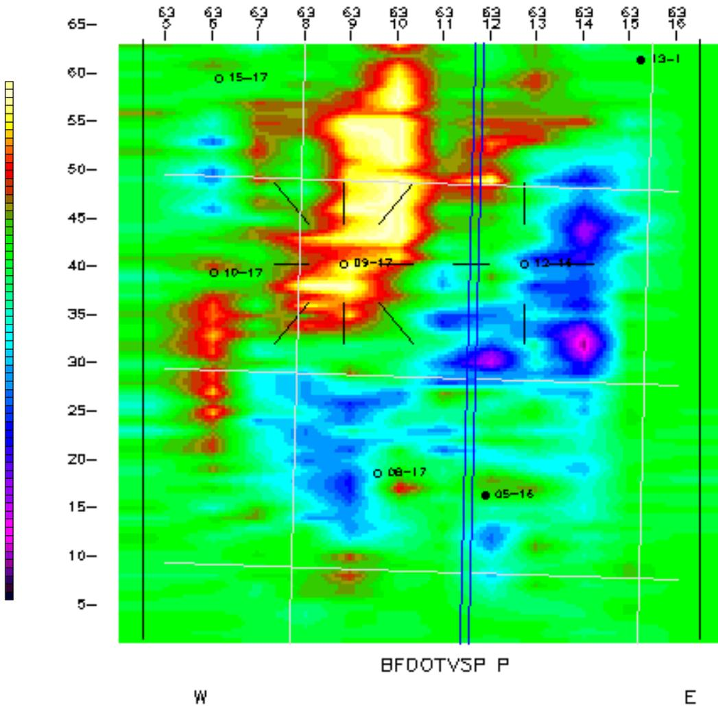
FIG. 10. 3-D VSP time slice at 1086 ms showing Mississippian structure.
