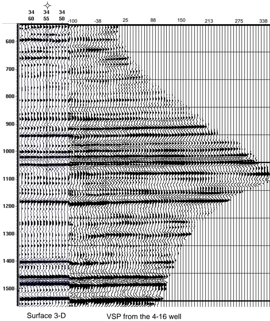
FIG. 7. P-P surface seismic and VSP sections near the 4-16 well.
