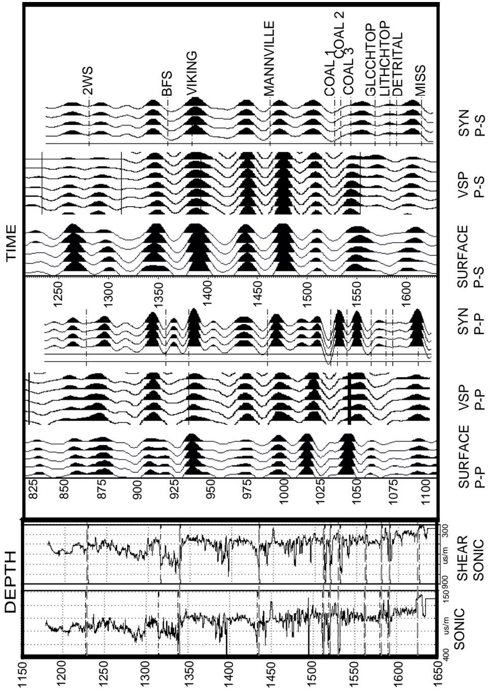
FIG. 4. Well logs, synthetic seismograms, and VSP traces for the 4-16-23-23W4 well
