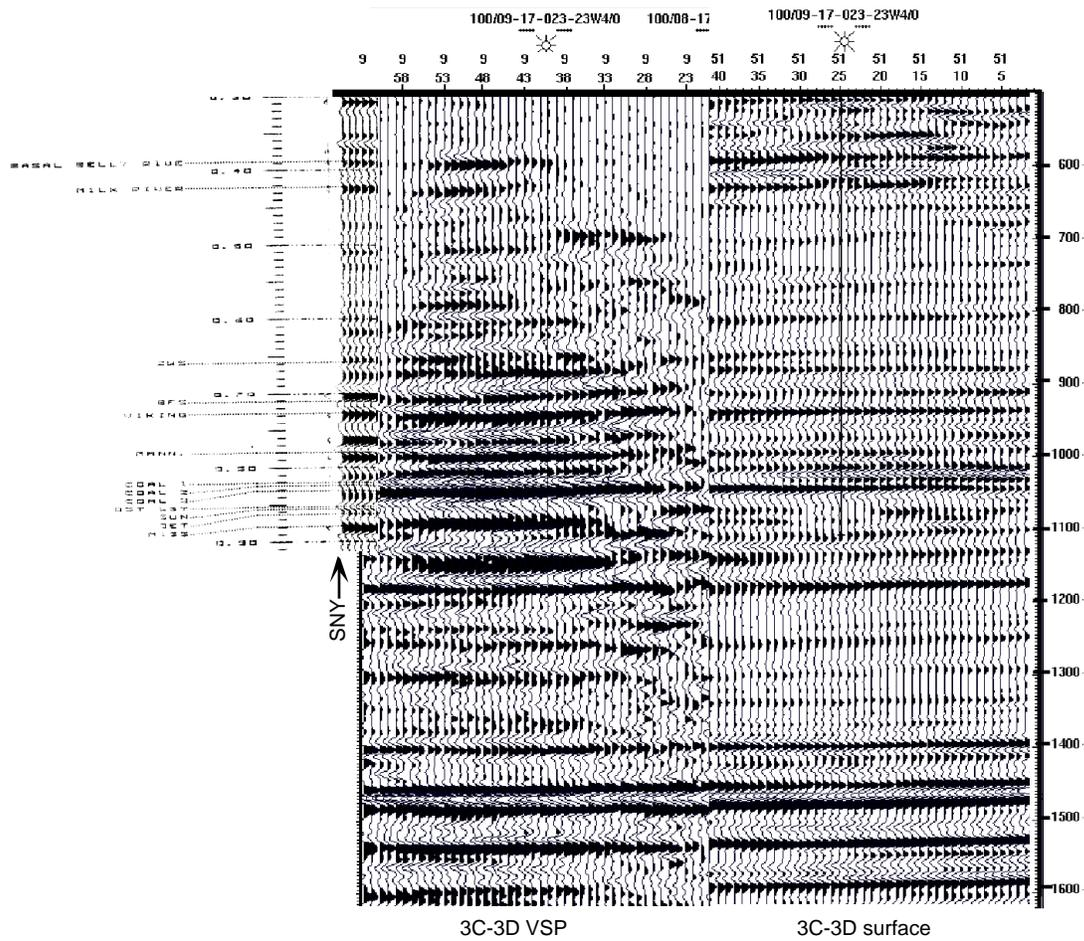
FIG. 9. 3-D VSP section for P-P waves correlated with the surface seismic section near the 12-16 well.
