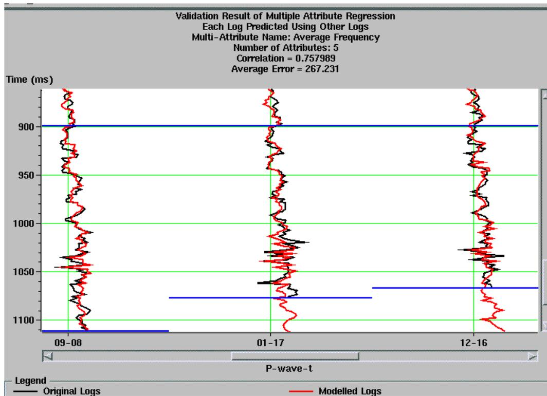
Figure 6: Measured logs (in black) and predicted logs (in red) using convolution operator.
