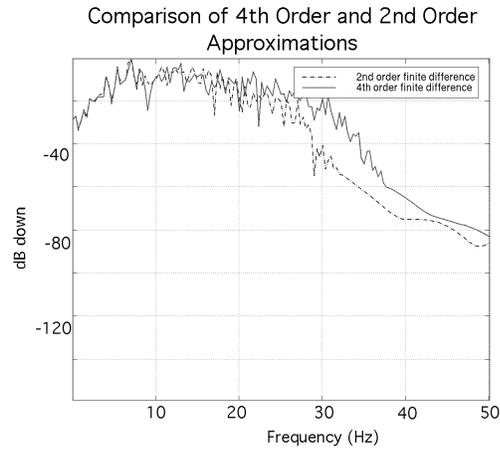
Fig. 8. A comparison of the dB spectrum of the second and fourth order approximations to the Laplacian operator. One can see that the fourth order approximation (solid line) has an increased bandwidth.
