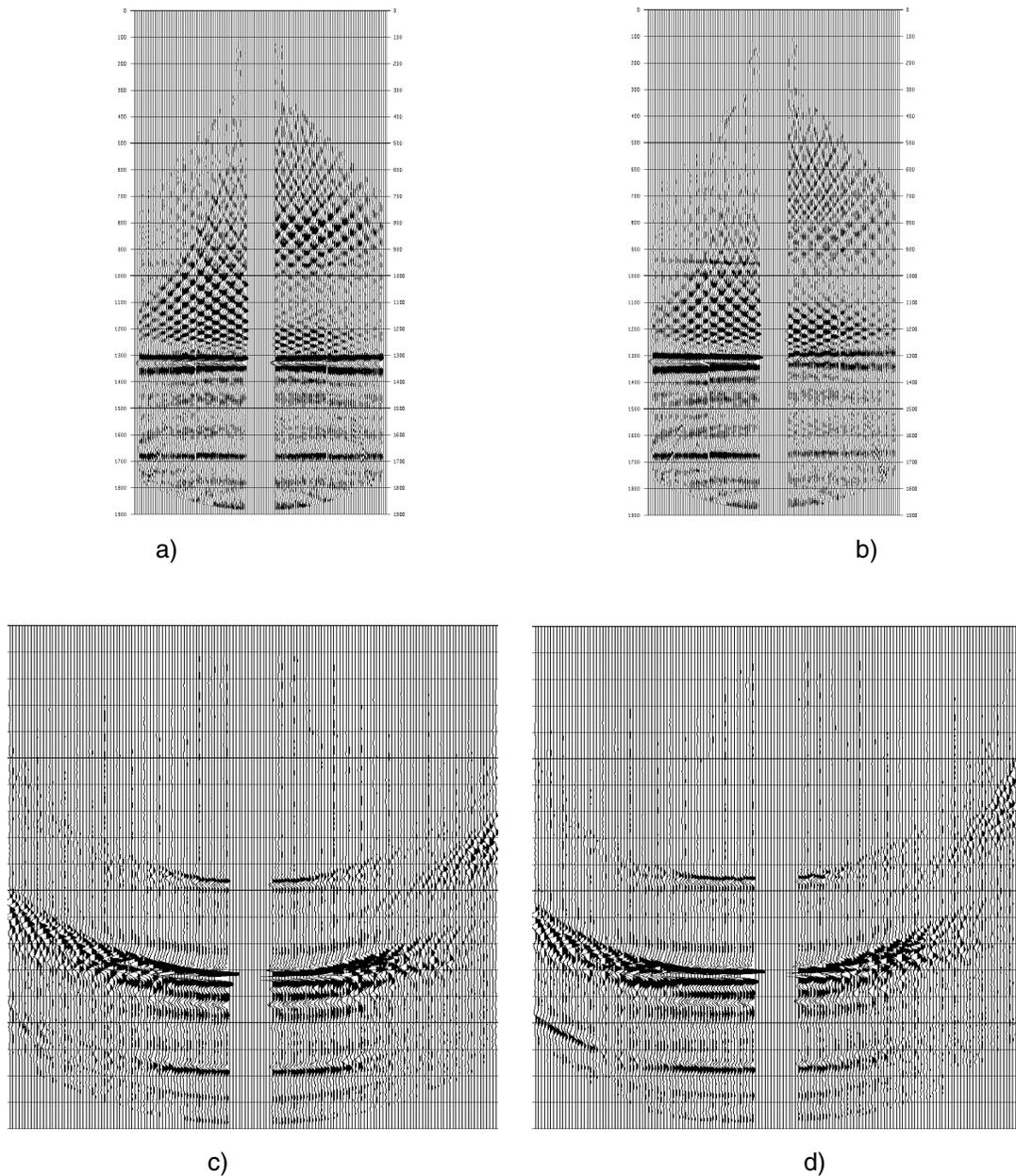
Figure 1. Comparison of CMP and CSP gathers that first ignore, then include anisotropic traveltimes computations, i.e.: a) isotropic CMP gather; b) anisotropic CMP gather; c) isotropic CSP gather; and d) anisotropic CSP gather.
