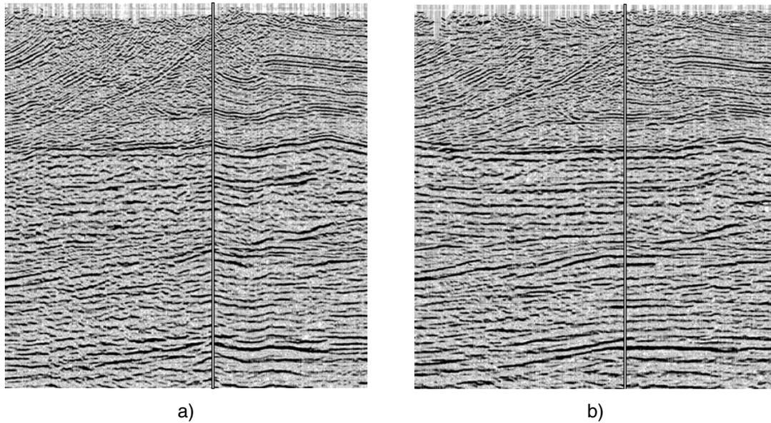
Figure 3. Conventional depth migrated sections with a) using isotropic velocities, and b) using anisotropic velocities. The vertical lines indicate the location of the CMP and CSP gathers in Figure 2.
