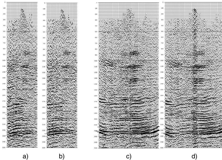
Figure 2. Foothills data example showing a) isotropic CMP gather, b) anisotropic CMP gather, c) isotropic CSP gather and d) anisotropic CSP gather.
