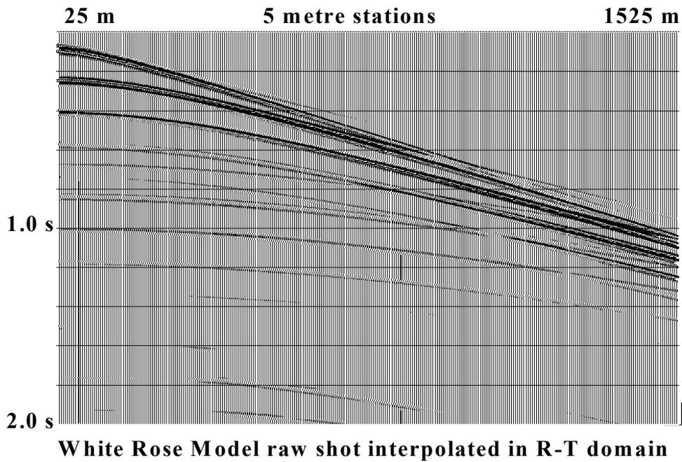
Figure 8. Synthetic shot gather after interpolation to finer station spacing in the radial trace transform. Spatial aliasing has been greatly reduced.
