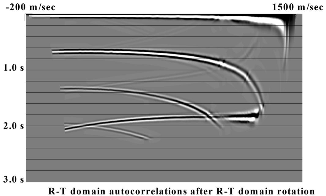
Figure 14. Autocorrelations of radial trace transform of the shot gather in Figure 12 (after radial trace domain rotation).
