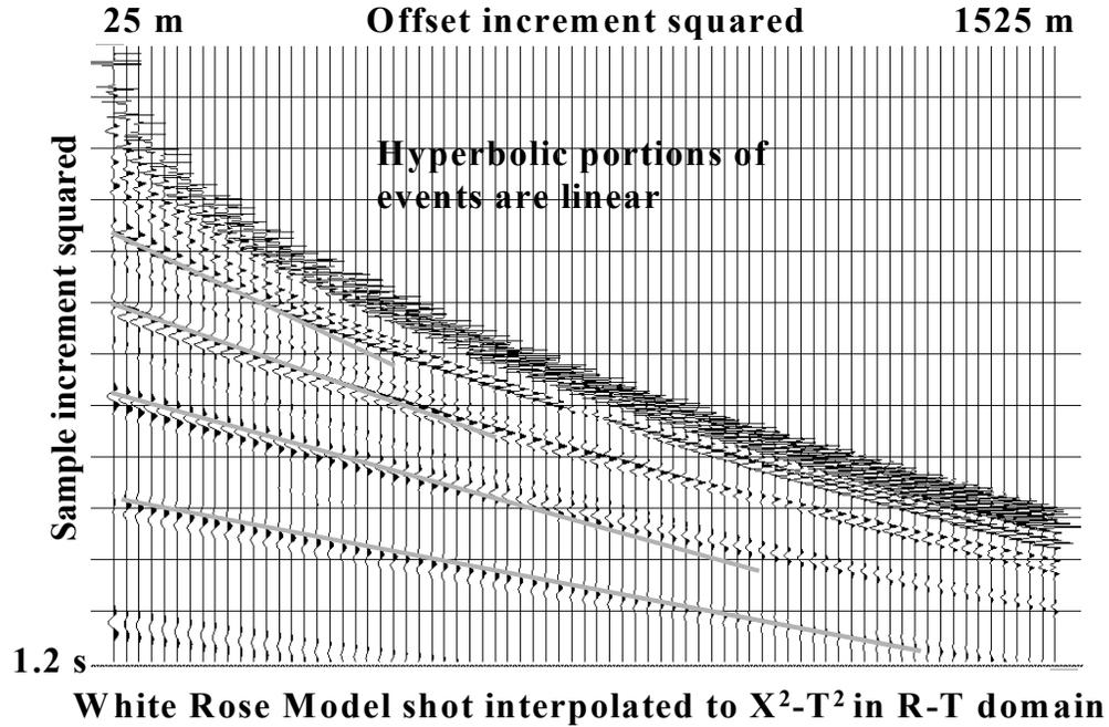
Figure 10. Synthetic shot gather interpolated to squared increments along both axes in the radial trace transform.
