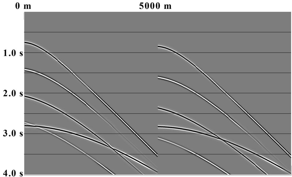
**Sea floor multiple model with 7.5 deg sea floor slope**
