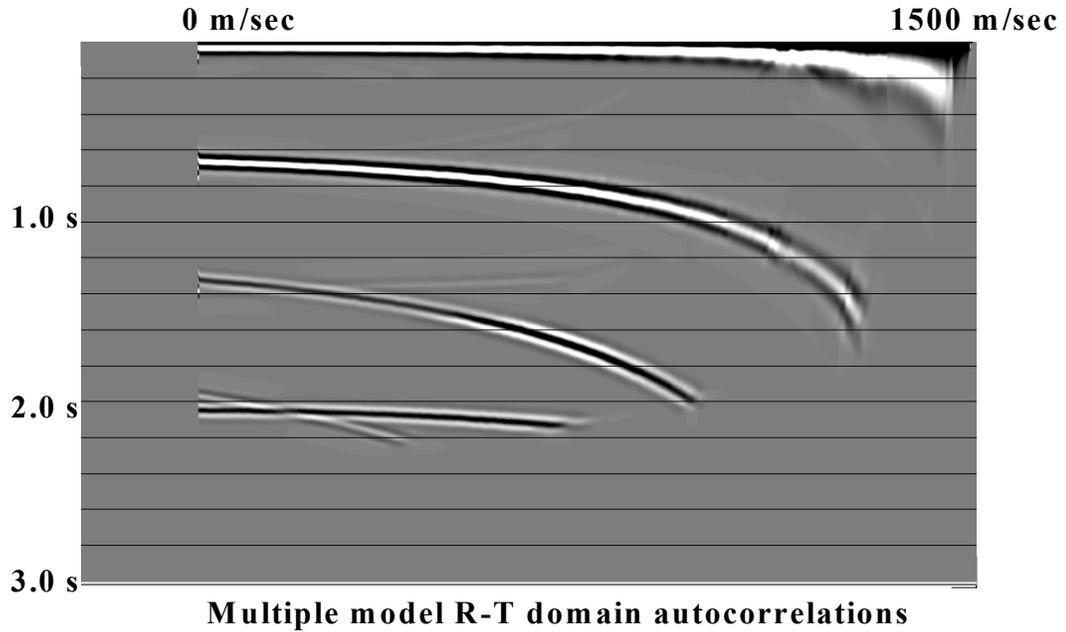
Figure 13. Autocorrelations of radial trace transform of the shot gather in Figure 11 (without radial trace domain rotation).
