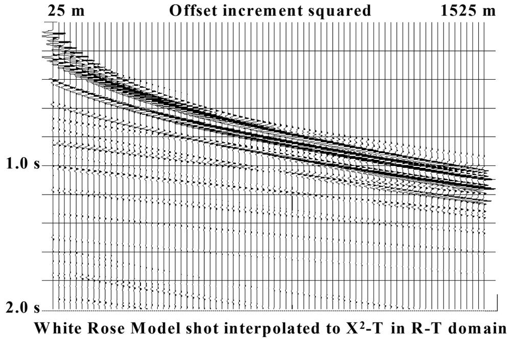
Figure 9. Synthetic shot gather interpolated to squared offset increment in the radial trace transform.
