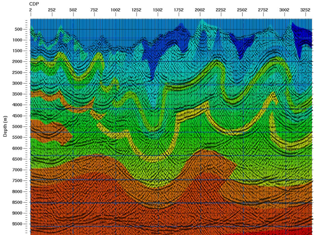
Figure 4. The post-stack depth migration image is super-imposed over the correct velocity model. This migration was performed with internal velocities calculated from picked stacking velocities.
