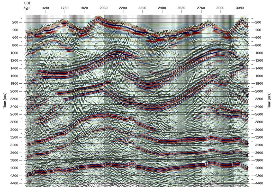
Figure. 9 The results from post-stack time migration (displayed in black wiggle) superimposed on the results from pre-stack depth migration from topography (displayed in color).
