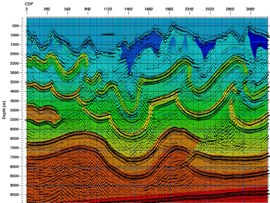
Figure 8. The image from pre-stack depth migration from topography is superimposed on the correct velocity model. The migration velocity was the correct model.
