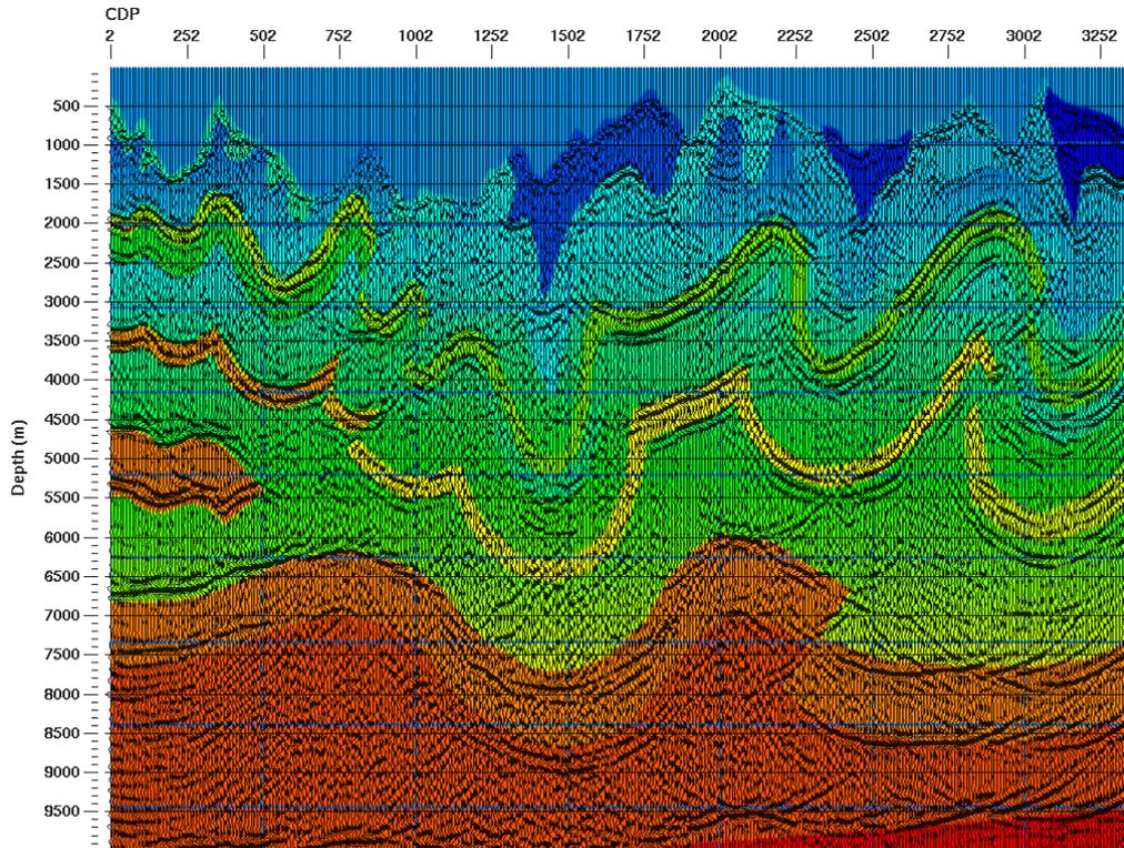
Figure 6. The post-stack time migration section, converted from time to depth. This section was migrated using internal velocities calculated from stacking velocities.
