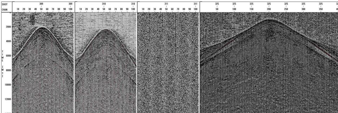
FIG. 6. Horizontal component (H2), receiver gathers for locations 3090, 3110, 3100 and 3250.
