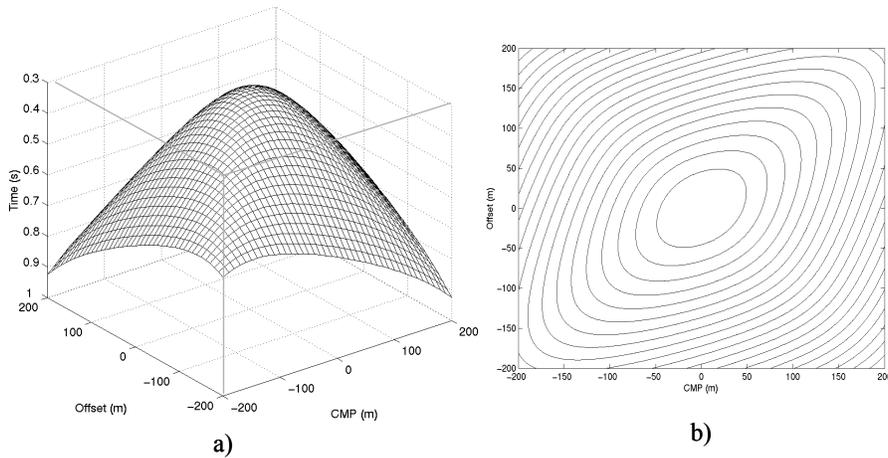
FIG. 2: a) Perspective view of a P-SV wave traveltimes surface for a scatterpoint located at  $z_0=100m$ .  $V_P=800m/s$  and  $V_S=400m/s$ ; b) plan view of (a) showing contour lines of constant traveltimes.
