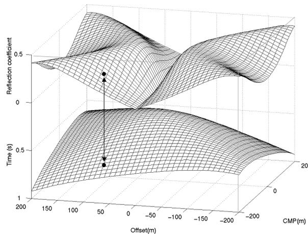
FIG. 4: A sample located on the traveltimes surface (bottom) is shown to be scaled by the corresponding reflection coefficient of the signal surface (top).
