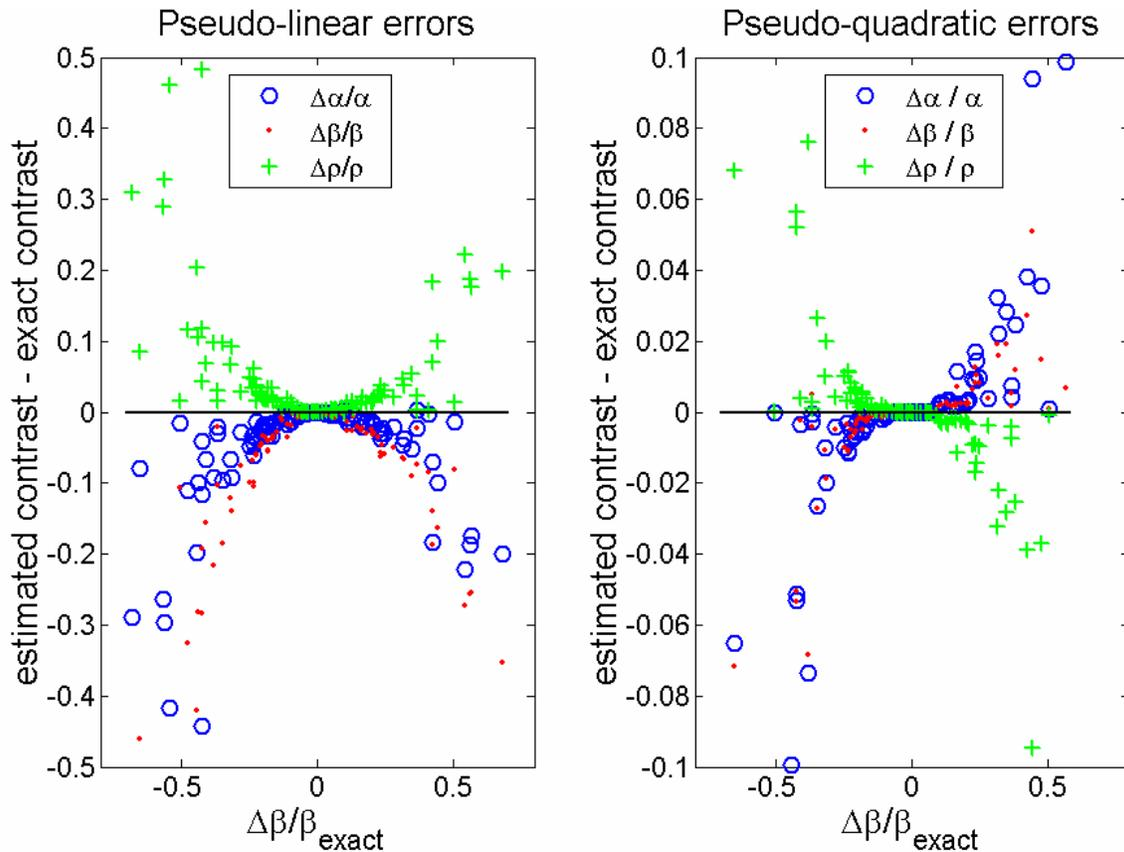
FIG. 3. Errors in the estimate of earth parameter contrasts for pseudo-linear and pseudo-quadratic methods. (The Aki-Richards predictions appear similar to those of the pseudo-linear method.) Note that the errors are strongly correlated with the value of  $\Delta\beta/\beta$ .
