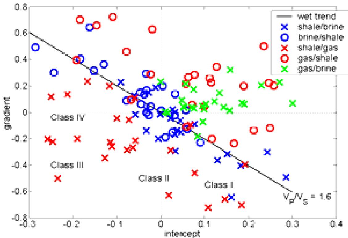
FIG. 1b. Crossplots of AVO gradient and intercept derived from earth-parameter ratios used in this study. Based on data from Table 1 of Castagna and Smith (1994).
