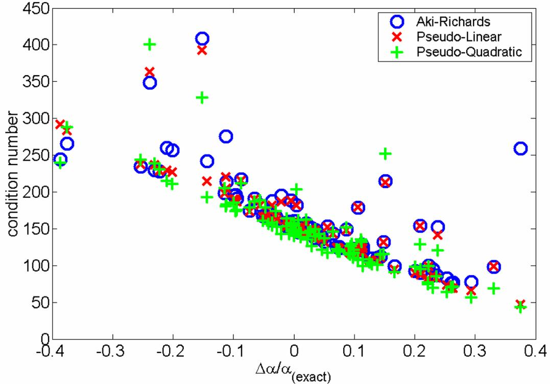
FIG. 2b. Plot of condition numbers and their variation with  $\Delta\alpha/\alpha$ . Note that this is unrelated to convergence, as the smallest condition numbers occur for large  $\Delta\alpha/\alpha$ .
