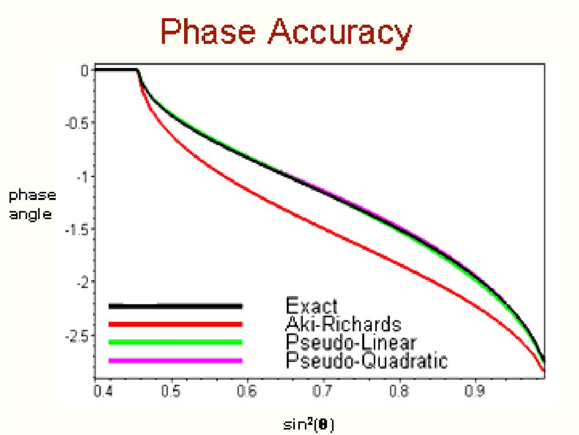
FIG. A-2. The phase angles (in units of pi) are plotted from just before the critical angle to nearly 90°. It is apparent that, while the Aki-Richards approach yields a reasonable approximation to the phase, the pseudo-linear and pseudo-quadratic methods provide a more quantitative representation.
