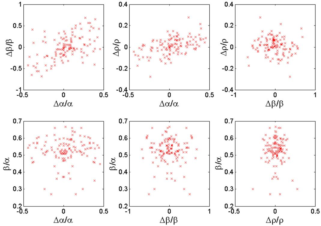
FIG. 1a. Crossplots of earth-parameter ratios used in this study. Based on data from Table 1 of Castagna and Smith (1994).
