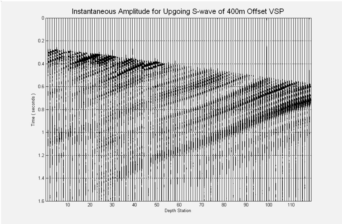
FIG. 5. Converted-wave instantaneous amplitude.
