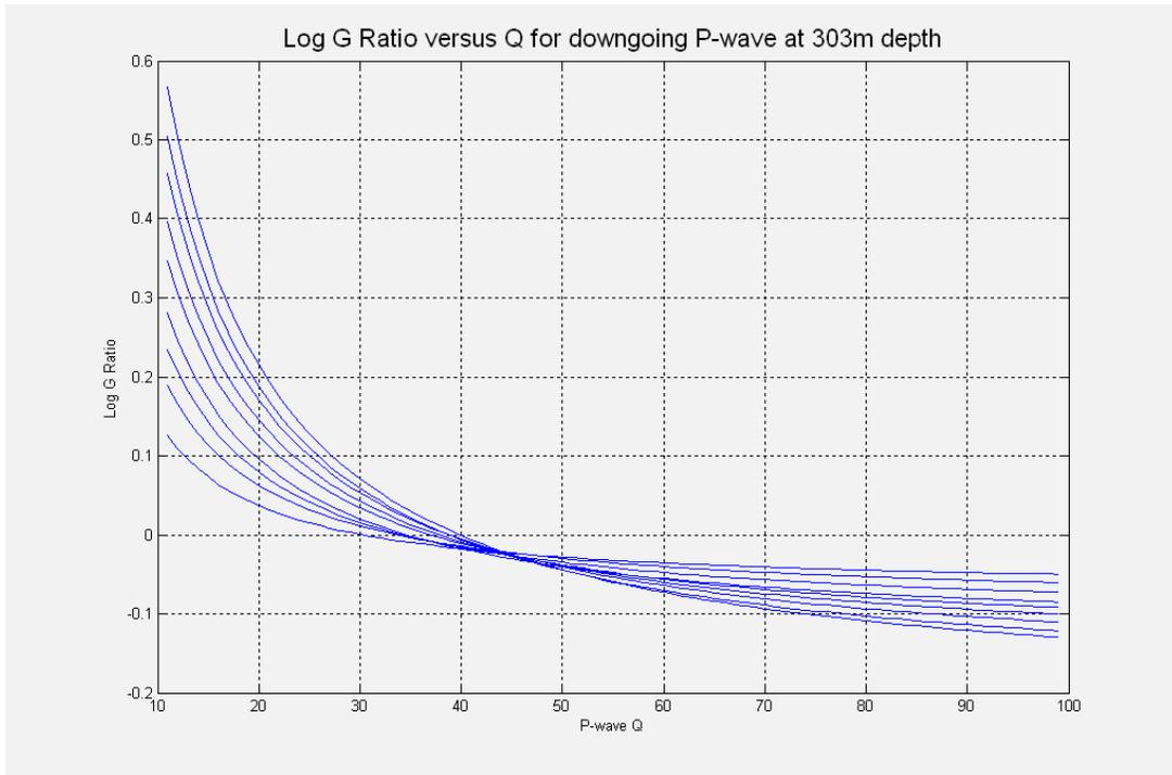
FIG. 3. Log spreading ratio versus Q for P-wave.
