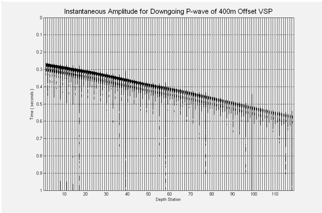
FIG. 2. Instantaneous amplitude of the Ross Lake VSP data shown in Figure 1.
