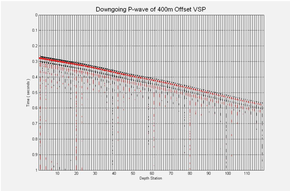
FIG. 1. Downgoing P-wave data from the Ross Lake offset VSP.
