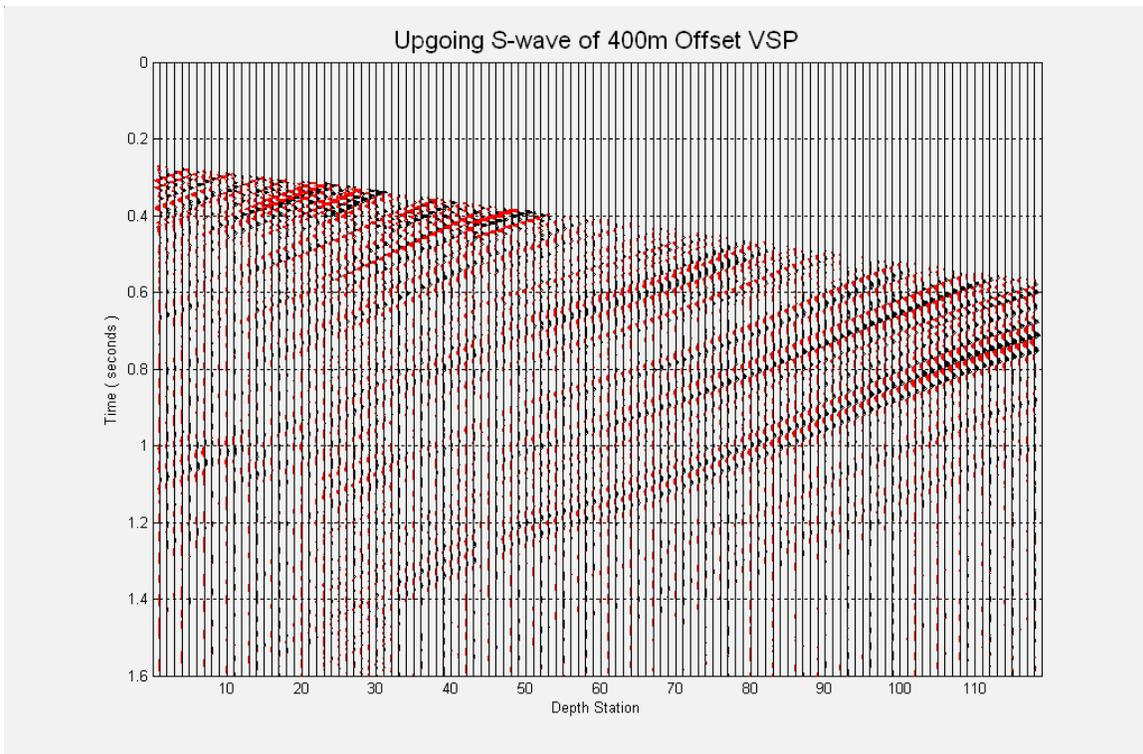
FIG. 4. Upgoing converted-waves.
