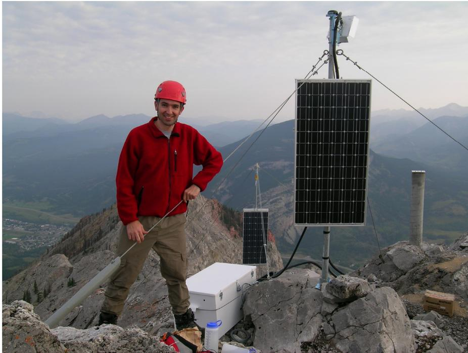
FIG. 3. H. Bland finishes checking the South Peak station. The solar panel in the background will power the subsurface geophone installation. The pillar on the right will be a prism reflector for electronic distance measurement.
