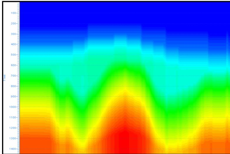
FIG. 13. RMS velocity model used for migration.
