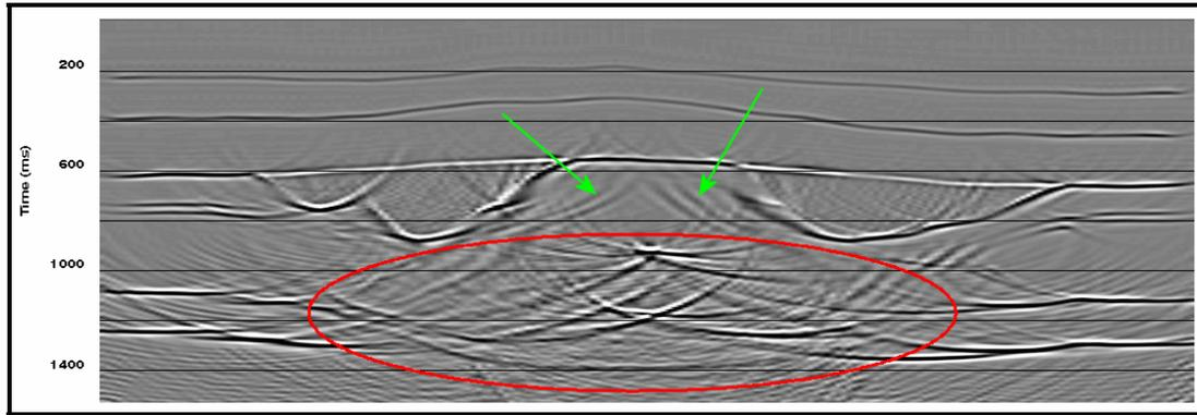
FIG. 11. Post-stack TIME migration. The algorithm has imaged successfully the upturned, steep layers, shallow reflectors and breccia deposits, but performed very poorly in the deep section.
