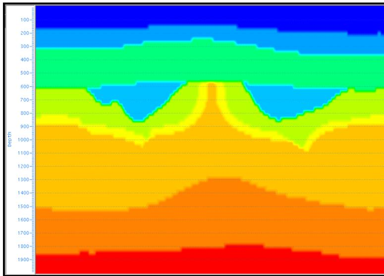
FIG. 5. Interval velocity model used to generate the synthetic seismic traces. The velocities are summarized in Table 2.
