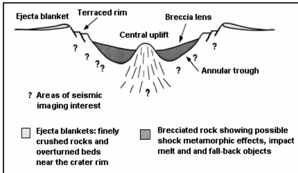
FIG. 1. Schematic of a complex crater (Westbroek and Stewart, 1995).
