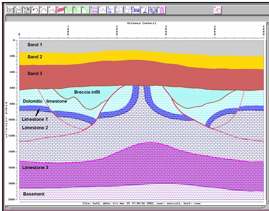
FIG. 3. Geologic model built in GX II. The velocity model is plotted in Figure 5 and summarized in Table 2.
