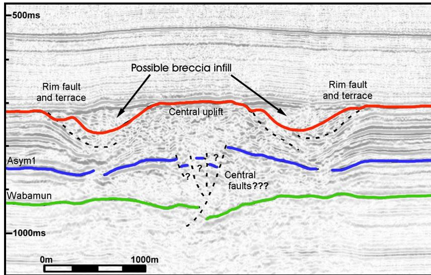
FIG. 2. Interpreted seismic section over the Hotchkiss structure of Alberta (Mazur et al., 2000).
