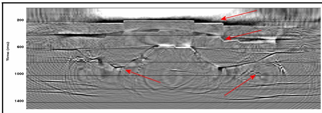
FIG. 12. Pre-stack TIME migration. Notice how the poorly smoothed, step-like character in the shallower RMS velocity transition (Figure 13) has affected the imaging and spread across the section (as indicated by the red arrows).
