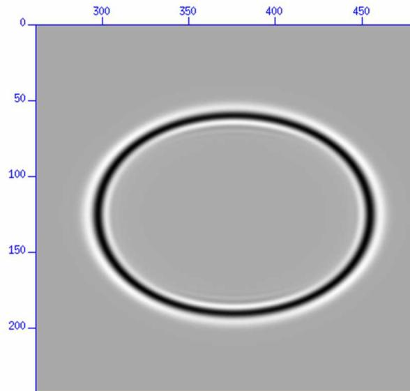
FIG. 2. Snapshot of the wavefront in medium with  $\epsilon = 0.2$  and  $\delta = 0.1$ .
