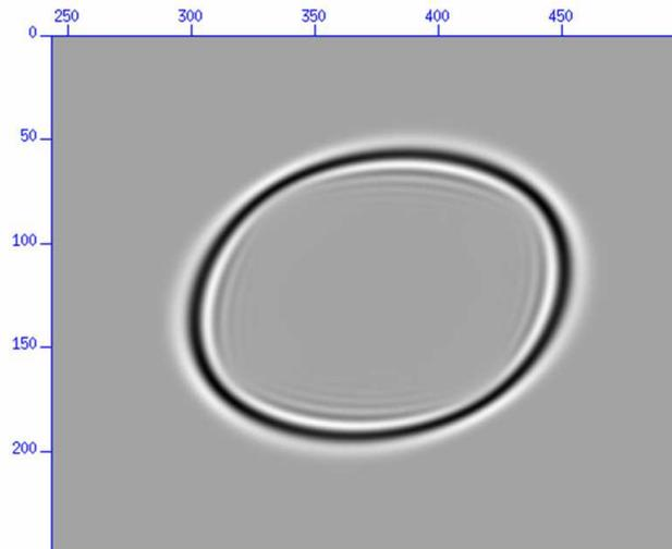
FIG. 5. Snapshot of the wavefront in medium with dip of  $30^\circ$ .
