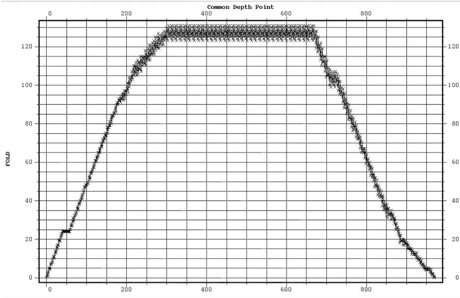
FIG. 6. CCP folds for  $V_p/V_s=2.2$  used for the horizontal components processing.
