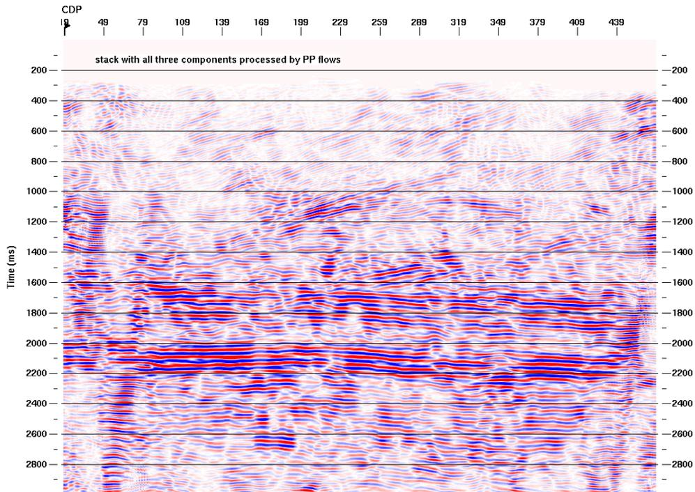
FIG. 13. Results of the vertical component, the radial component processed by the vertical component flow, and the transverse component processed by the vertical component flow are stacked to reduce the random noise.
