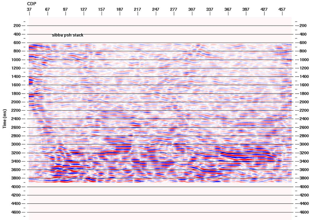
FIG. 8. The stacked section of the transverse component;  $V_p/V_s=2.2$ .
