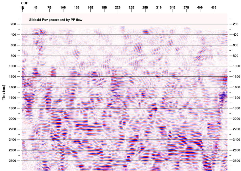
FIG. 12. The stacked section of the radial component processed with the vertical component processing flow shows only little similarity with the results from the vertical component.
