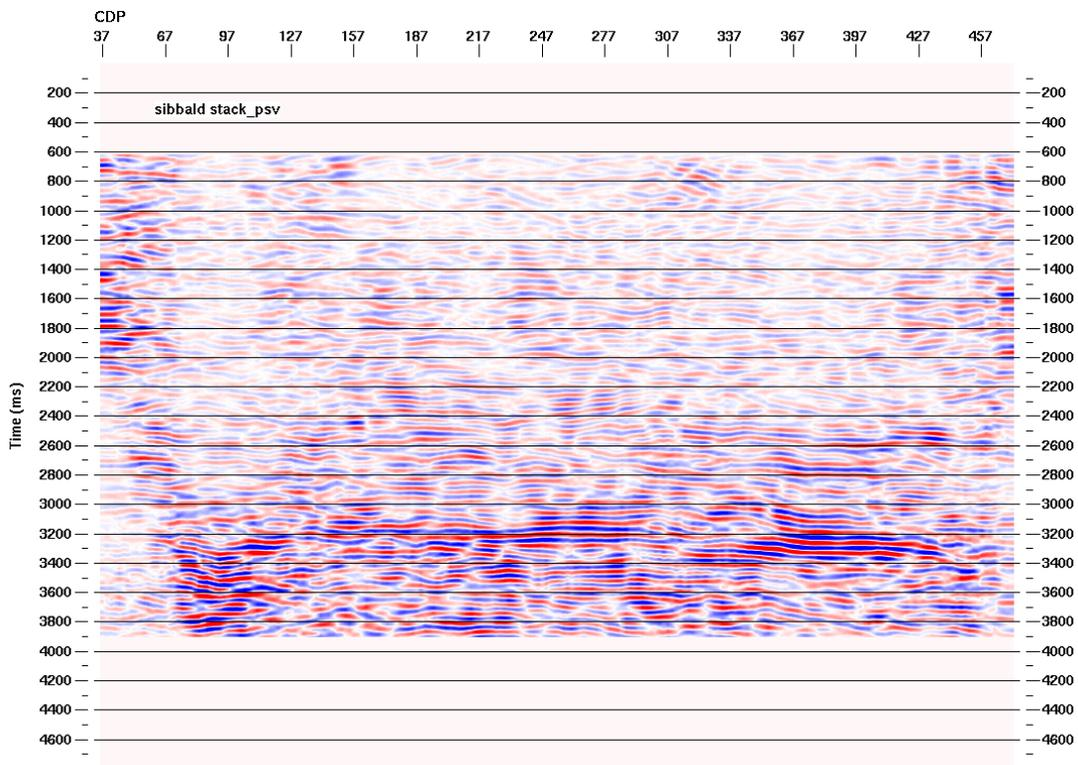
FIG. 7. The stacked section of the radial component for Vibrator sources;  $V_p/V_s=2.2$ .
