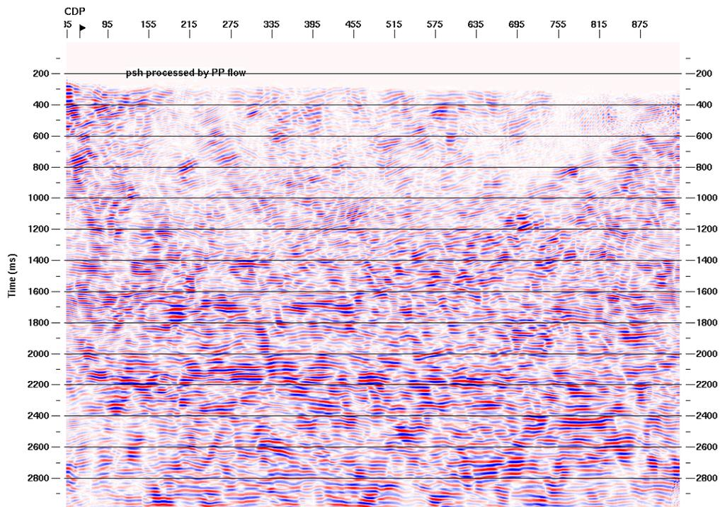
FIG. 17. The stacked section of the transverse component processed with the vertical component processing flow for the dynamite sources.
