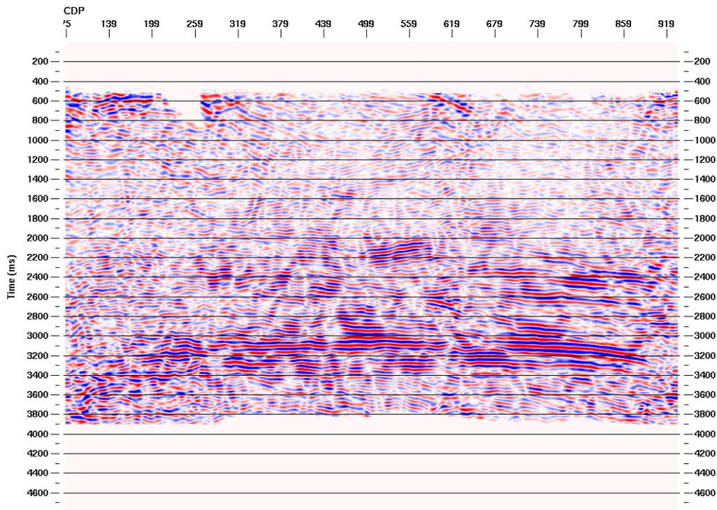
FIG. 15. Stacked section of the radial component (P-SV) from the dynamite sources.
