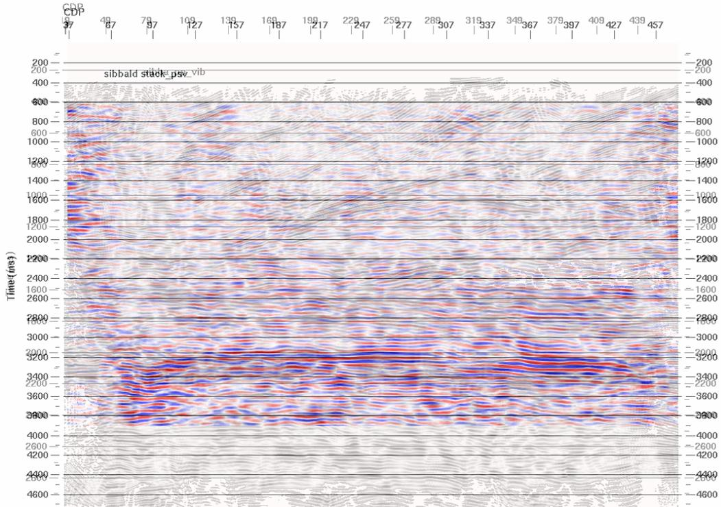
FIG. 9. The results from the vertical component and the radial component (after scaling stretching) are overlaid, the black lines are for the vertical component, the colour image is for the radial component.
