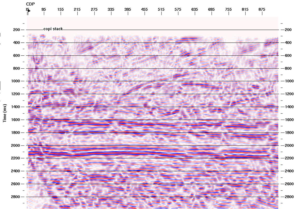
FIG. 14. Stacked section of the vertical component (P-P) from dynamite sources.
