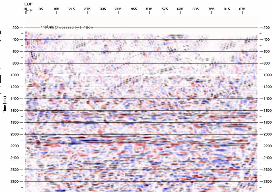
FIG. 18. The stacked section of the vertical component (in black) and the stacked section of the transverse component processed by the vertical component flow (in colour) from dynamite sources are overlaid.
