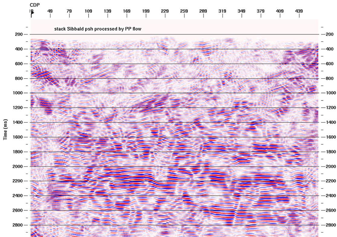
FIG. 10. The stacked section of the transverse component processed using the P-P processing flow. The strong P-P energy can be seen in this section.
