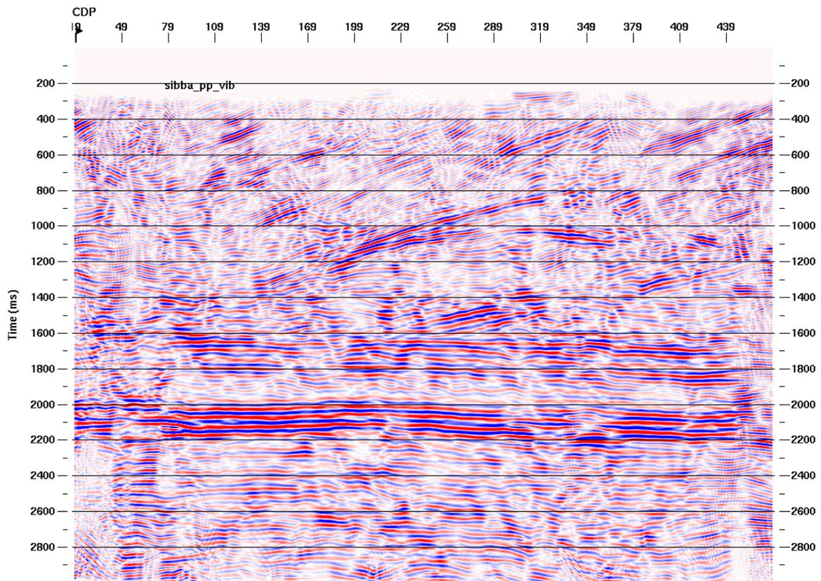
FIG. 5. The stacked section for Vibrator sources of the vertical component.
