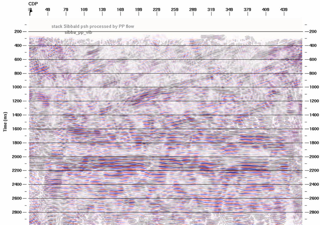
FIG. 11. Results from the P-P component are shown in black, and the results from the transverse component processed by the vertical component's flow are shown in colour.
