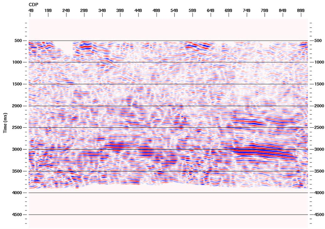
FIG. 16. Stacked section of the transverse component (P-SH) from the dynamite sources.
