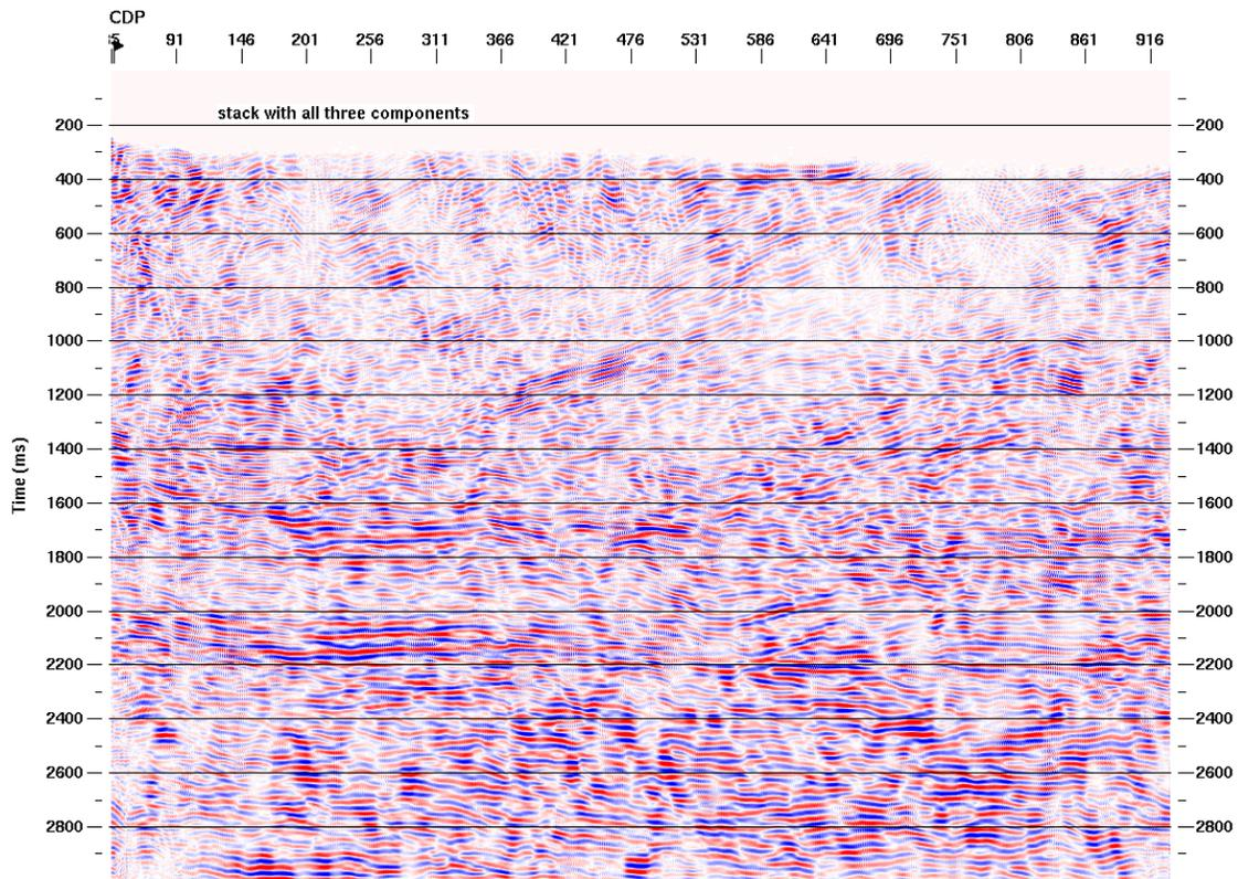
FIG. 19. The stacked section of the vertical component and the stacked section of the radial component and the transverse component processed by the vertical component flow from dynamite sources are stacked together into one section.
