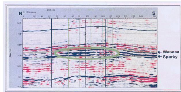
FIG. 19. Acoustic impedance difference section (from Watson et al., 2002).
