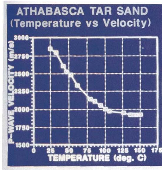
FIG. 10. Representative velocity-versus-temperature profile (from Matthews, 1992).
