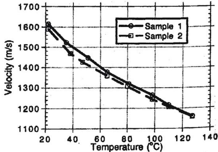
FIG. 9. Measured velocities in two Cold Lake bitumen samples (from Eastwood, 1993).
