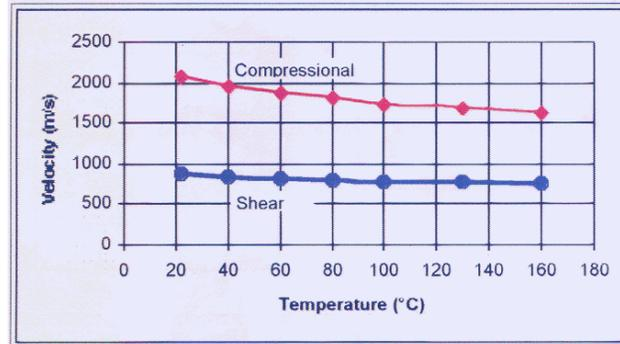
FIG. 22. Effect of temperature on  $V_p$  and  $V_s$  on a core sample from Pikes Peak (from Watson et al., 2002).
