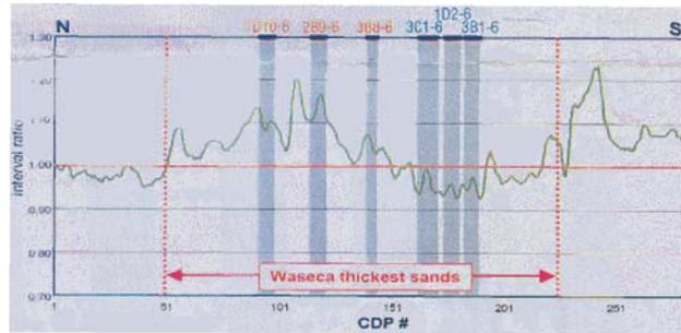
FIG. 13. H2000/H1991 ratio of Waseca interval traveltimes for P-wave arrivals (from Watson et al., 2002).
