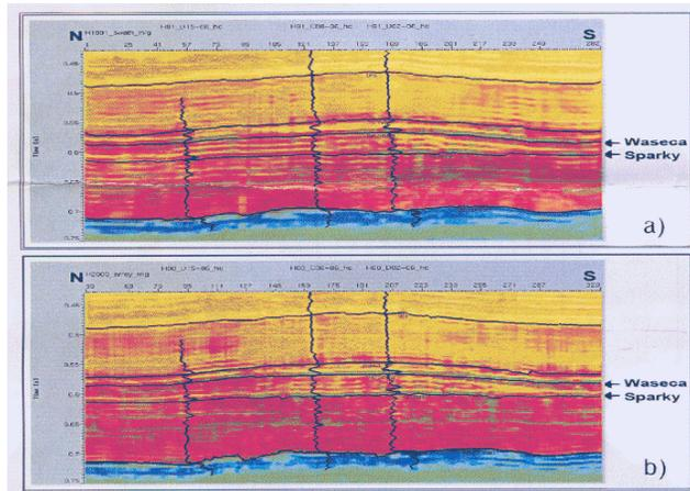
FIG. 17. (a) H1991 acoustic impedance section; and (b) H2000 acoustic impedance section (from Watson et al., 2002).
