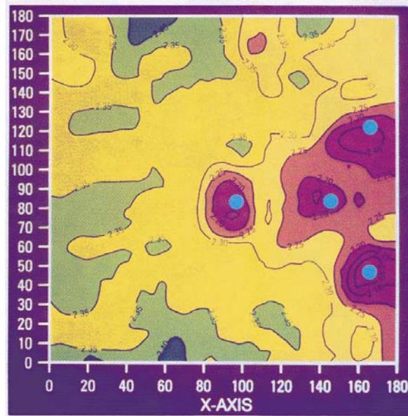
FIG. 12. Map of the tar-sands velocity model from monitoring survey 2 (from Lines et al., 1990).
