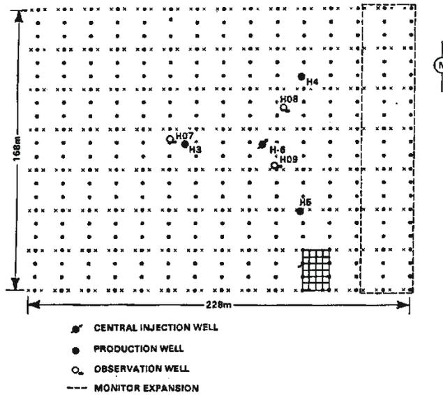
FIG. 2. Plan showing well configuration, source and receiver locations, and a portion of the stacking cell grid (from Matthews, 1992).
