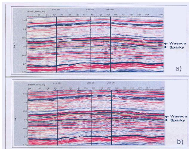
FIG. 16. (a) H1991 interpreted P-wave reflectivity section; and (b) H2000 reflectivity section (from Watson et al., 2002).
