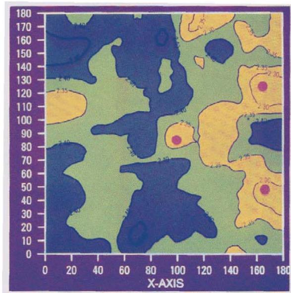
FIG. 11. Map of the tar-sands velocity model from monitoring survey 1 (from Lines et al., 1990).
