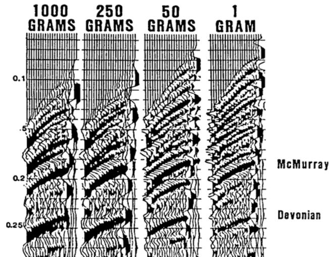
FIG. 7. Shot records (buried seismometers) for different charge sizes (from Pullin et al., 1987).
