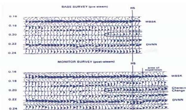
FIG. 14. Seismic amplitude change associated with pre- and post-steam surveys (from Matthews, 1992).
