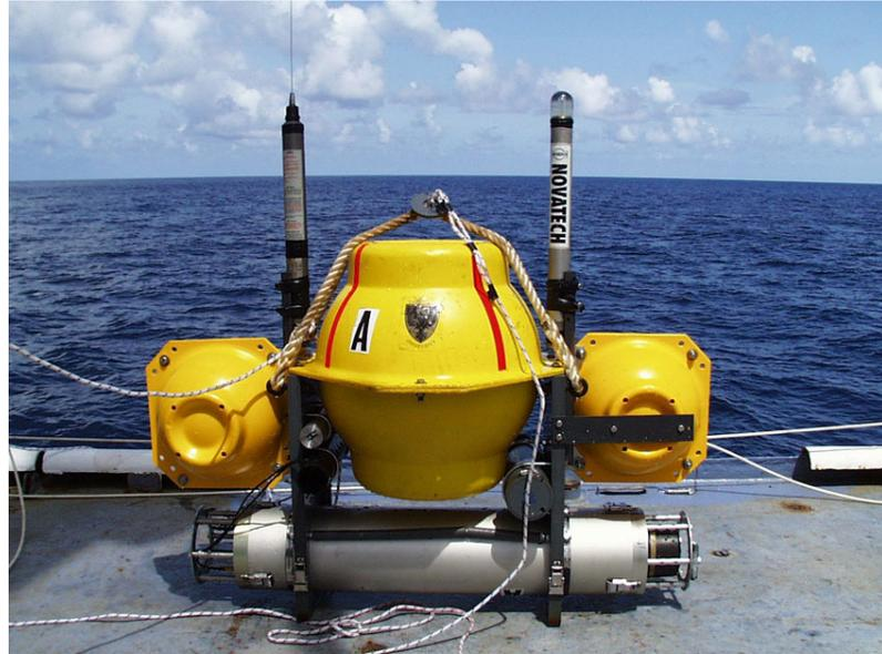
FIG. 11: Dalhousie ocean-bottom seismometer (OBS). (Modified from [www.dal.ca](http://www.dal.ca), 2002)
