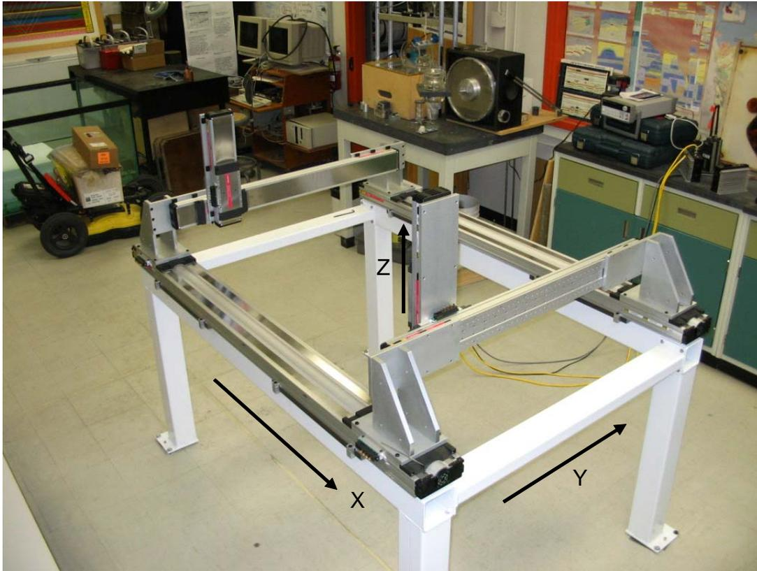
FIG. 2. Physical modelling system. The system measures 1.4m along the X axis, 1.1 m along the Y axis. Models can stand up to 1 m tall within the centre of the system.
