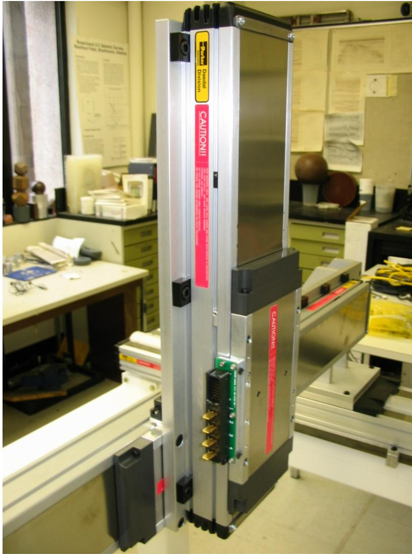
FIG. 3. Close-up of the Z axis linear motor. The four pin electrical connector in the picture is mounted to the side of the Z axis forcer. The forcer is in the down position. The transducer assembly (not attached) connects to the flat face of the forcer.
