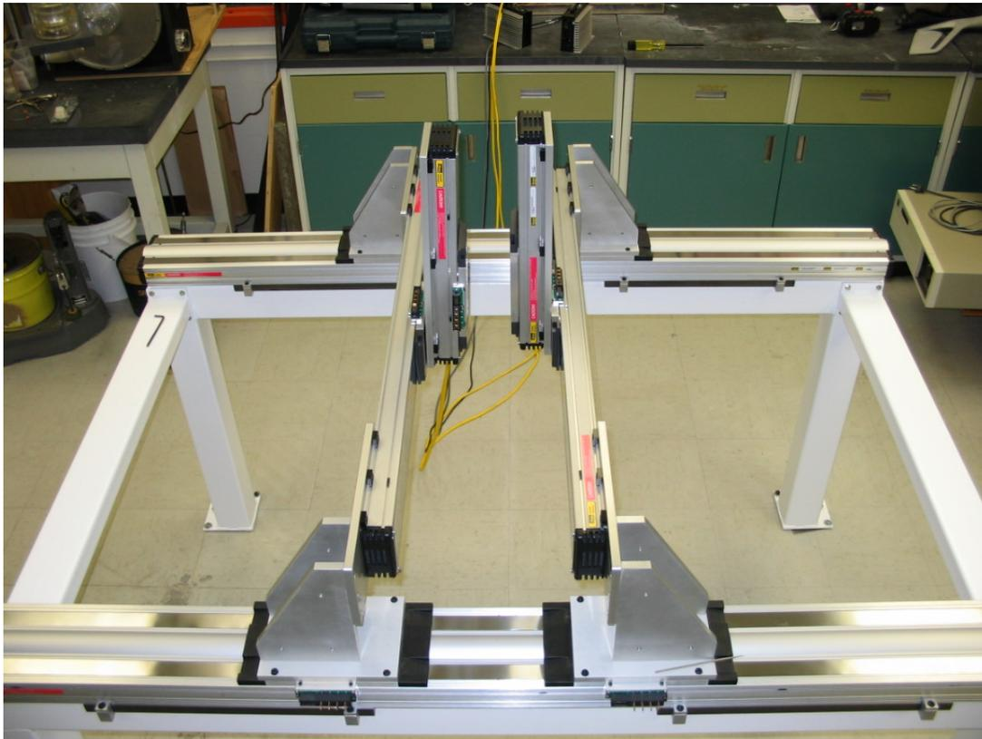
FIG. 2. Z axes forcings are shown face to face in the center of the acquisition area. The photograph, taken during assembly, does not show the transducer mount, cables, or cable management system.
