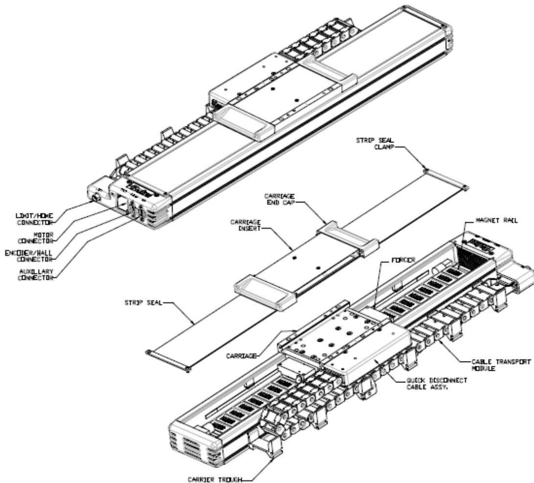
FIG. 1. Components of a linear motor (Parker Automation 400LXR series linear motor) are shown assembled (top) and disassembled (bottom). Source: 400LXR users manual, Parker Automation.
