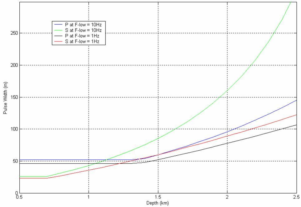
FIG. 3. -40dB noise floor  $\sin(x)/x$  resolution as function of depth ( $Q_P = 80$ ,  $Q_S = 40$ ,  $F_{max} = 80\text{Hz}$ ).
