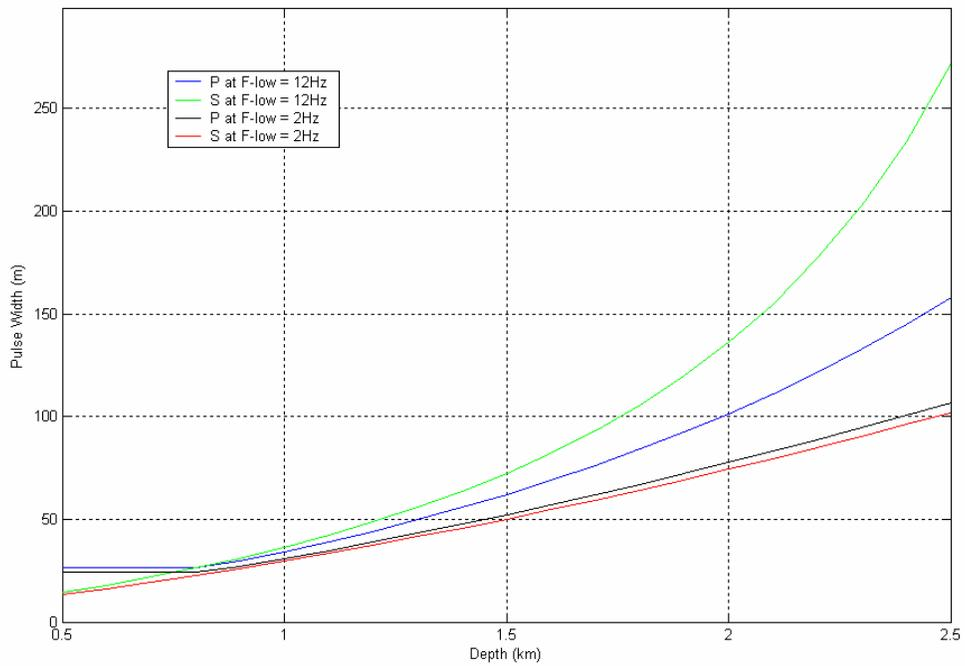
FIG. 4. -40dB noise floor  $\sin(x)/x$  resolution as function of depth ( $Q_P = 80$ ,  $Q_S = 50$ ,  $F_{max} = 150\text{Hz}$ ).
